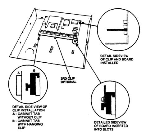
Before mounting the circuit board be certain that the appropriate metal knockouts have been removed. DO NOT ATTEMPT TO REMOVE THE KNOCKOUTS AFTER THE CIRCUIT BOARD HAS BEEN INSTALLED.
