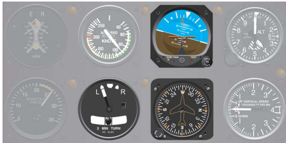
Figure 6-4. The flight instruments used for bank control are the attitude, heading, and turn indicators.
