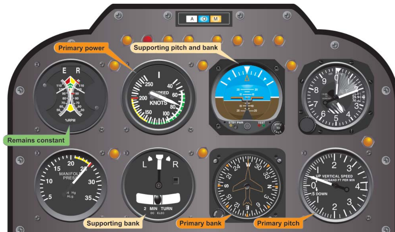
Figure 6-13. Flight Instrument Indications in a Stabilized Constant-Rate Climb.
