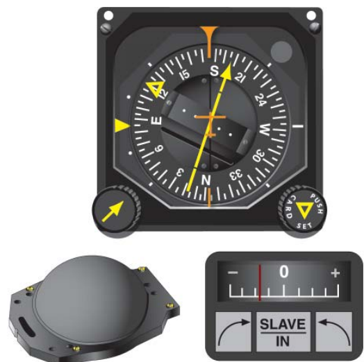
Figure 3-25. Pictorial Navigation Indicator (HSI Top), Slaving Control and Compensator Unit.
