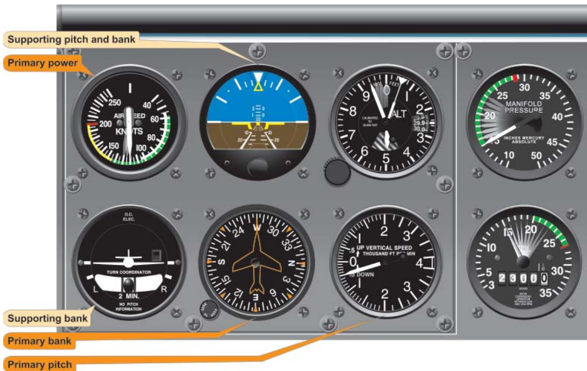
Figure 5-30. Constant Airspeed Descent, Airspeed High—Reduce Power.
