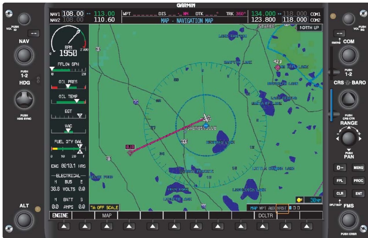
Figure 11-13. The MFD is another means of viewing the nearest airports.
