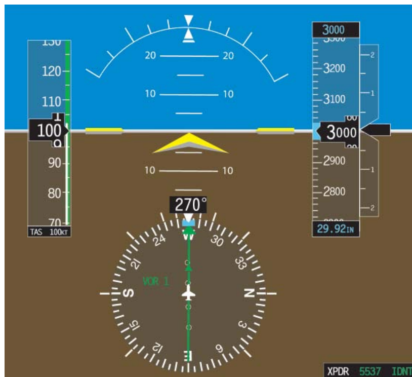
Figure 6-17. PFD Indications During Straight-and-Level Flight.
