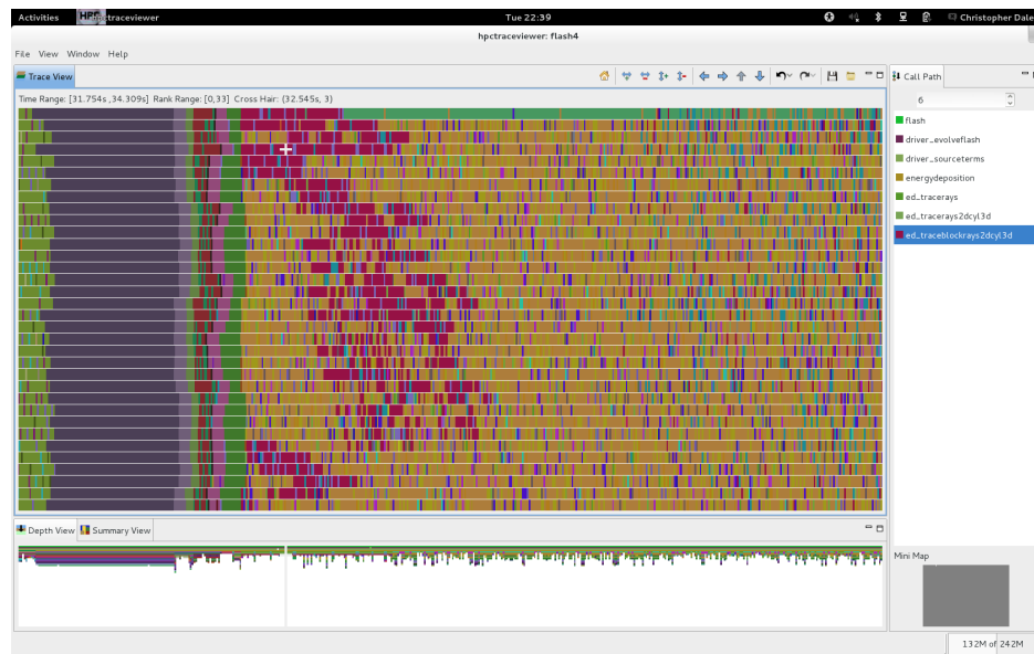
Figure 17.13: Performance trace of MPI ranks 0-33 in a laser simulation using asynchronous communication and run with 2048 MPI ranks on Intrepid BG/P.
