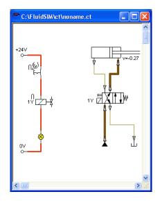
Electrically or hydraulically operated valves can only be switched manually, when there is no control signal applied.
