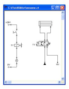
So that the valve can be controlled by the solenoid, you have to link the components with a label.
