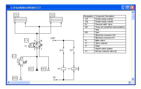
The parts list component analyzes all components of the diagram and generates table with columns for the component identifications and the component designations. In this connection, FluidSIM uses existing labels and texts as component identifications.
