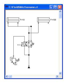
The following circuit diagram contains mistakes of type 2, 3, 4, and 6:
