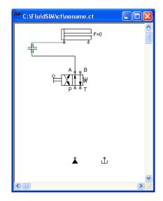
In the Edit Mode the components and lines can be selected, moved, or deleted by clicking on *Edit Delete* or by pressing the *Del* key.
