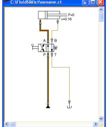
After the cylinder has been extended, the pressure in the cylinder supply line must inevitably increase. This situation is recognized by FluidSIM and the parameters are recalculated; the pressure downstream of the pump unit increases to the value, as defined by the pump unit safety guard.
