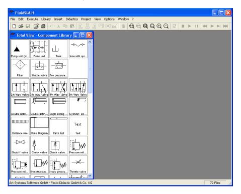
The left-hand side shows the component library of FluidSIM in its total view; it contains hydraulic and electrical components for the creation of new circuit diagrams. The menu bar at the top of the window lists all the functions needed for the simulation and creation of circuit diagrams. The toolbar beneath this menu displays frequently used menu functions.
