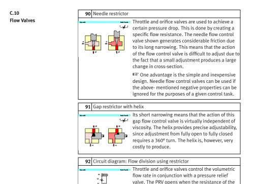
flow control valve becomes greater than that of the opening pressure set on the PRV. This produces a
