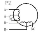
6-wire motor high torque mode
