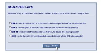
Select the radio button beside the RAID level you want for your logical drive. WebPAM displays the RAID levels you can use with the available disk drives. You can also select JBOD on this screen.
