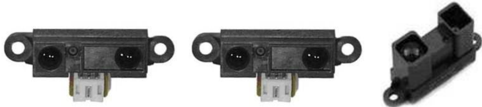
GP2D120 GP2D12 GP2Y0A02YK Figure 3.32: Sharp IR Range sensors for Fire Bird V
