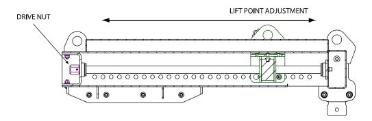
Turning the drive nut on the end of the shaft the lift point moves along the rear spine, tilting the load by varying the motor connection point relative to the centre of mass of the cluster. The screw is located in polymer sealed bearings requiring no maintenance under normal operating conditions, and is designed to last the lifetime of the product.
