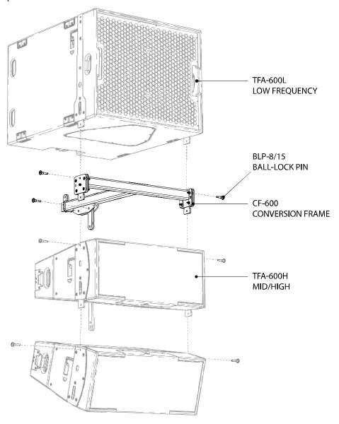
Connection to the first TFA-600H cabinet is made via two 10mm ball-lock pins which are engaged into the rear spine of the mid/high cabinet (one pin is located on the loudspeaker and one pin is located on the conversion frame).
