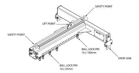
The movable lift point can be traversed along the spine by means of a screw which is turned by a 22mm (7/8") socket (available from Turbosound) fitted to a speed brace or electric drill.
