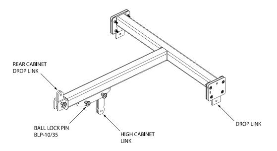
The CF-600 conversion frame also functions as a ground stacking frame, interfacing between ground stacked TFA-600L bass cabinets and the mid-high cabinets positioned on top.
