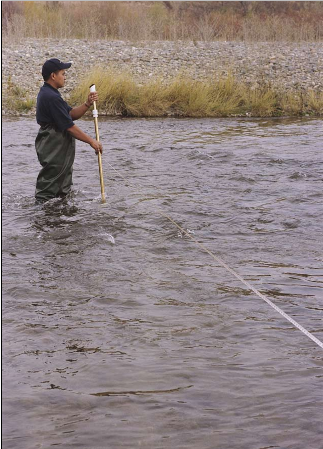
Measuring streamflow with Global Water's Flow Probe.
