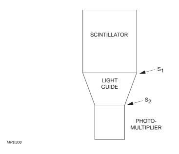
Fig.6.5 Truncated cone light guide
