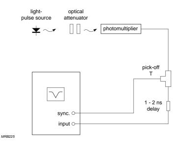
Fig.4.6 Set-up for measuring pulse response
