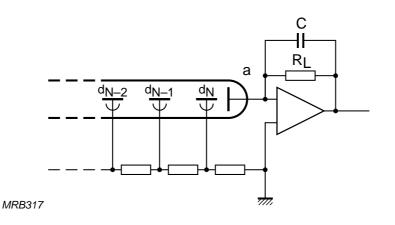
Fig.6.14 Circuit for a photomultiplier in continuous mode
