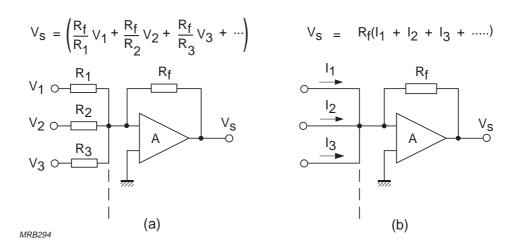
Fig.5.32 (a) Voltage adder, (b) current adder
