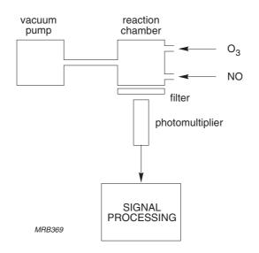
Fig.8.2 Measurement of chemiluminescence
