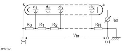
Fig.2.12 Dark-current measurement; the tube is connected in negative polarity with (+) supply terminal grounded.
