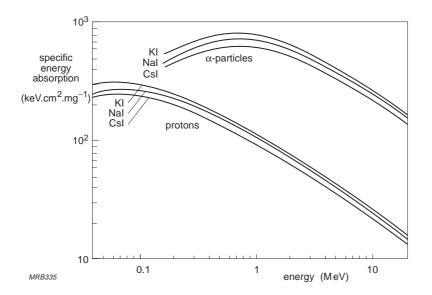
Fig.A6.7 Specific energy absorption for ionizing  $\alpha$ -particles and protons in pure KI, Nal and CsI scintillators
