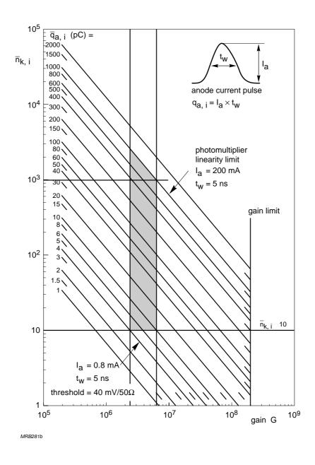
Fig.5.19 Photomultiplier working diagram in terms of photoelectrons per pulse, n<sub>k i</sub>, gain, and mean anode charge per pulse
