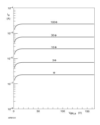
Fig.1.13 Anode current as a function of last-dynode-to-anode voltage, with relative incident flux  $\phi$  as parameter
