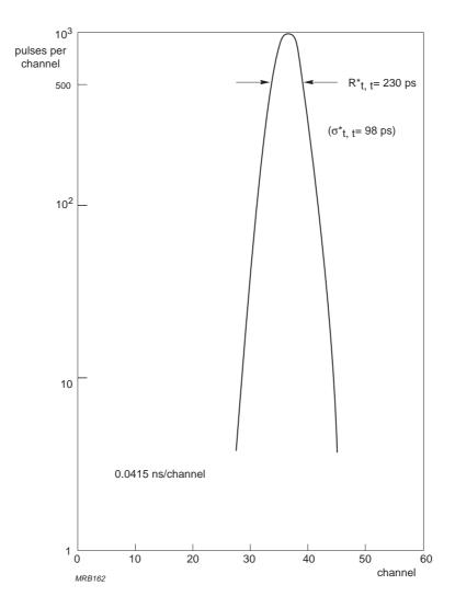
Fig.6.27 Coincidence time resolution distribution from two fast scintillation counters for  $^{60}$ Co coincidence  $\gamma$ - $\gamma$  radiation
