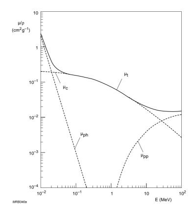
Fig.A6.11 Mass absorption coefficient for X- and  $\gamma$ -radiation in an organic anthracene C<sub>14</sub>H<sub>10</sub> scintillator
