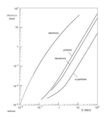
Fig.A6.12 Calculated pathlength of four types of charged particle in an organic scintillator (*Nuclear Enterprises Ltd.*)
