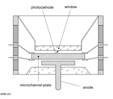
Fig.1.14 Section through a microchannel-plate photomultiplier
