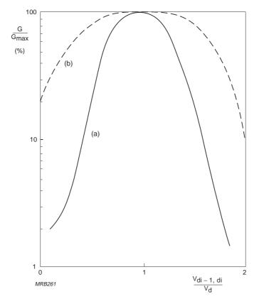
Fig.4.10 Gain variation as a function of the voltage between successive dynodes, for a tube with (a) linear focusing dynodes, (b) venetian-blind dynodes. V<sub>d</sub> = nominal interdynode voltage
