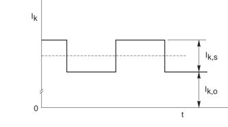
Fig.3.10 Cathode current when the input flux is chopped
