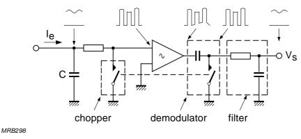
Fig.5.36 Chopper-stabilized amplifier
