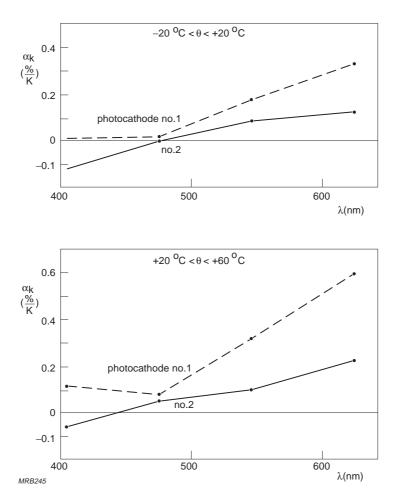
Fig.4.30 Examples of the variation of the temperature sensitivity coefficient  $\alpha_k$  of SbKCs bialkali cathodes as a function of wavelength
