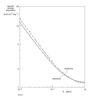
Fig.A6.6 Specific energy absorption for electrons and positrons in pure Nal as a function of their energy (U.S. National of Bureau Standards, circular number 577, 1956)
