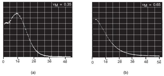
Fig.3.8 Single-electron spectra of photomultipliers with CuBe dynodes a) linear-focusing, b) venetianblind. Vertical axes, pulse frequency (arbitrary scale; horizontal axes, anode pulse amplitude referred to number of electrons per pulse at the cathode
