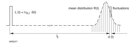
Fig.A4.6 Transit-time distribution of n<sub>k,i</sub> elementary response pulses
