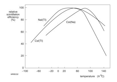
Fig.A6.10 Scintillation efficiency as a function of temperature for several inorganic scintillators (Harshaw Chemical Company)
