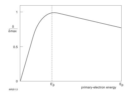
Fig.A1.10 Relative variation of secondary-emission coefficient  $\delta$  as a function of primary-electron energy  $E_p$ . For energies above  $E'_p$ ,  $\delta$  falls off proportional to  $E_p^{1-\alpha}$
