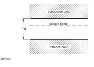
Fig.A6.1 Energy band diagram in an inorganic crystal
