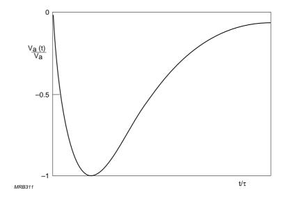
Fig.6.8 Voltage pulse shape over the anode load  $\rm R_L C$
