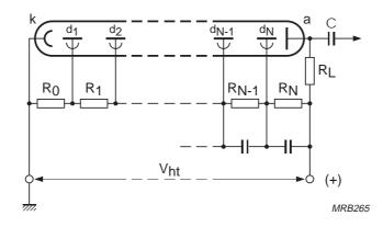
Fig.5.1 Positive-polarity voltage supply
