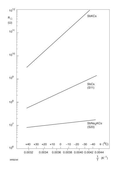
Fig.4.33 Surface resistivities of three photoemissive materials as functions of temperature
