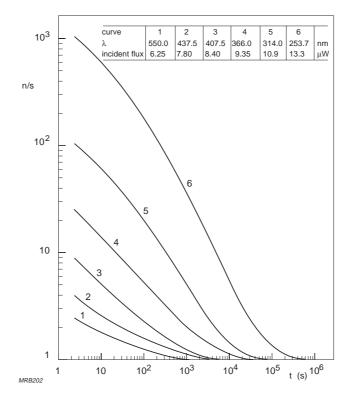
Fig.3.5 Dark-current decay of an S13 cathode at 0 °C following exposure for 100 s to equal numbers of photons, with wavelength as parameter ( $\phi \propto 1/\lambda$ ). Vertical scale, relative number of electrons per second
