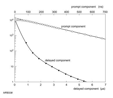
Fig.A6.9 Decay time components of a Nal(TI) scintillator for γ-radiation (*Rev. Sci. Instr.* 32 (1952) 1044)
