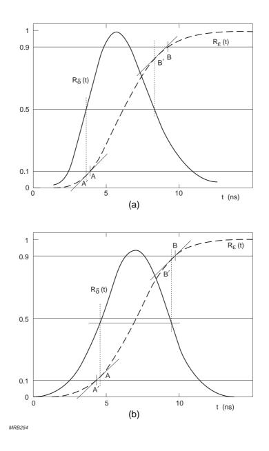
Fig.A4.3 Pulse response (a) of the type at<sup>m</sup>exp (-bt); (b) Gaussian pulse response
