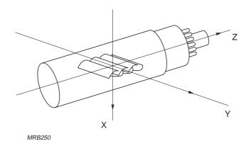
Fig.4.35 Axes used in measuring magnetic sensitivity
