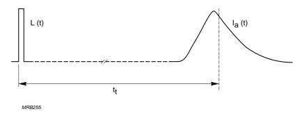
Fig.A4.4 Pulse transit time t<sub>t</sub>.
