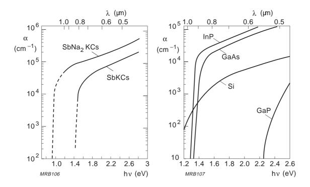
Fig.A1.5 Absorption coefficients  $\alpha$  as functions of photon energy hv for various photoemissive layers
