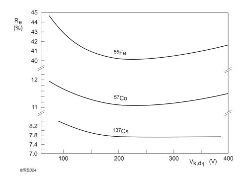
Fig.6.23 Energy resolution variation as a function of cathode to first-dynode voltage. Sources <sup>55</sup>Fe, <sup>57</sup>Co and <sup>137</sup>Cs
