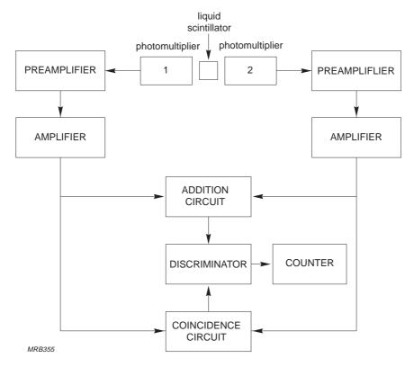
Fig.7.6 Schematic diagram of a liquid scintillation counter
