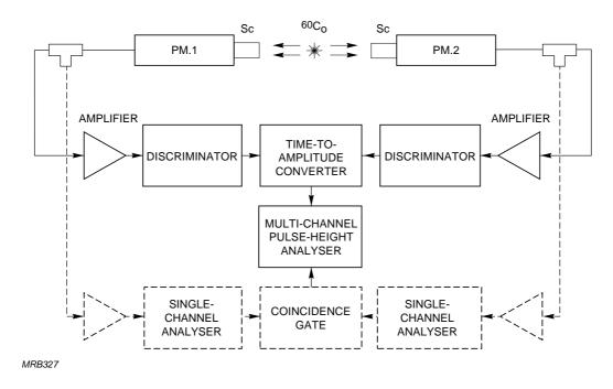
Fig.6.26 Basic setup for time spectrometry
