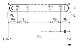
Fig.5.2 Negative-polarity voltage supply
