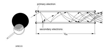
Fig.1.15 Electron multiplication in a microchannel
