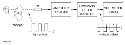
Fig.3.13 Set-up for measuring noise equivalent power
