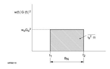
Fig.A3.1 Definition of noise pass-band B<sub>N</sub>.
