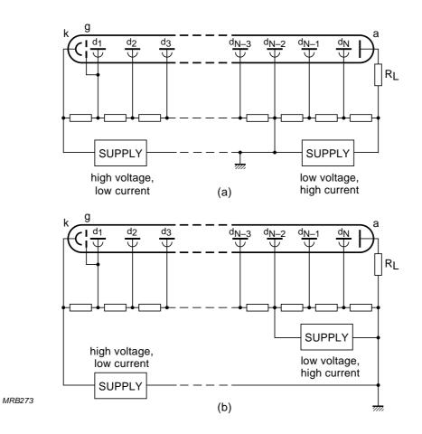
Fig.5.9 Dual voltage supplies: (a) series, (b) parallel
