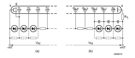
Fig.5.8 Inter-electrode voltage stabilization with zener diodes: (a) in first stages, (b) in last stages (dashed lines, protection resistors)
