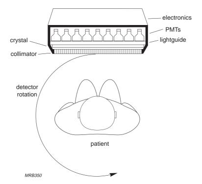
Fig.7.3 Principle of single-photon emission computed tomography (SPECT). The γ-camera head (sometimes 2 or 3) is moved around the patient and acquires projections from several angles. These are back-projected by computer to give transversal slices
