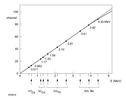
Fig.4.18 Distribution of γ-ray energies emitted by a source consisting of <sup>60</sup>Co, <sup>137</sup>Cs, <sup>232</sup>Th and AmBe as used in measuring photomultiplier linearity. Vertical scale, channel number of multichannel pulse-height analyser
