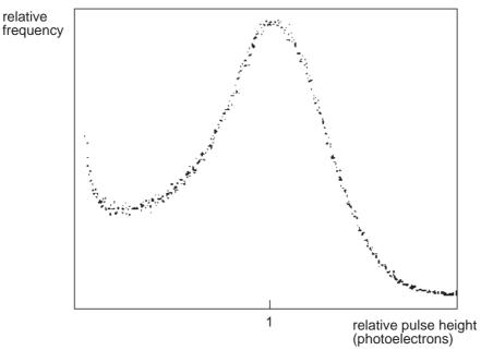
Fig.2.4 Typical single-electron spectrum. Resolution 67% FWHM. Peak-to-valley ratio 2.8:1
