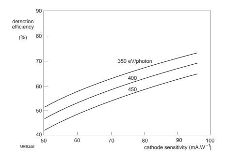
Fig.7.7 Detection efficiency as a function of photocathode sensitivity for <sup>3</sup>H, with energy loss as parameter
