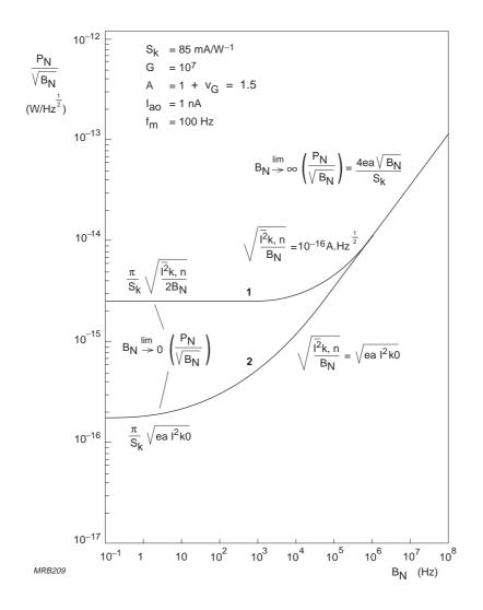
Fig.3.12 Noise equivalent power (flux as a function of the measuring circuit passband, for two value of additional noise: 1)  $10^{-16}$  A/Hz<sup>1/2</sup>, 2)  $7 \times 10^{-18}$  A/Hz<sup>1/2</sup>
