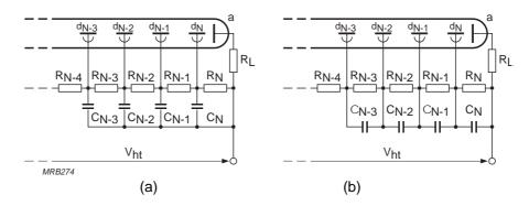
Fig.5.10 Dynode decoupling: (a) parallel, (b) series.
