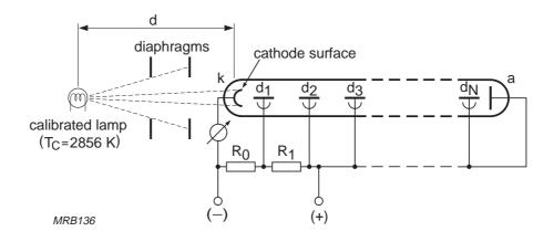
Fig.2.11 Set-up for measuring cathode sensitivity
