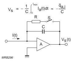
Fig.5.34 Integrator. For integrating the charge due to light pulses, t<sub>min</sub> must exceed the pulse duration. Switch S discharges the capacitor between pulses
