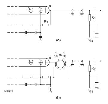
Fig.5.14 Voltage supply via the output cable
