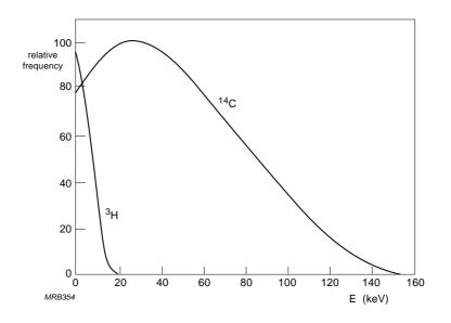
Fig.7.5 Relative spectral energy E of  $\beta$  emission from tritium (^3H) and carbon (^14C)
