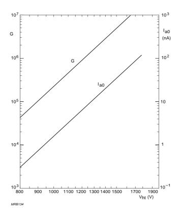
Fig.2.8 Examples of photomultiplier gain and anode darkcurrent variation as functions of applied voltage
