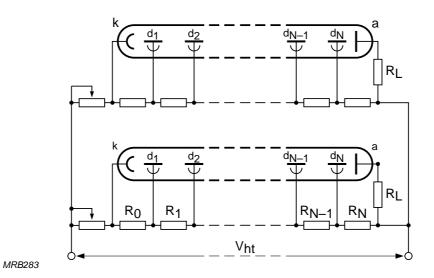
Fig.5.21 High-voltage supply to photomultipliers in parallel
