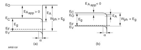
Fig.A1.7 Energy-band diagrams showing (a) positive and (b) negative electron affinity
