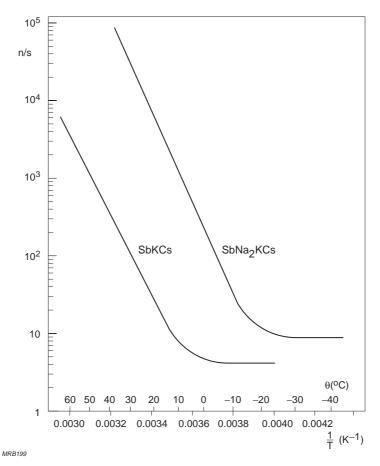
Fig.3.1 Number of dark pulses per second as a function of temperature, for SbKCs and SbNa<sub>2</sub>KCs photocathodes
