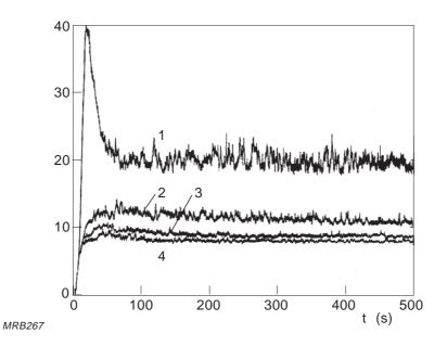
Fig.5.3 Stabilization of anode dark current  $I_{ao}$  (arbitrary scale) following gradual application of voltage in negative polarity, showing the effect of different ways of insulating the tube from its magnetic shield.
