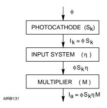
Fig.2.3 Photomultiplier sensitivity characteristics
