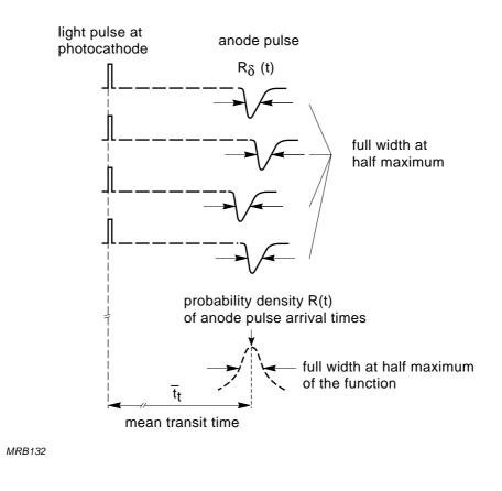
Fig.2.7 Response-pulse jitter due to transit time fluctuations
