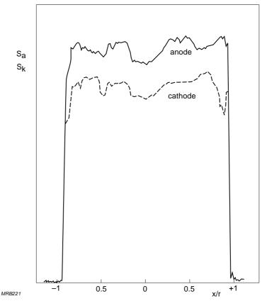
Fig.4.2 Example anode and cathode sensitivity variation measured at  $\lambda = 424$  mm along one cathode diameter of a photomultiplier with a 32 mm SbKCs cathode. Vertical axis, relative sensitivity (arbitrary scale); horizontal axis, distance from cathode centre, normalized with respect to cathode radius. Curves offset for clarity
