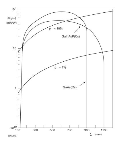
Fig.1.4 Spectral sensitivity characteristics for two negative-electron-affinity photocathode materials; quantum efficiency curves  $\rho = 1\%$  and  $\rho = 10\%$  shown for reference
