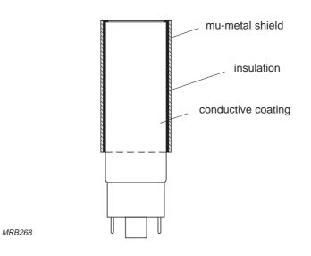
Fig.5.4 Magnetic shielding, insulation, and conductive coating
