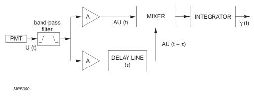
Fig.5.38 Autocorrelation detector
