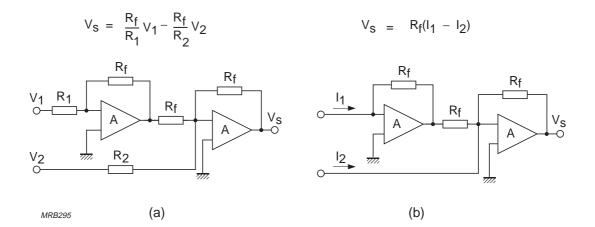
Fig.5.33 (a) Voltage subtractor, (b) current subtractor
