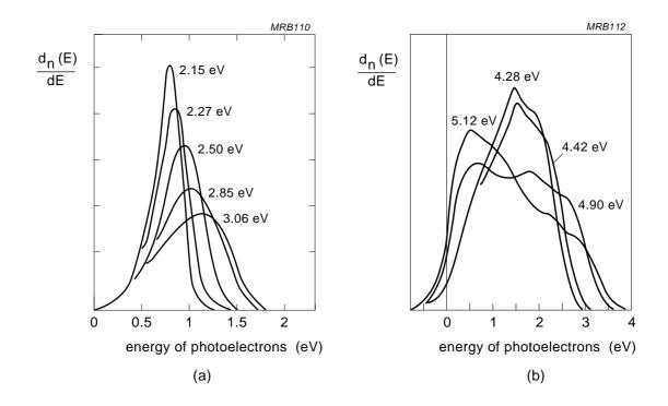
Fig.A1.8 Relative distribution of photoelectron energies, E<sub>ph</sub>, from a layer of SbKCs at 290 K, for incident photon energies (a) from 2.15 eV to 3.06 eV, and (b) from 4.28 eV to 5.12 eV
