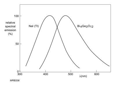
Fig.A6.8 Normalized emission spectra of NaI(TI) and Bi<sub>4</sub>Ge<sub>3</sub>O<sub>12</sub>
