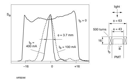
Fig.5.24 Effective-cathode-area reduction due to a solenoid surrounding the cathode (32 mm diameter S1 cathode)
