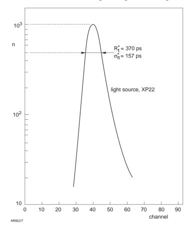
Fig.4.9 Time resolution of a fast-response photomultiplier, for single-electron pulses originating from a single point on the cathode at an illumination wavelength of 560 nm, measured according to the method of Fig.4.8. Vertical axis, number of pulses per channel (arbitrary scale); horizontal axis, channel number (about 40 ps per channel)
