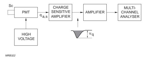
Fig.6.19 Energy spectrometer using a multichannel pulse-height analyser
