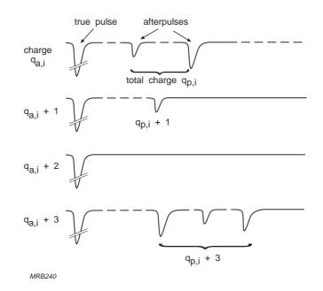
Fig.4.26 Examples of the development in number and charge of afterpulses
