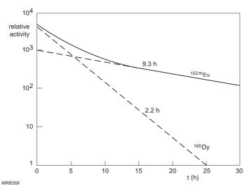
Fig.7.9 Illustration of the graphical separation of two half lives
