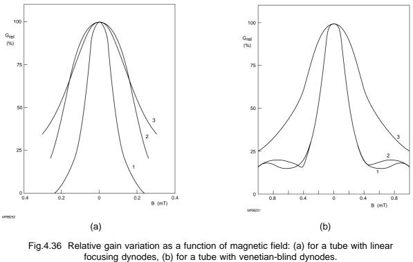
curve 1: field aligned with y-axis (Fig.4.35) curve 2: field aligned with x-axis curve 3: field aligned with z-axis
