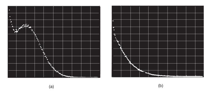
Fig.2.10 Examples of dark-current pulse spectra (a) with linear-focusing CuBe dynodes, and (b) with venetian blind dynodes. Vertical axes, pulse frequency; horizontal axes, pulse amplitude
