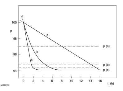
Fig.4.22 Anode sensitivity curves showing the same absolute change over 16 hours but different values of mean gain deviation (MGD) according to the ANSI method. Curve a: MGD = 1.6%; curve b: MGD = 1.1%; curve c: MGD = 0.75%; p(a), p(b) and p(c) are the corresponding mean heights of the pulse peak averaged over 17 readings
