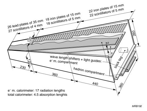
Fig.7.15 Calorimeter tower based on the wavelength shifter principle (courtesy of CERN, experiment UA 2)
