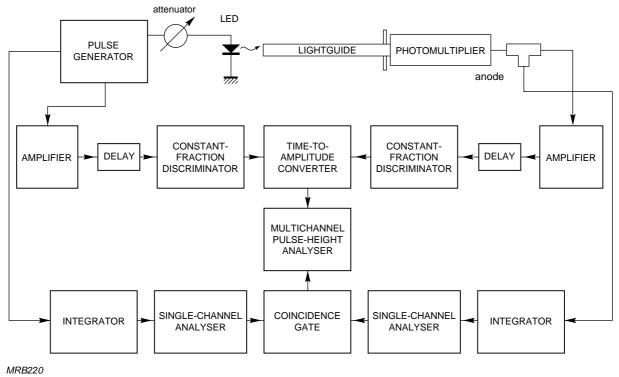
Fig.4.8 Set-up for measuring transit-time differences and transit-time spread
