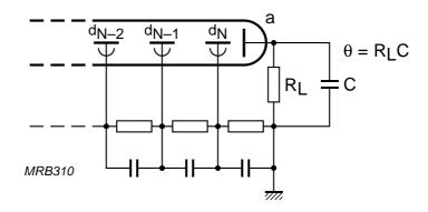
Fig.6.7 Anode circuit with the anode load  $\rm R_L C$
