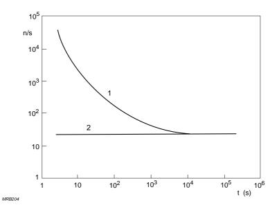
Fig.3.6 Dark-current behaviour following application of high voltage in 1) negative, 2) positive polarity. Vertical scale, number of dark pulses per second
