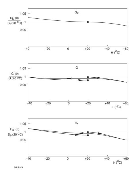
Fig.4.34 Temperature variation of cathode and anode sensitivity and gain of a tube with a bialkali cathode at a wavelength of 405 nm, showing hysteresis.
