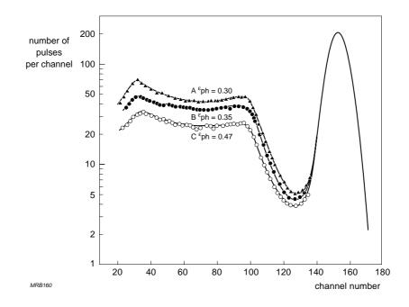
Fig.6.25 Scintillation pulse amplitude distributions with <sup>137</sup>Cs sources and scintillators of dimensions  $\phi$ 38 mm  $\times$  25 mm (A),  $\phi$ 50 mm  $\times$  50 mm (B) and  $\phi$ 75 mm  $\times$  75 mm (C). The distributions are normalized to give the same area under their full energy peak curves
