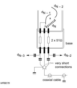
Fig.5.12 Connection of damping resistors and decoupling capacitors to the last two dynodes
