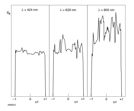
Fig.4.3 Examples of cathode sensitivity variation measured along one diameter of a SbNa<sub>2</sub>KCs cathode at three wavelengths
