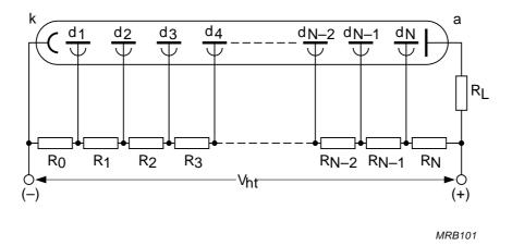
Fig.1.2 Voltage-divider high-tension supply
