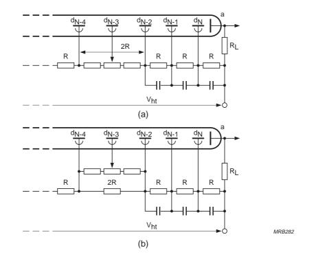
Fig.5.20 Alternative circuits for adjusting gain by adjusting the voltage of one dynode
