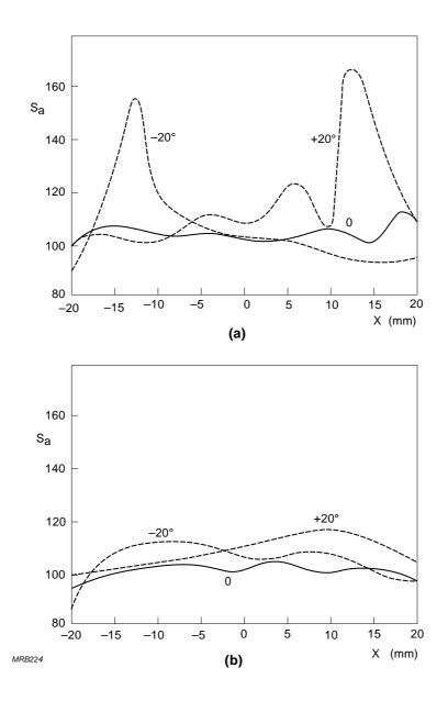
Fig.4.5 Examples of relative anode sensitivity variation at three angles of incidence, measured at  $\lambda = 629$  mm along one diameter of a tube with SbNa<sub>2</sub>KCs cathode; with (a) polished and (b) frosted input window. x is the distance from the cathode centre
