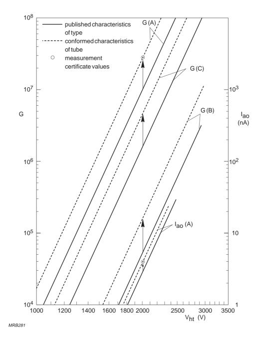
Fig.5.18 Conforming the measured gain and dark current characteristics of an individual tube to the published characteristics of the type. G(A), G(B)) and G(C) are the gain characteristics with the recommended type A, B and C voltage dividers; I<sub>ao</sub>(A), the dark current with the recommended type A voltage divider
