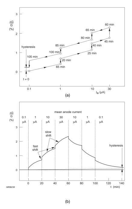
Fig.4.25 Gain change of a photomultiplier with one short and one long stabilization time constant: (a) as a function of mean anode current, (b) as a function of time. Measuring conditions as for Fig.4.24
