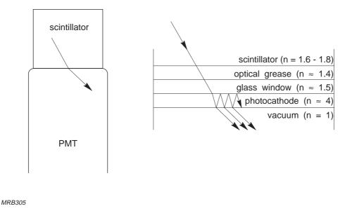
Fig.6.2 Light transmission through the window and through the photocathode
