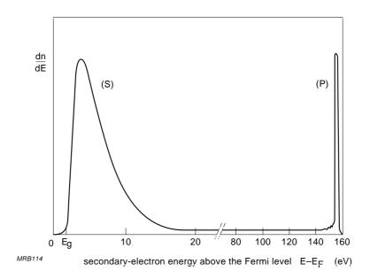
Fig.A1.11 Distribution of secondary-electron energies E above the Fermi level  ${\rm E_{F}}.$
