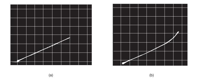
Fig.4.17 Oscillogram obtained by the method of Fig.4.16 showing (a) linear and (b) non-linear response. Scales, 50 mA/div
