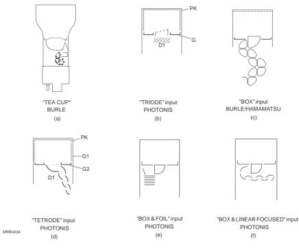
Fig.7.2 Examples of γ-camera tube input systems
