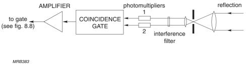
Fig.8.9 The use of a coincidence detector to reduce spurious responses in laser telemetry
