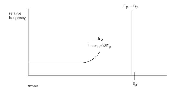
Fig.6.24 Spectrum of primary electron energies produced in a scintillator by monoenergetic  $\gamma$  radiation of energy  $\mathsf{E}_{\mathsf{p}}$ , showing the Compton continuum, the Compton edge and the photoelectric line
