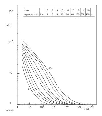
Fig.3.4 Dark-current decay of an S13 cathode at 0 °C following exposure to an incident flux of 120  $\mu$ W at  $\lambda$  = 366 nm, with exposure time as parameter. Vertical scale, relative number of electrons per second
