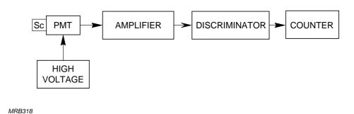
Fig.6.15 Block diagram of a scintillator pulse counter
