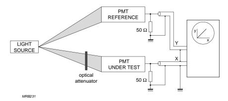
Fig.4.16 Set-up for the XY-method of measuring linearity
