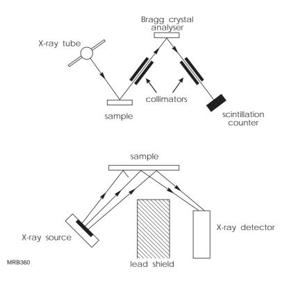
Fig.7.11 Schematic diagram of two X-ray spectrometers (a) dispersive, (b) non-dispersive
