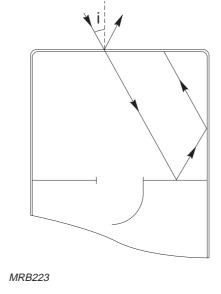
Fig.4.4 Light that passes through a semitransparent cathode may be reflected back to it by internal surfaces
