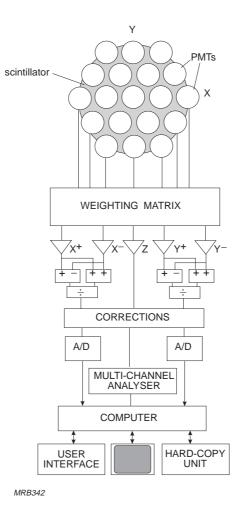
Fig.7.1 Operating principle of a  $\gamma$ -camera
