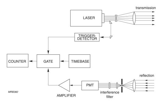
Fig.8.8 Principle of laser telemetry
