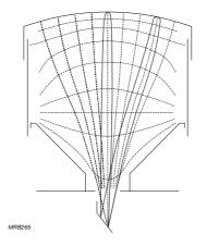
Fig.1.7 Example of a large fast photomultiplier input optics
