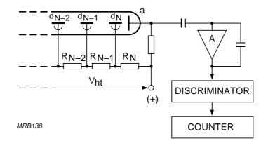
Fig.2.13 Dark-pulse-rate measurement
