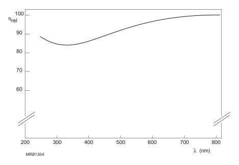
Fig.2.2 Example of relative input system collection efficiency as a function of wavelength
