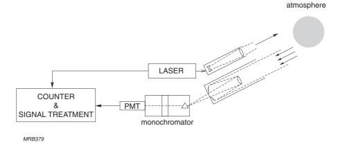
Fig.8.6 Principle of Raman spectrometry for measuring atmospheric pollution using a laser as the excitation light source
