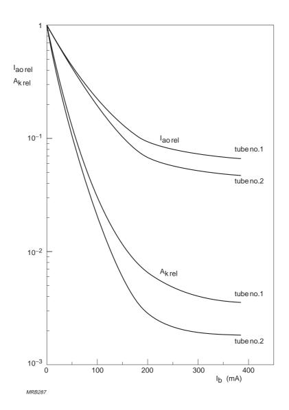
Fig.5.25 Relative dark-current  $(I_{a0})$  and cathode-area  $(A_k)$  reduction as functions of solenoid current  $I_b$  in two tubes with 32 mm diameter S1 cathodes, using the method of Fig.5.24. Note that the dark-current reduction is much less than the effective-cathode-area reduction
