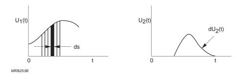
Fig.A4.2 Superposition of elemental pulses
