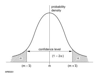
Fig.6.17 The confidence level is the probability that an observation  $\overline{x}$  is within a given percentage of the origin m of the distribution
