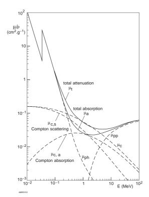
Fig.A6.5 Mass attenuation and mass absorption coefficients for X- and  $\gamma\text{-radiation}$  in Nal(Tl),  $\rho$  = 3,67 g/cm^3
