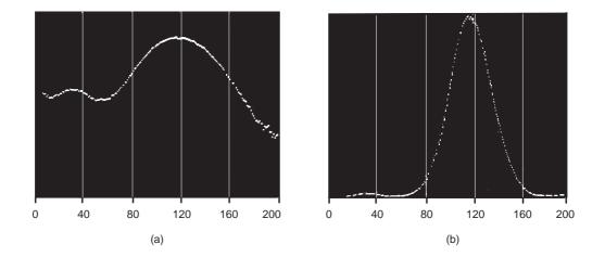
Fig.6.22 Scintillation pulse amplitude distribution for a  ${}^{55}$ Fe source with (a) a logarithmic and (b) a linear scale on the y axis
