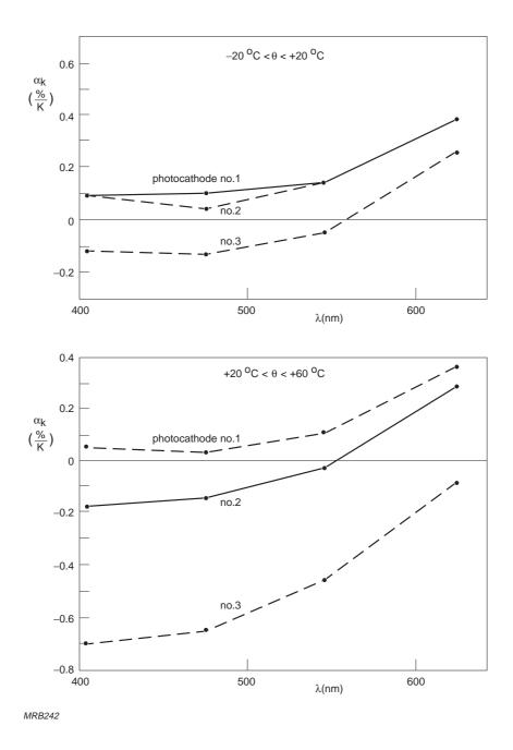
Fig.4.28 Examples of the variation of the temperature sensitivity coefficient  $\alpha_k$  of type S11 cathodes as a function wavelength
