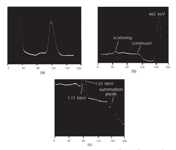
Fig.6.21 Scintillator pulse amplitude distribution using sources of (a) <sup>57</sup>Co, (b) <sup>137</sup>Cs and (c) <sup>60</sup>Co
