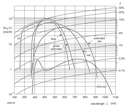
Fig.1.3 Spectral sensitivity characteristics for various photocathode types. Curves of uniform quantum efficiencies, ρ, are shown for reference; see ch.2.1.2.
