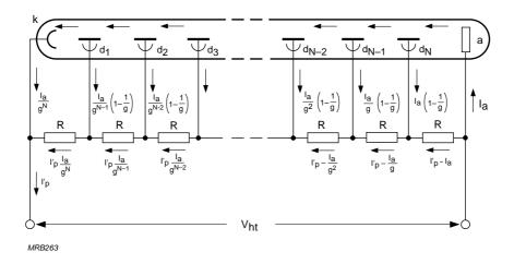
Fig.4.11 Current distribution in an iterative voltage divider
