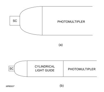
Fig.6.4 Logarithmic-spiral light guide (a) between scintillator and PMT, (b) with an intermediate cylindrical light guide
