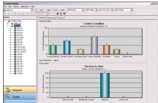
InSight control performance monitoring.
