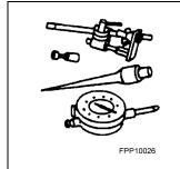
Dial Indicator with Bracketry TOOL-4201-C or Equivalent
