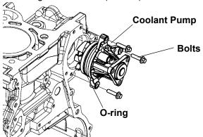
48. Install coolant pump pulley and 3 bolts:
