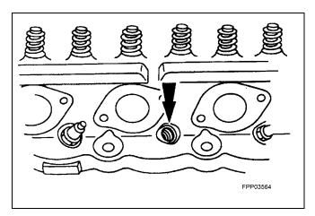
2. Start the tap into the spark plug hole, being careful to keep it properly aligned. As the tap begins to cut new threads, apply aluminum cutting oil
