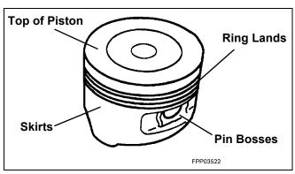
2. Use the Piston Ring Groove Cleaner to clean the piston ring grooves.
