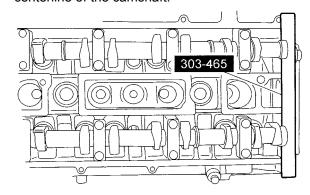
**NOTE:** Use a wrench on the flats between cylinders No.1 and No. 2 to hold the camshafts in place.
