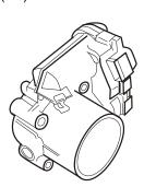
The Electronic Actuator also acts as an idle air control (IAC) valve. Changes in engine load are detected by the GCP by comparing manifold absolute pressure (TMAP) with throttle position. When the GCP detects a change in engine load, it can adjust idle speed by changing the PWM signal to the actuator.
