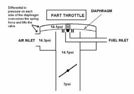
The greater the airflow into the engine, the greater the pressure drop across the diaphragm and the more lift occurs on the fuel valve. This allows more fuel to be
