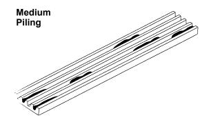
If heavy deposits are apparent, resulting in noise and belt instability, install a new belt.
