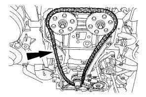
32. Remove 2 bolts and left timing chain guide.
