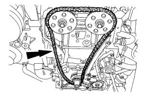
6. Remove the 2 bolts and left timing chain guide.
