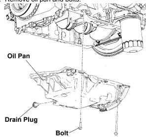
CAUTION: Do not use metal scrapers, wire brushes, power abrasive discs or other abrasive means to clean the sealing surfaces. These tools cause scratches and gouges which make leak paths. Use a plastic scraping tool to remove all traces of old sealant.
