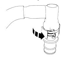
5. Pull on the fitting to make sure it is fully engaged.
