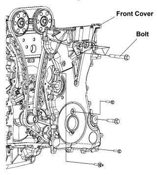
CAUTION: Do not use metal scrapers, wire brushes, power abrasive discs or other abrasive means to clean the sealing surfaces. These tools cause scratches and gouges which make leak paths. Use a plastic scraping tool to remove all traces of old sealant.
