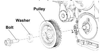
CAUTION: Only hand tighten crankshaft pulley bolt or damage to front cover can occur.
