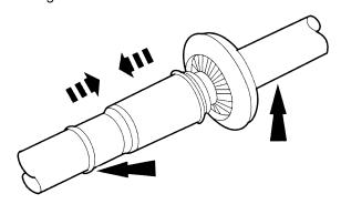
4. Make sure the coupling is engaged by pulling on the lines and install the safety clip.
