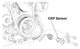
7. Install an M6 bolt in the position shown.
