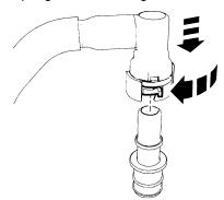
4. Position the locking tab into the latched position.
