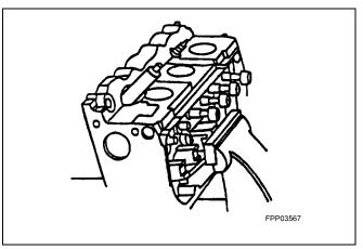
7. Turn the mandrel body approximately one-half turn counterclockwise and remove.
