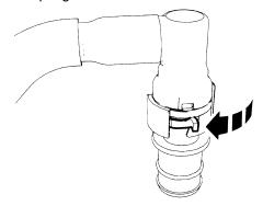
3. Separate the quick connect coupling from the fitting
