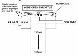
While the carburetor is designed to mix the fuel and air and adjust fuel to match the speed and load of the engine, it has only "ballpark" accuracy. This accuracy is not fine enough to achieve emissions targets. To achieve accurate fueling, the air inlet pressure to the carburetor is controlled by an Electronic Pressure Regulator (EPR).
