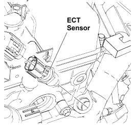
After engine start-up, the temperature should rise steadily to about 85°C (185°F). It then stabilizes when the thermostat opens. If the engine has not been run for several hours (overnight), the engine coolant temperature and intake air temperature displays should be close to each other. A fault in the engine coolant sensor circuit will set a DTC 221 or DTC 222.
