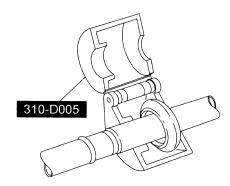
4. Close and push the special tool into the open side of the cage.
