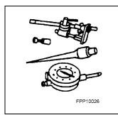
Dial Indicator with Bracketry TOOL-4201-C or Equivalent
