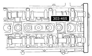
**NOTE:** Camshaft timing slots are offset. If special tool cannot be installed, rotate crankshaft one complete revolution clockwise to correctly position camshafts.
