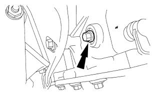
5. Install special tool 303-507 and turn the crankshaft pulley bolt to position the No. 1 cylinder at top dead center (TDC).
