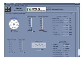
Recording the values and voltages can be a very useful tool while diagnosing engine problems. The FORD diagnostic software includes real time **plotting** and real time **logging** capabilities. These features enhance the ability to diagnose and repair possible problems with the FORD system. Both plotting and logging allows the user to record, in real time, any variable that can be seen in the FPP\_Dis software. In order to record variables, the FPP\_Dis software must be "Connected" to the GCP.
