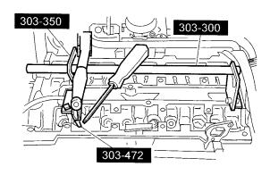
4. Remove the valve spring retainer and valve spring.
