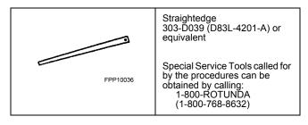
Use a straight edge and a feeler gauge to inspect the cylinder head for flatness. Compare with specifications. If the cylinder head is distorted, install a new cylinder head.
