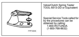
Use the Valve/Clutch Spring Tester to check the valve springs for proper strength at the specified valve spring length.
