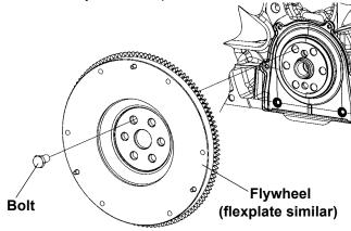
**CAUTION:** Special bolts are used for installation. Do not use standard bolts.
