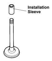
2. Using special tool 303-470, install a new valve seal.
