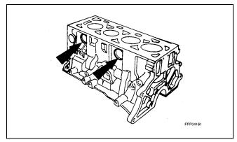
Inspect the cylinder block plug bore for any damage that would interfered with the proper sealing of the plug. If the cylinder block plug bore is damaged, bore for the next oversize plug.
