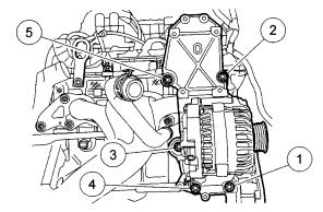
63. Install A/C compressor (if equipped) and bolts:
