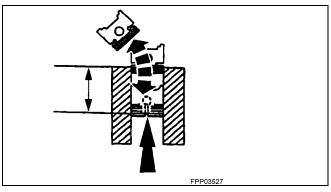
Use a feeler gauge to measure the top piston ring end gap and the second piston ring end gap.
