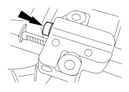
19. Using a small pick, push back and hold the ratchet mechanism.
