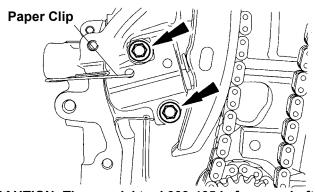
CAUTION: The special tool 303-465 is for camshaft alignment only. Using this tool to prevent engine rotation can result in engine damage.
