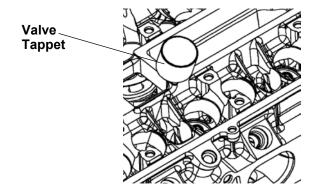
**NOTE:** Coat valve tappets with clean engine oil prior to installation.
