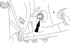
40. Position a new crankshaft position (CKP) sensor and loosely install 2 bolts.
