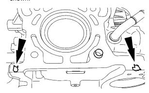
**NOTE:** If not secured within 4 minutes, the sealant must be removed and the sealing area recleaned as before. Refer to previous CAUTION & WARNING.
