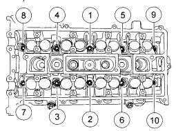
CAUTION: Install the camshafts with alignment slots in the camshaft lined up so the camshaft alignment plate can be installed without rotating the camshafts. Make sure the lobes on the No.1 cylinder are in the same position as noted in the disassembly procedure. Rotating the camshafts or installing the camshafts 180 degrees out of position can cause severe damage to the valves and pistons.
