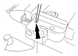
20. While holding the ratchet mechanism, push the ratchet arm back into the tensioner housing.
