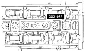
CAUTION: Do not rely on the Camshaft Alignment Plate to prevent camshaft rotation. Damage to the tool or the camshaft can occur.
