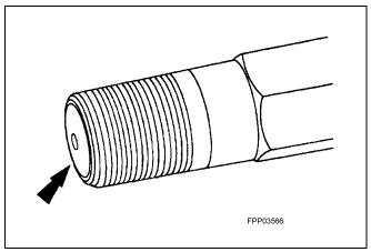
**NOTE:** A properly installed tapersert will be either flush with or 1.0 mm (0.039 inch) below the spark plug gasket
