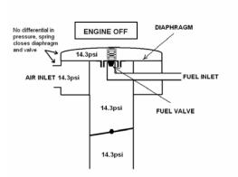
The variable venturi carburetor controls fuel flow based on a differential pressure across the diaphragm. The more air the engine demands, the lower the pressure in the throat and hence on the top of the diaphragm. When the pressure on the top of the diaphragm is low enough, the diaphragm overcomes the spring force holding it down and lifts and allows fuel to be drawn from the fuel port into the air flow into the engine.
