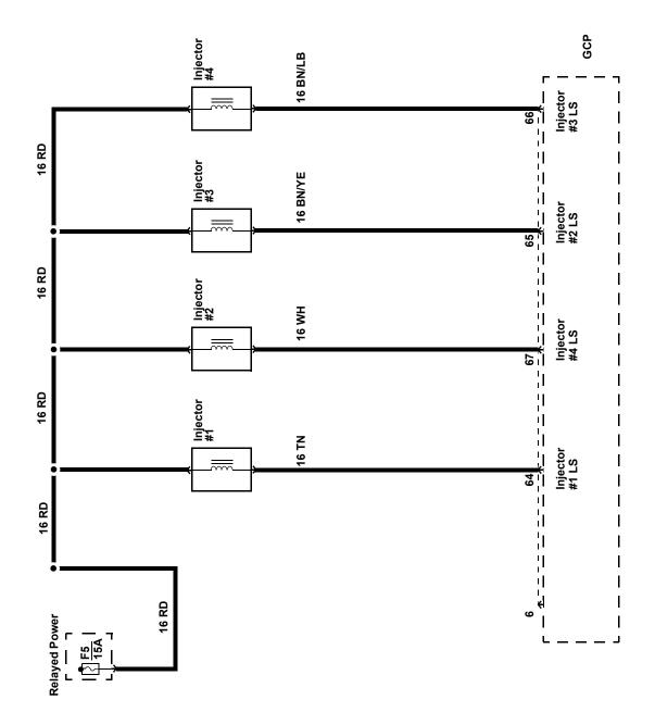
Engine Controls - Actuator / Data Link Connector (DLC)
