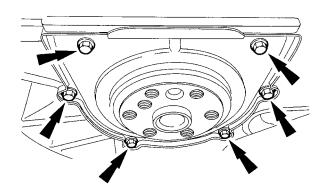
47. Remove bolts, oil pump pickup tube and discard gasket.
