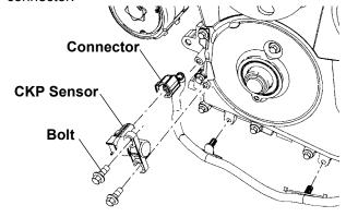
CAUTION: A new CKP Sensor must be installed whenever the old sensor is removed.
