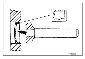
Cylinder Block Core Plug - Expansion-Type
