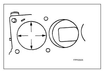
**NOTE:** For precision fit, new pistons are divided into three categories within each size range based on their relative position within the range. A paint spot on the new pistons indicates the position within the size range.
