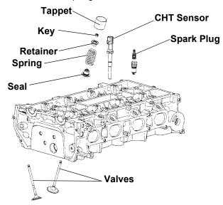
4. Using special tools 303-350, 303-300 and 303-472, compress valve spring and install retainer keys.
