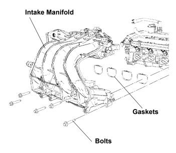
4. Remove 5 bolts and the intake manifold.
