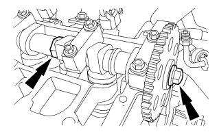
34. Release tension on oil pump chain tensioner.
