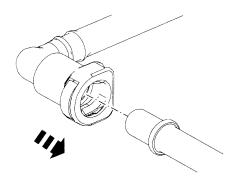
4. Pull on the fitting to make sure it is fully engaged.
