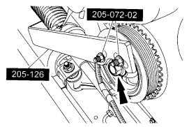
CAUTION: Failure to hold the crankshaft pulley in place during bolt loosening can cause damage to the engine.
