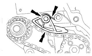
**NOTE:** Sprockets must turn freely on the camshafts. 17. Position camshaft sprockets and loosely install bolts.
