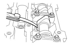
**NOTE:** Measure each valve's clearance at base circle with lobe pointed away from the tappet, before removing camshafts. Failure to measure all clearances prior to removing camshafts will necessitate repeated removal and installation and wasted labor time.
