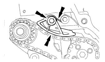
35. Remove the bolt and tensioner.
