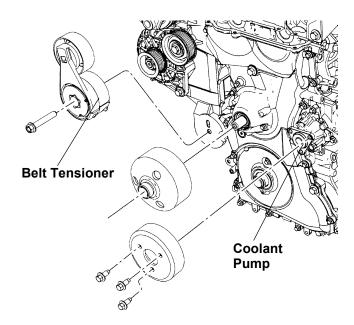
The coolant pump circulates the coolant through the engine block and cylinder heads to the thermostat. If the thermostat is closed, the coolant returns to the coolant pump through a bypass hose. Once the coolant reaches a specified temperature, the thermostat will open, allowing the coolant to flow to the radiator for heat transfer and back to the coolant pump inlet.
