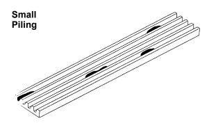
Longer deposits building up to 50% of the rib height is also not a concern, except it can result in excessive noise.
