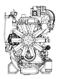
The dual camshafts are chain driven with an automatic tensioning system. The valve train components are alternate fuel ready. Spark is delivered by an individual coil on plug ignition system. A broadband knock sensor is calibrated for individual cylinder use.
