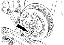
31. Rotate the crankshaft pulley as necessary to align the bolt holes.
