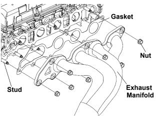
60. Position a new gasket and install exhaust manifold and 7 new nuts:
