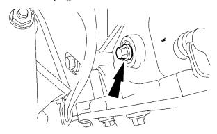
CAUTION: Installing special tool in this next step will prevent engine from being rotated in the clockwise direction. However, the engine can still be rotated in the counterclockwise direction. Only turn the engine in the normal direction of rotation.
