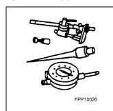
Dial Indicator with Bracketry TOOL-4201-C or Equivalent
