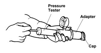
**NOTE:** If the plunger of the pressure tester is depressed too fast, an incorrect pressure reading will result.
