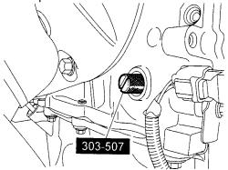
CAUTION: Only hand tighten the bolt in the next step or damage to the front cover can occur.
