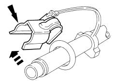
3. Install special tool 310-D005 as shown.
