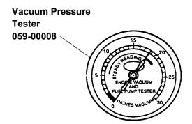
The vacuum gauge should read between 51-74 kPa (15-22 in-Hg) depending upon the engine condition and the altitude at which the test is performed. Subtract 5.5 kPa (1 in-Hg) from the specified reading for every 500 meters (1,000 feet) of elevation above sea level.
