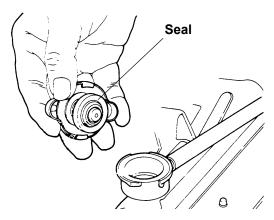
2. Fit the radiator cap to the pressure tester using an adapter.
