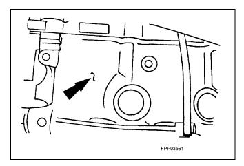
Repair porosity defects with an epoxy sealer meeting Ford specification M3D35-A (E).
