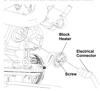
**NOTE:** Do not loosen the screw more than necessary for removal.
