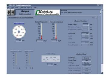
Most applicable sensor and actuator values are displayed on the Gauges Screen. The display shows the voltage the FORD system GCP is reading and, for sensors, the sensor value in engineering units.
