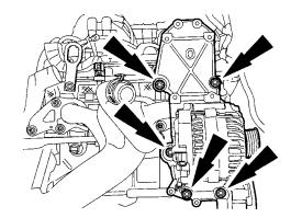
7. Remove nuts and exhaust manifold. Discard nuts.
