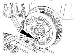
8. Using special tool 303-465, check the position of the camshaft. If it is not possible to install the special tool, correct the engine timing.
