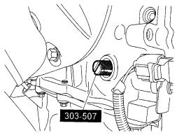
CAUTION: Only hand tighten the bolt in this next step or damage to the front cover can occur.
