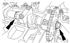
**NOTE:** Use the flats on the camshaft to prevent camshaft rotation.
