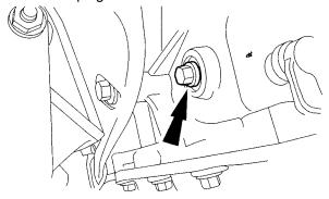
CAUTION: Only turn the engine in the normal direction of rotation. Installing the special tool in this next step will prevent the engine from being rotated in the clockwise direction. However, the engine can still be rotated in the counterclockwise direction.
