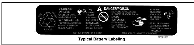
The handling and correct use of lead acid batteries is not as hazardous provided that sensible precautions are observed and that operatives have been trained in their use and are adequately supervised. It is important that all labeling on the battery is carefully read, understood and complied with. The format of the following symbols and labels is common to most brands of lead acid battery.
