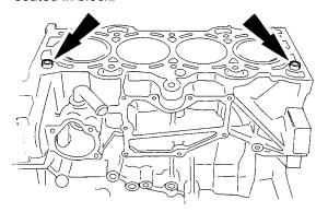
**NOTE:** If cylinder head is not secured within 4 minutes, the sealant must be removed and the sealing area recleaned -- Refer to "Engine Cleaning" on page 34 of this section.
