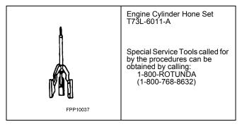
**NOTE:** Before any cylinder bore is honed, all main bearing caps must be installed so the crankshaft bearing bores will not become distorted.
