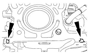
10. Install a new gasket and position cylinder head.
