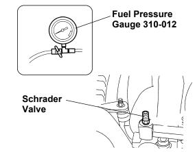
If fuel pressure is insufficient, check for a clogged pump filter, screen or fuel filter. Also check for a break or restriction in the fuel lines. If fuel pump is inoperative, check for damaged or loose ground or improper wiring. Make sure fuel lines connections area tight and not leaking.
