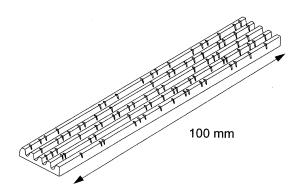
If cracks are beyond acceptable or, any chunks are found to be missing from the ribs, a new belt must be installed.
