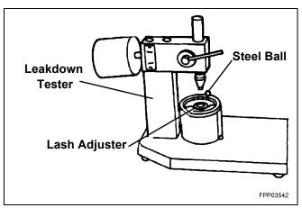
Adjust the length of the ram so the pointer is just below the start timing mark when the ram contacts the hydraulic lash adjuster. Start Timing as the pointer passes the start timing mark and end timing as the pointer reaches the center mark.
