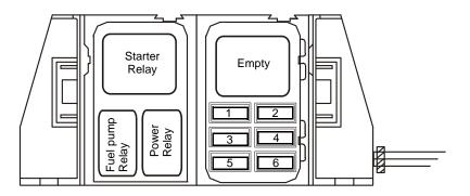
Fuse **Circuits protected Amps** Battery Voltage to EPR 10 1 2 5 Ignition Voltage to GCP and Relays 3 10 Battery Voltage to GCP 4 15 Fuel pump 5 15 Battery Voltage out of Power Relay 6 -Not used
