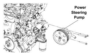
CAUTION: There is one bolt behind the cooling fan drive pulley. This bolt can be accessed by lining up one of the holes in the pulley with the bolt.
