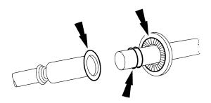
CAUTION: Make sure the fuel tube clicks into place when installing the tube. To make sure that the fuel tube is fully seated, pull on the tube.
