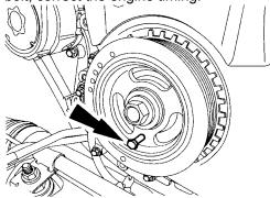
37. Using special tool 303-465, check the position of the camshafts. If it is not possible to install the special tool, correct the engine timing.
