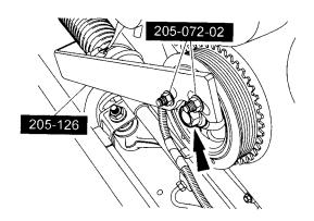
CAUTION: Failure to hold the crankshaft pulley in place during bolt loosening can cause damage to the engine.
