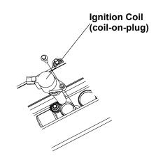
The coil-on-plug design has individual coils mounted directly over each spark plug. Each cylinder is paired with its opposing cylinder in the firing order, so that one cylinder on compression fires simultaneously with the opposing cylinder on exhaust. The spark that occurs in the cylinder on the exhaust stroke is referred to as a "waste spark".
