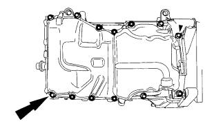
46. Remove bolts and rear seal retainer plate.
