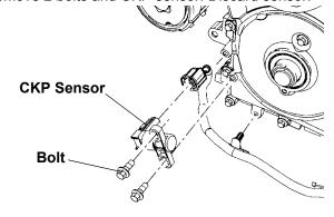
CAUTION: Failure to position the No. 1 piston at top dead center (TDC) can result in damage to the engine. Turn the engine in the normal direction of rotation only.
