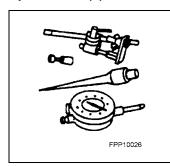
Dial Indicator with Bracketry TOOL-4201-C or Equivalent
