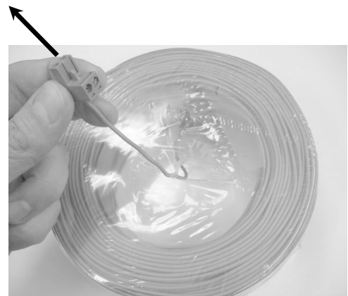
Figure 1.12 – Pull out the wire from the plastic covering – do not remove the covering; it is designed as a dispenser.
