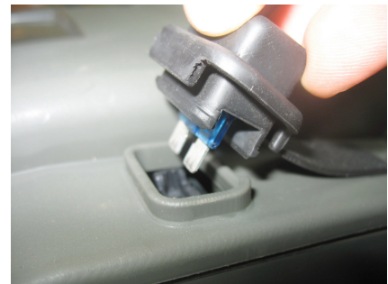
Figure 1.27 - Inserting batteries fuse
