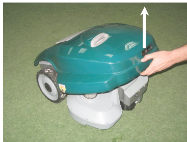
Figure 1.25 - Lifting the Bumper Cover
