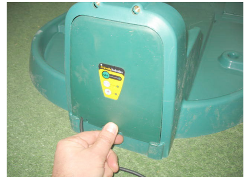
Figure 1.22 - Closing the Base Station cover
