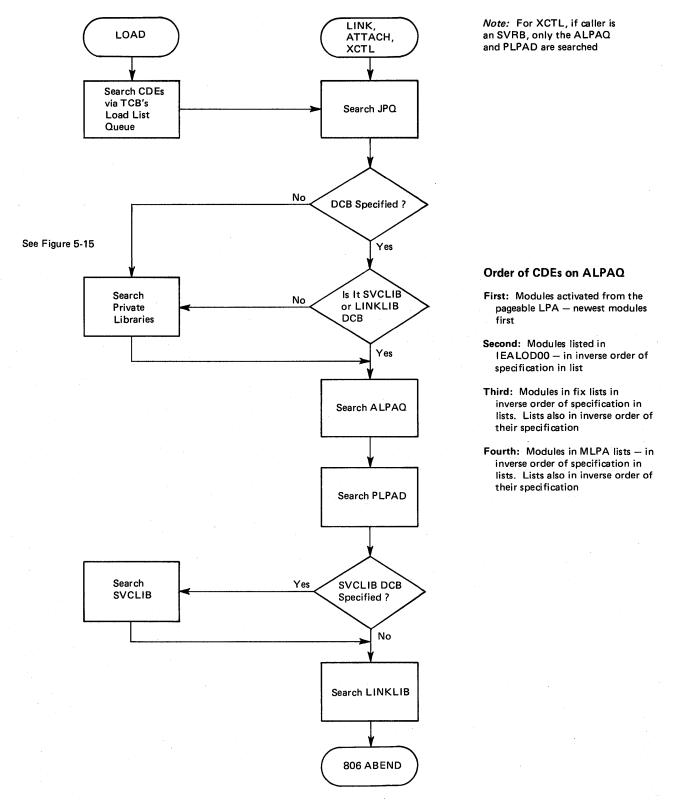
Figure 5-14. Module Search Sequence for LINK, ATTACH, XCTL and LOAD
