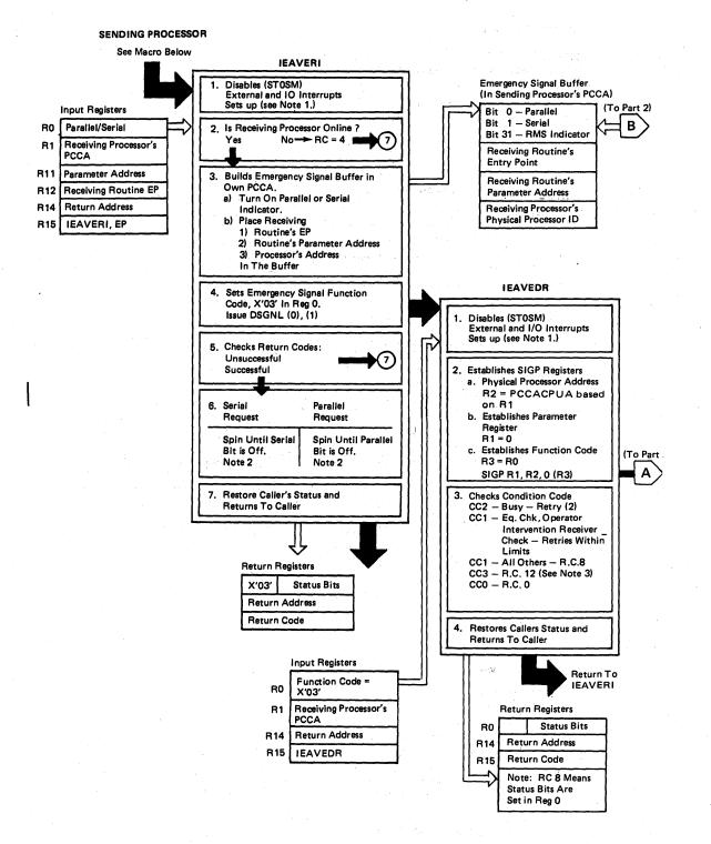
Figure 2-11. Emergency Signal (EMS) Process Flow (Part 1 of 2)
