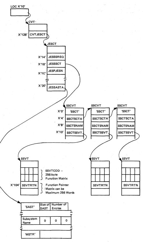
Figure 5-50. Subsystem Interface Control Block Usage
