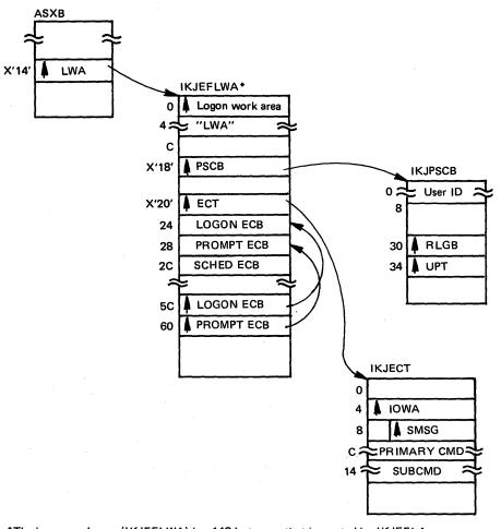
\*The logon work area (IKJEFLWA) is a 148-byte area that is created by IKJEFLA and is pointed to by ASXB and JSXL. It contains control block pointers, entrance lists, and parameter lists that are required for logon/logoff.
