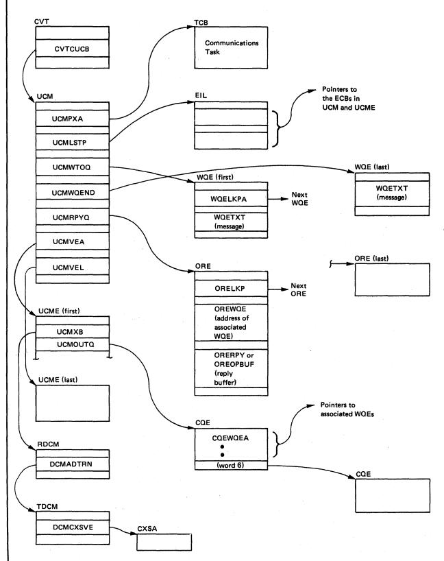
Figure 5-54. Communications Task Control Block Structure
