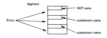
The node name is in the first eight bytes of each RDT entry. Stop chaining through the RDT entries when the major node name (that is, NCP or LBUILD) is found; then scan down the RDT entries of this major node until the node in question is found. Offset X'28' of the appropriate RDT entry points to the DNCB (offset X'28' from beginning of name). DNCB + X'10' points to the FMCB.
