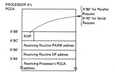
By locating the proper PCCA (in this case processor A's), you can determine whether the EMS request was parallel or serial, the entry point, and, therefore, the name of the receiving routine. Although this information tells quite a bit about the current process on processor A, the real problem, however, is most likely on processor B. Three past experiences can help determine the state of processor B.
