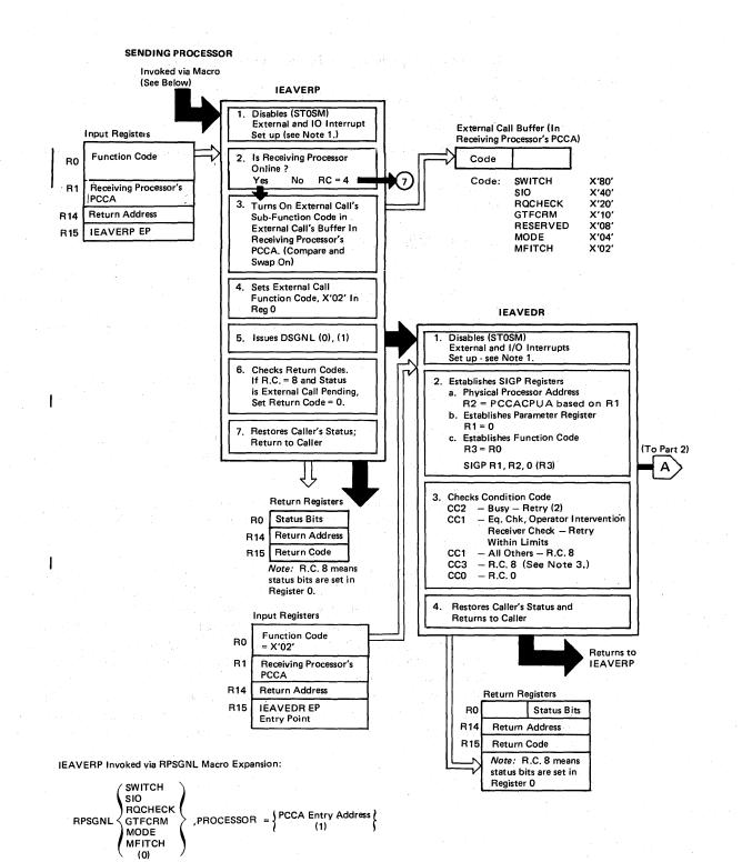
Figure 2-10. External Call (XC) Process Flow (Part 1 of 2)
