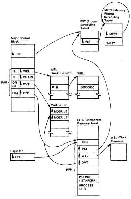
Figure 5-32. VTAM Control Block Structure
