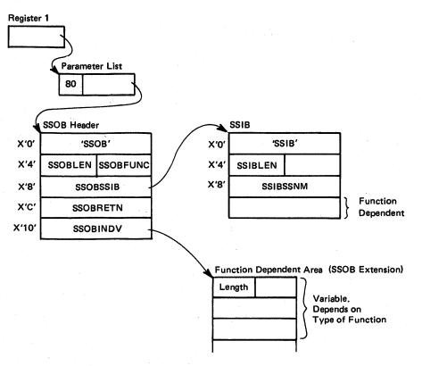
Figure 5-51. Control Block Structure for Invoking Subsystem Interface
