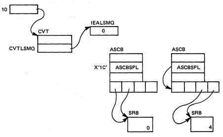
Figure 5-2. Local SRB Queue Structure and Control Block Relationships
