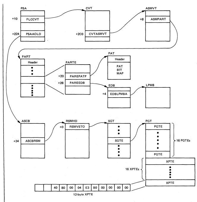
Figure 5-28. Relating the Virtual Address to the PART and PAT
