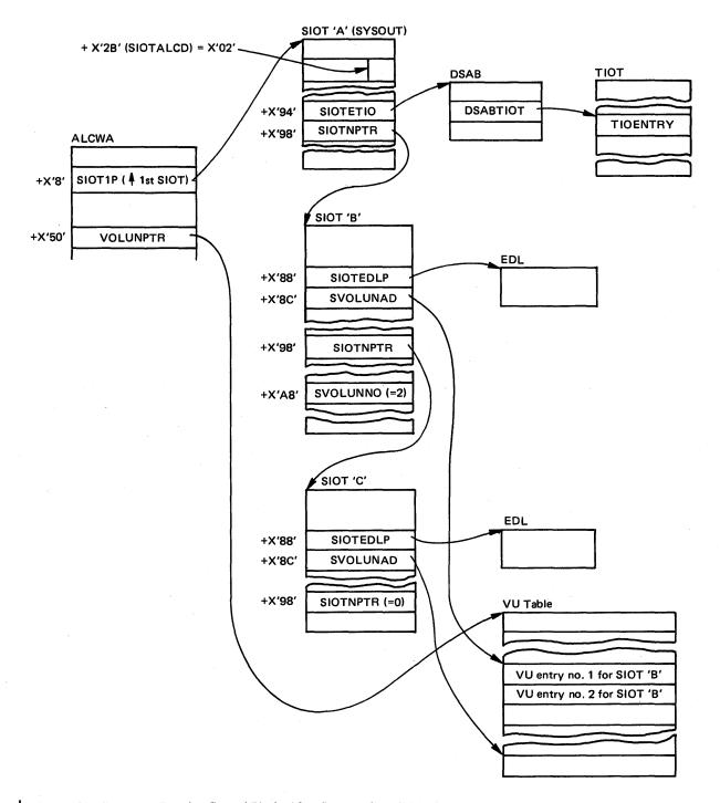
Figure 5-38. Common Allocation Control Blocks After Construction of Volunit Table and EDLs.
