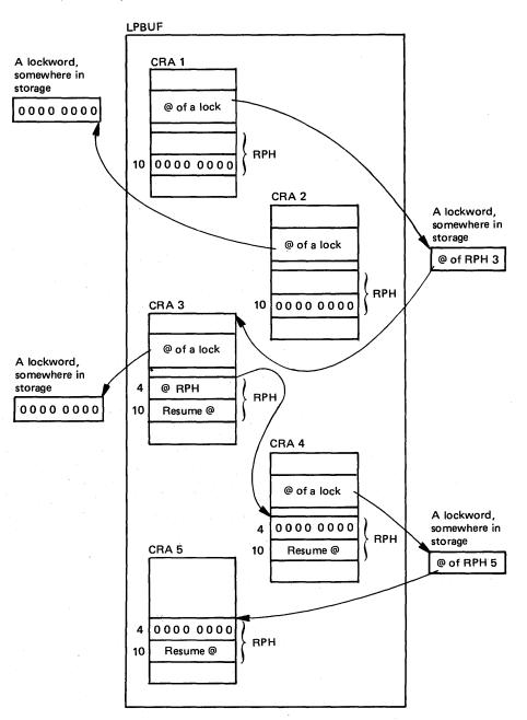
Non-waiting RPH (CRA 1) holds the lock that RPH 3 (CRA 3) and RPH 4 (CRA 4) are waiting for. Non-waiting RPH 2 (CRA 2) holds a lock no RPHs are waiting for. Waiting RPH 3 (CRA 3) holds a lock that no RPH is waiting for. Waiting RPH 4 (CRA 4) holds a lock that RPH 5 (CRA 5) is waiting for.
