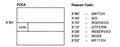
The code is set in the *receiving* processor's PCCA so that a bit on in processor B's PCCA, for example, means that processor A initiated the request.
