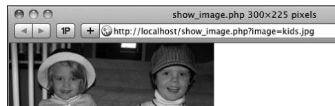
D The address of the pop-up window shows how the image value is passed in the URL.
