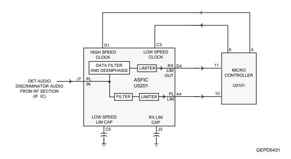
Figure 3-4 Receive Signalling Path.
