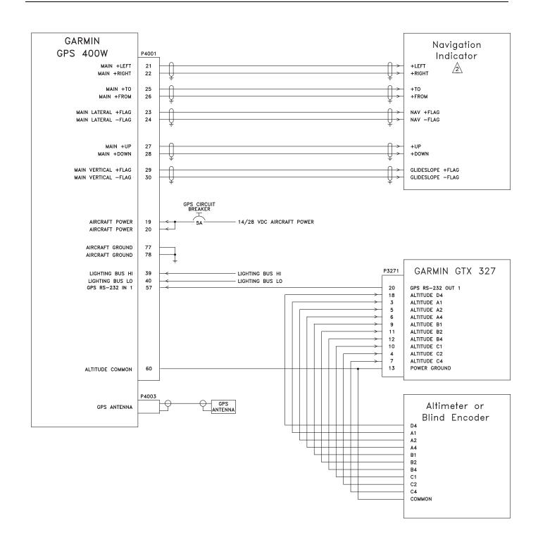
Figure H-4. GPS 400W Typical Installation Sheet 1 of 2
