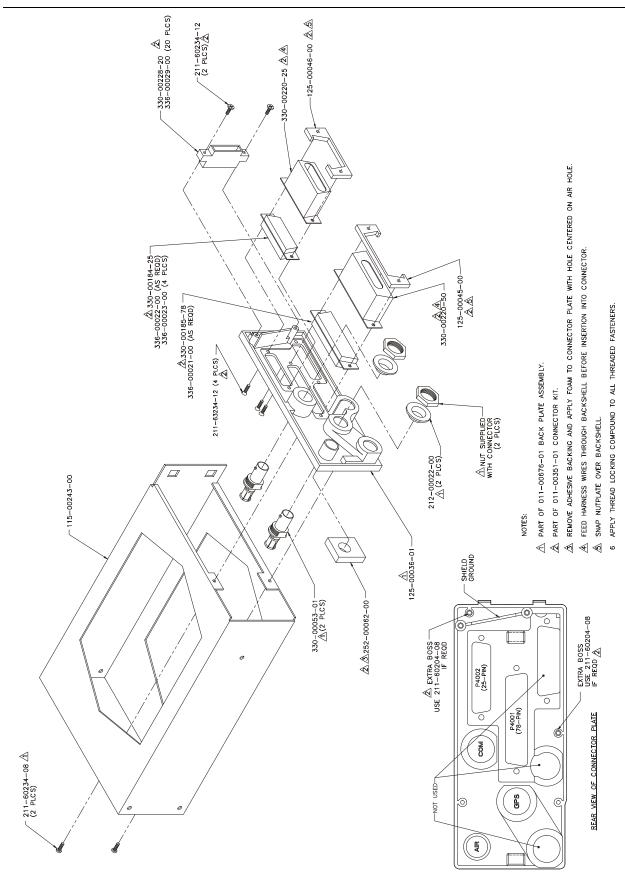
Figure F-3. GNC 420W Mounting Rack Installation
