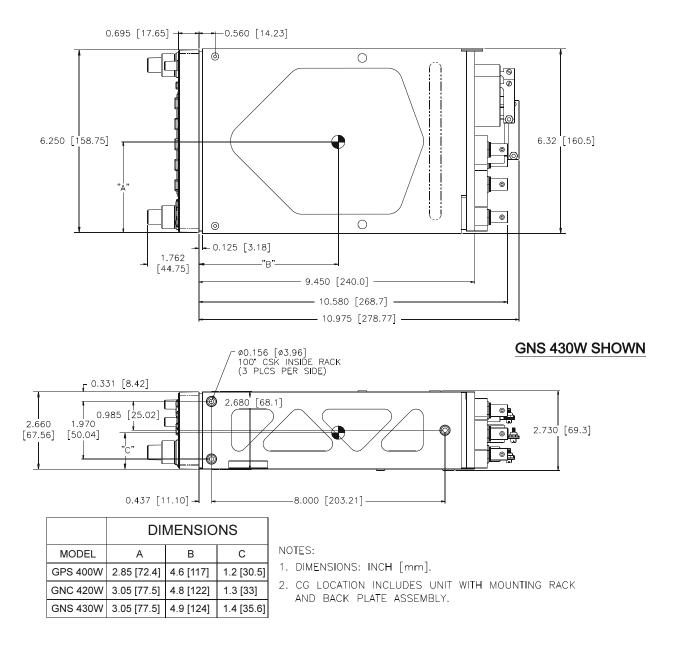
Figure F-1. 400W Series Mounting Rack Dimensions
