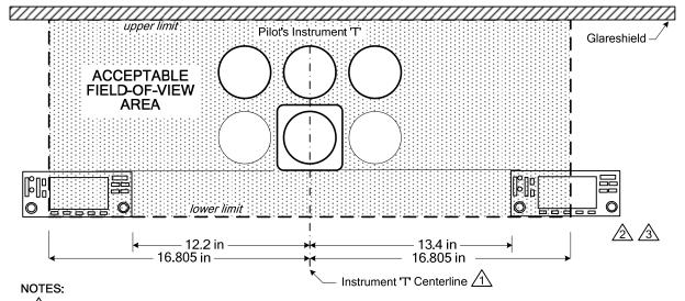
FOR AIRCRAFT WITHOUT THE BASIC INSTRUMENT 'T' CONFIGURATION, THE CENTER OF THE PILOT'S YOKE OR CONTROL STICK IN THE NEUTRAL POSITION SHOULD BE USED TO DETERMINE THE CENTERLINE. IF THE CONTROL YOKE/STICK IS OFFSET FROM THE CENTER OF THE PILOT'S SEAT, AN IMAGINARY LINE EXTENDED THROUGH THE CENTER OF THE PILOT'S SEAT MAY BE USED AS THE PRIMARY VIEW CENTERLINE.
