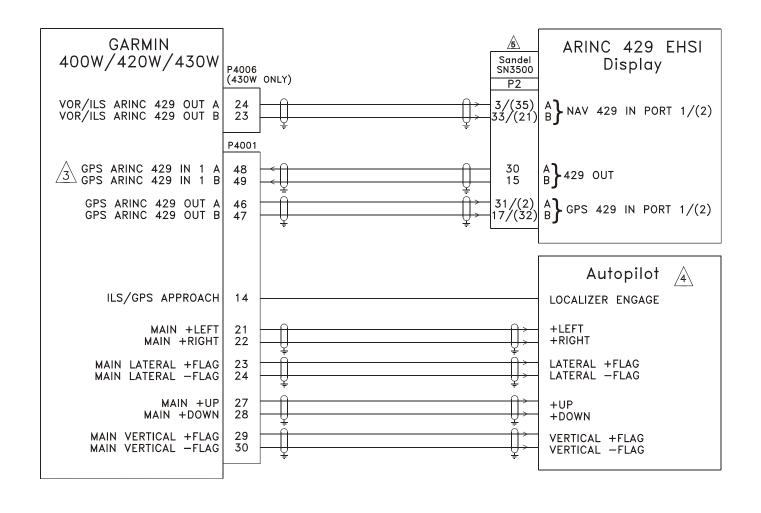
Figure H-28. ARINC 429 Sandel EHSI Interconnect (One 400W, One Sandel SN3500) Sheet 1 of 2
