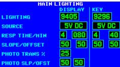
Figure 5-10. MAIN LIGHTING Page (Display Lighting from Lighting Bus)
