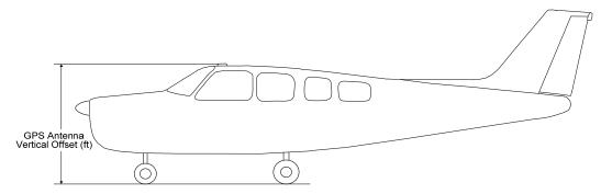
Figure 5-19. Measurement of GPS Vertical Offset
