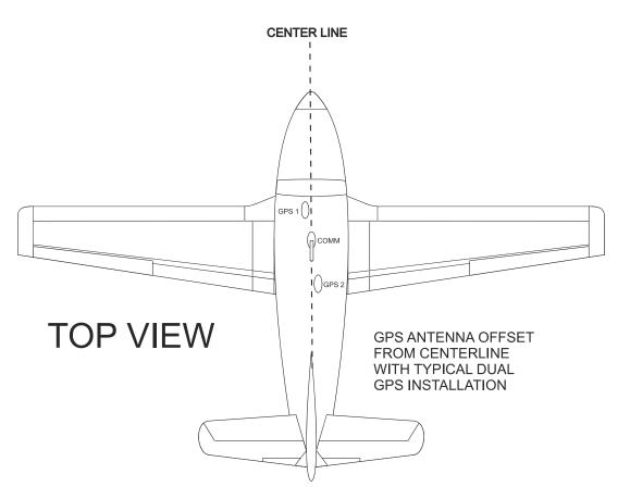
Figure 2-1. GPS Antenna Installation Considerations
