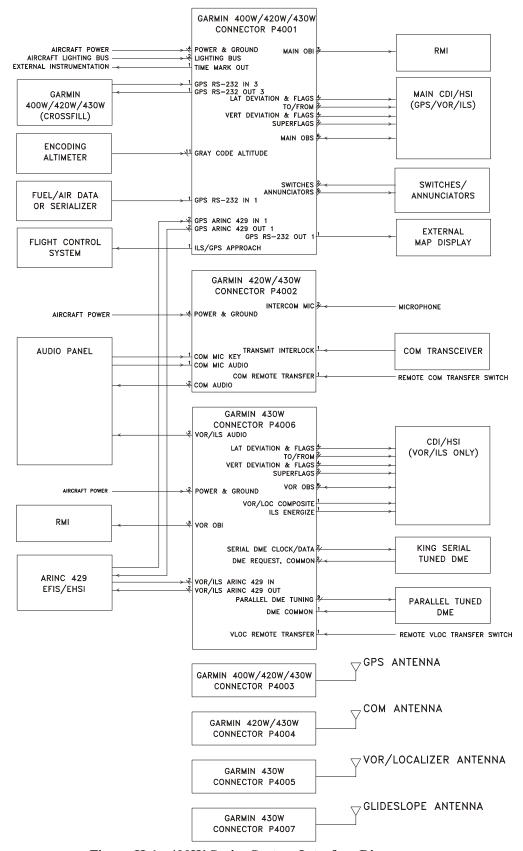
Figure H-1. 400W Series System Interface Diagram
