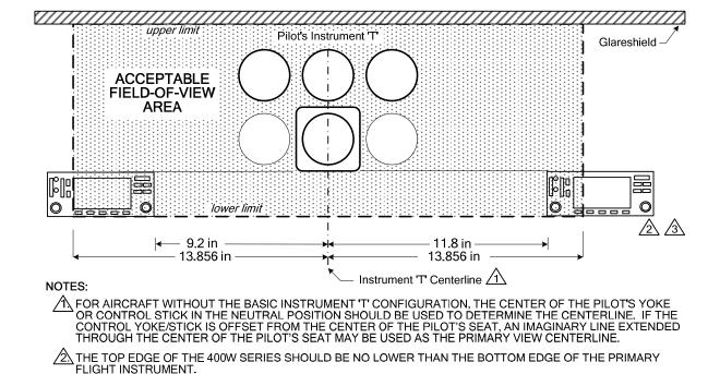
Figure 2-2. Source Selection Annunciation Field of View
