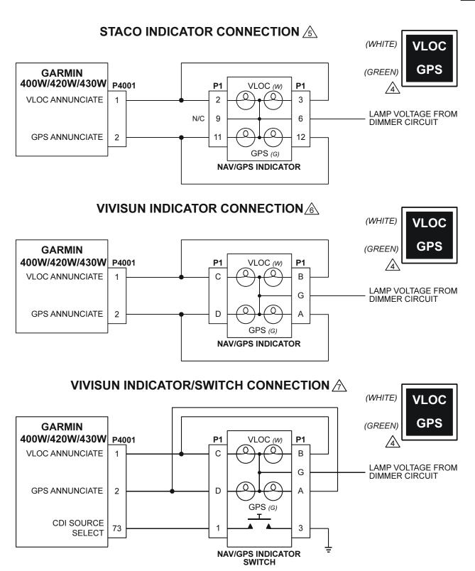
Figure H-29. External Navigation Source and GPS Annunciators Sheet 1 of 2
