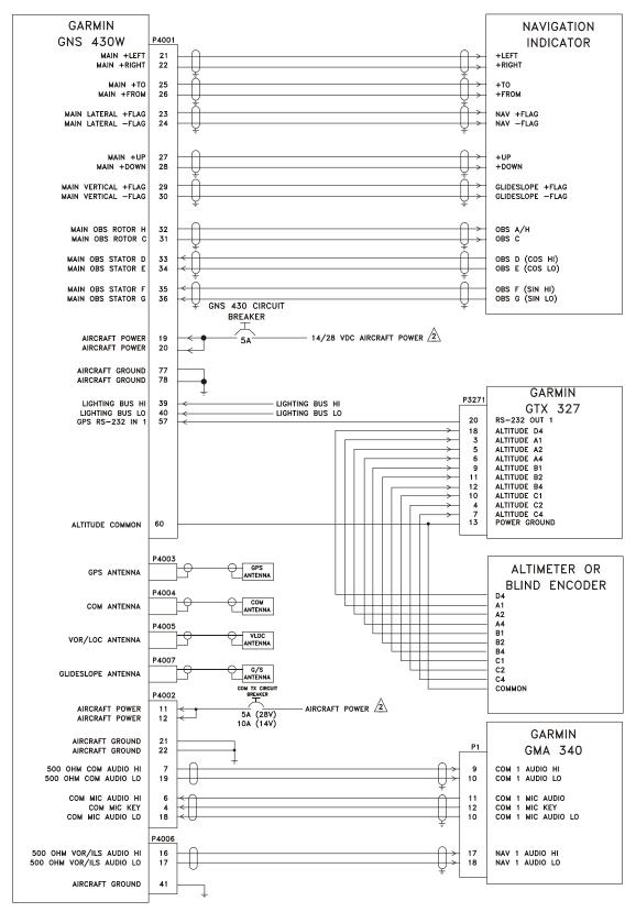
Figure H-2. GNS 430W Typical Installation Sheet 1 of 2
