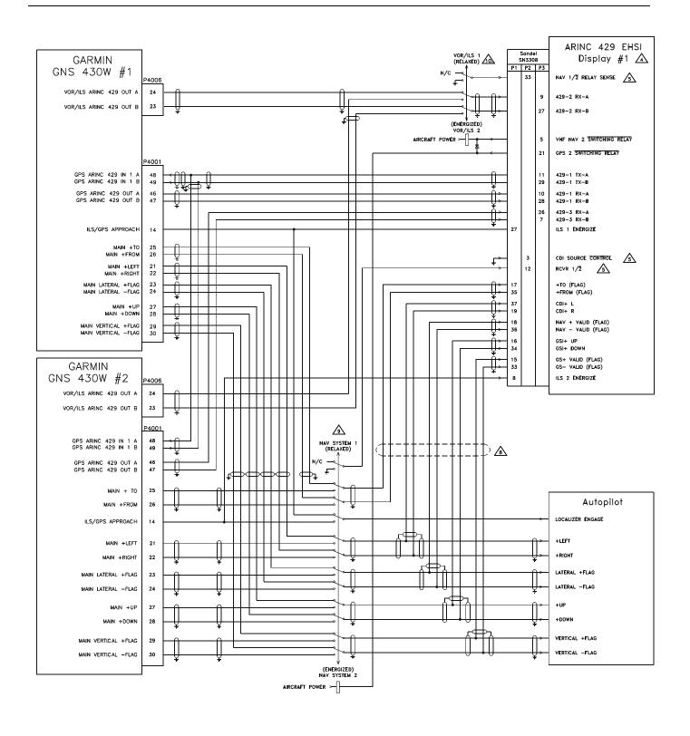
Figure H-13. ARINC 429 Sandel EHSI Interconnect (Two GNS 430W, One Sandel SN3308) Sheet 1 of 2
