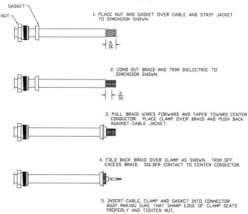
Figure 3-1. Coaxial Cable Installation
