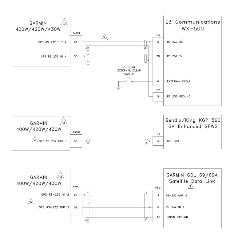
Figure H-18. Weather and Terrain Interconnect Sheet 1 of 2
