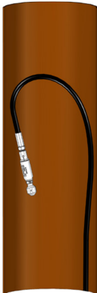
IMPROPER USE: Gopher will turn around in large diameter pipe VERY DANGEROUS!
