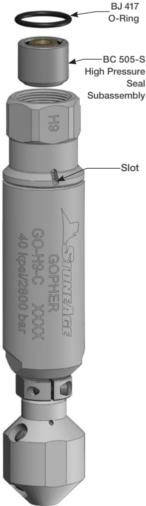
Figure 2: Remove BJ 417 O-Ring
