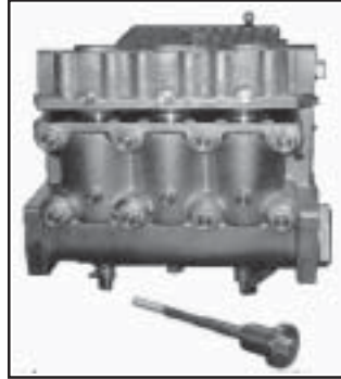
2) Remove discharge casing (50B) up and away.
