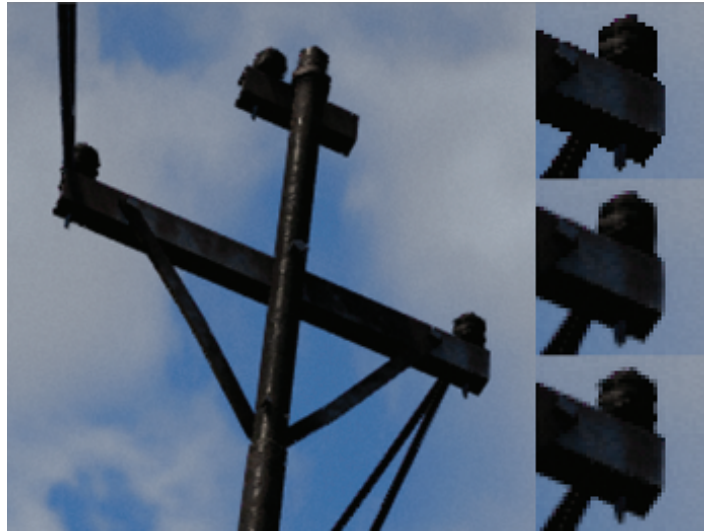
Figure 27.1. The crops on the right show no AA (top), SMAA (middle), and the presented HRAA (bottom) results. Only HRAA is capable of reconstructing additional details while providing high-quality antialiasing.
