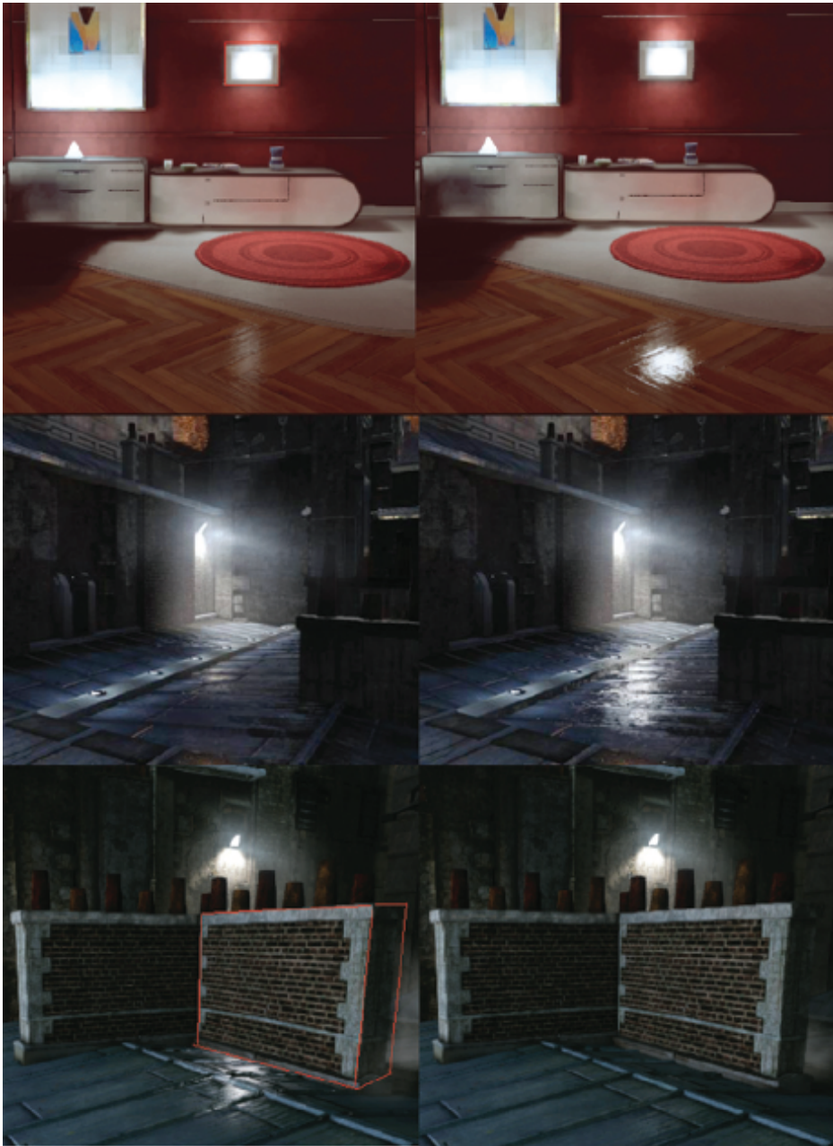
Figure 14.8. Examples of best practices. Top to bottom: cases 2, 3, and 4. On the left, the scene with only the cubemap reflection and the image proxy capture frustum (red box). on the right, the enhancement resulting from image proxy use.
