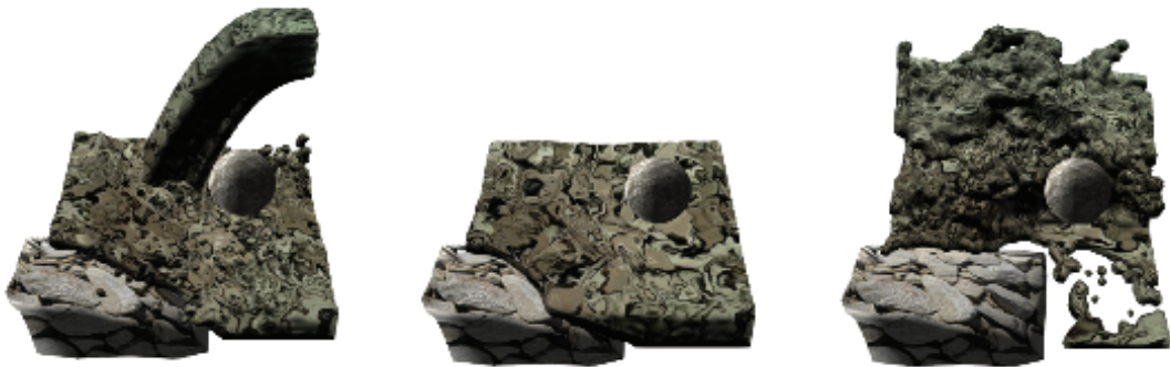
Figure 24.3. A 3D liquid simulation with obstacles in the domain implemented using the rasterization pipeline. The simulation runs at 35 FPS using 125k particles on a Quadro 2000M graphics card.
