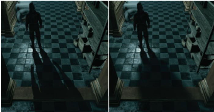
Figure 25.10. Shadow with ordinary filtering (left) and with contact-hardening shadows (right). [Image courtesy Square Enix Ltd.]
