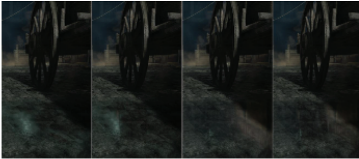
Figure 25.1. From left to right: cube map reflections only, SSR + cube maps, IBR + cube maps, and SSR + IBR + cube maps. [Image courtesy Square Enix Ltd.]
