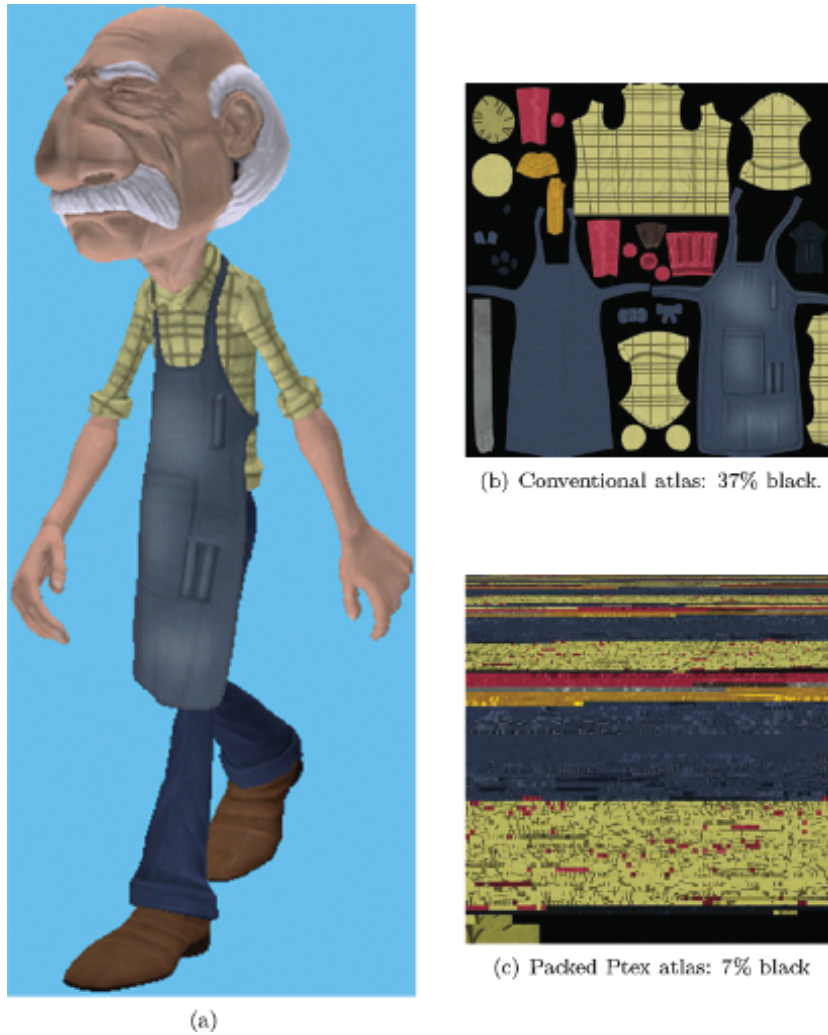
Figure 15.4. All textures for the model in (a) are in the packed Ptex format: Albedo, AO, specular, normal, and vector displacement: (b) an example of a conventional texture map and (c) an equivalent packed Ptex texture map.
