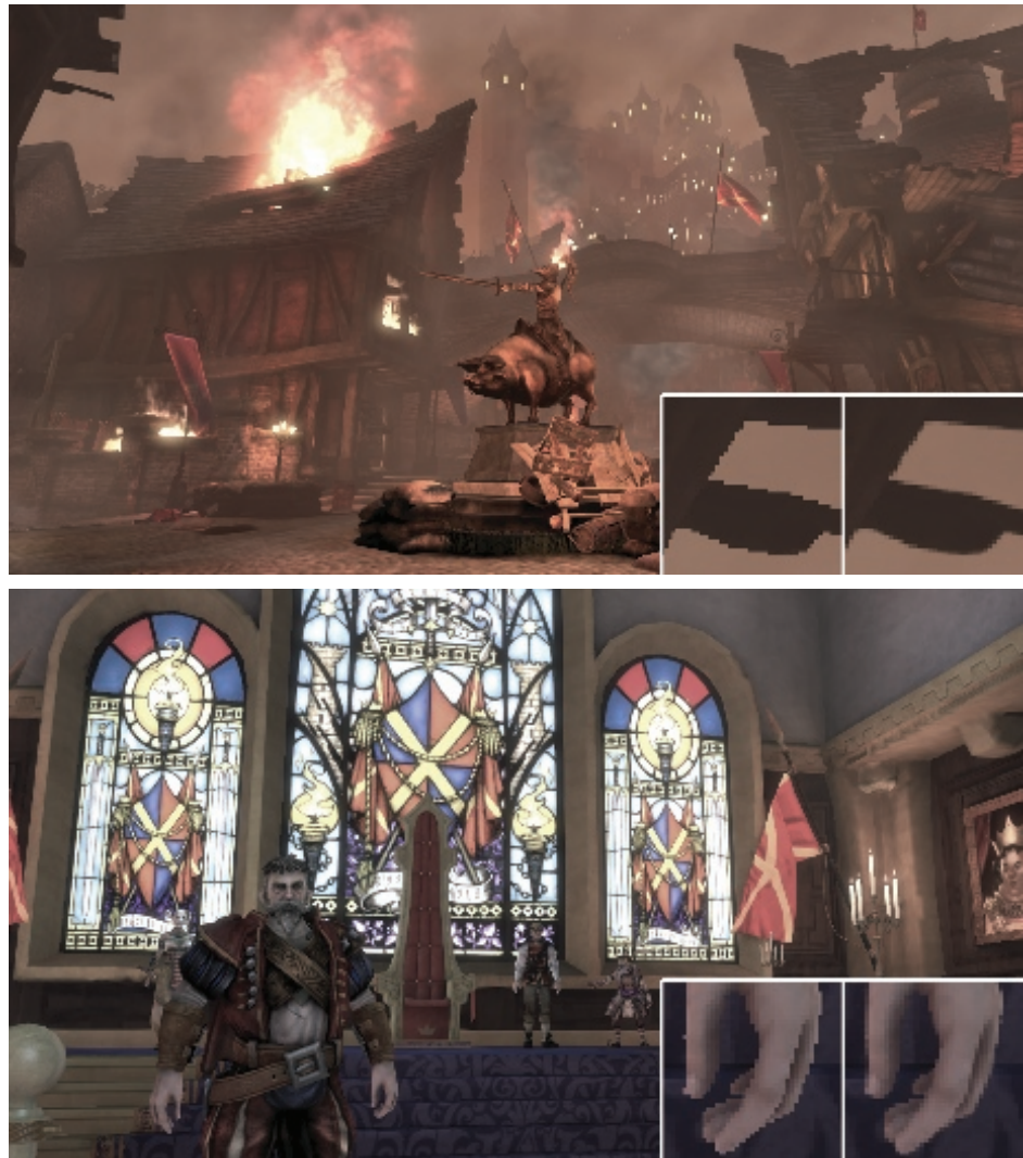
Figure 8.6. Images obtained with our algorithm. Insets show close-ups with no antialiasing at all (left) and processed with our technique (right). (Images from Fable III courtesy of Lionhead Studios.)
