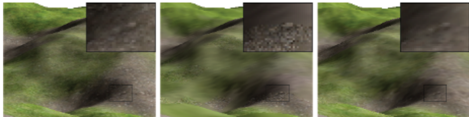
Figure 4.4. Half a second after the u-turn. Left: waiting for all tiles provides superior image quality but stalls for 330 ms. Middle: limiting the uploads per frame and using coarser MIP map levels as fallback provides smooth frame rates, but MIP levels vary strongly. Right: using prioritized loading of ancestors improves fallback, and image quality is much more balanced after the same time.
