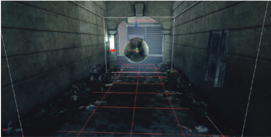
Figure 14.1. Cubemap with a box volume (white) and reflection plane (red) matching a rectangular room environment.
