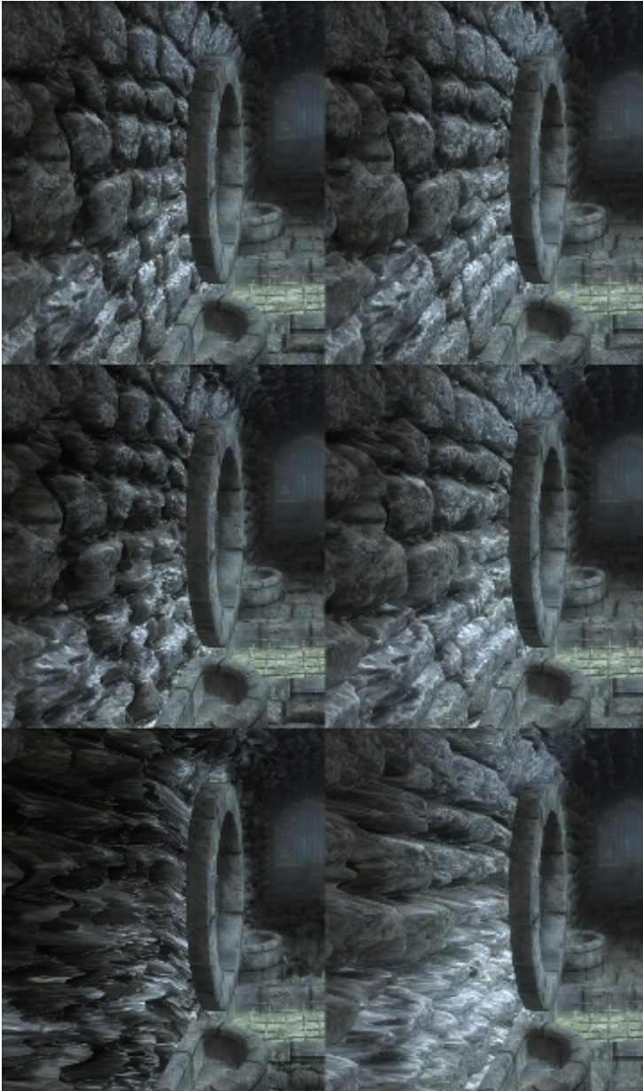
Figure 1.10. Quality comparison. Left POM. Right QDM. Depth Scale: 1.0, 1.5, 5.0. From depth scale 1.5 and above artifacts are visible while using POM.
