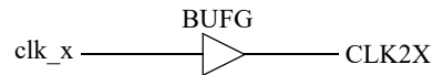
Figure 38. Spartan 3/e generation of CLK2X clock when VHDL generic clk2xen is zero
