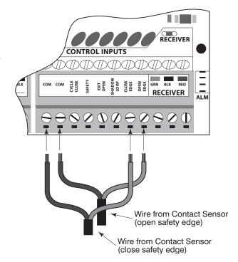
NOTE: If the close edge is contacted when the gate is opening, nothing happens. If the close edge is contacted when the gate is closing, then it reverses. If the open edge is contacted when the gate is closing, nothing happens. If the open edge is contacted when the gate is opening, then it reverses.
