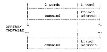
KEYTAB and KEYTABLE consist of threeword entries aligned on word boundaries. The first eight bytes are a left-adjusted character constant keyword. The third word is an unconditional branch to the keywordprocessing routine.
