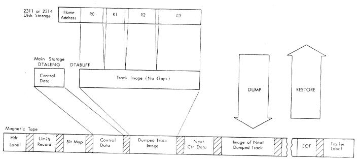
Figure 2. Dumping and Restoring a Direct-Access Track (SAM and VAM 1)
