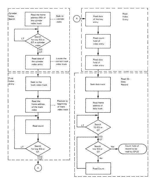
Figure 25. Scan Mode Channel Program 23
