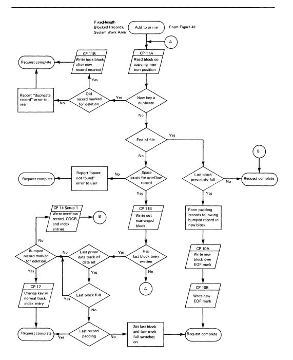
Figure 44. WRITE KN Channel Program Flow — Add to Prime (Fixed-Length Blocked Records, System Work Area)
