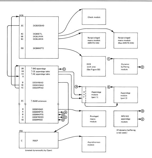
Figure 54. BISAM Control Blocks and Processing Modules
