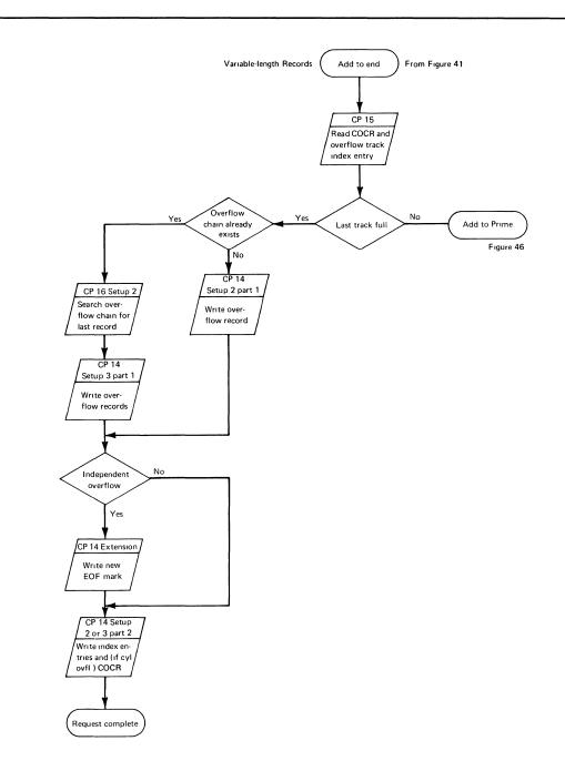
Figure 49. WRITE KN Channel Program Flow — Add to End (Variable- Length Records)
