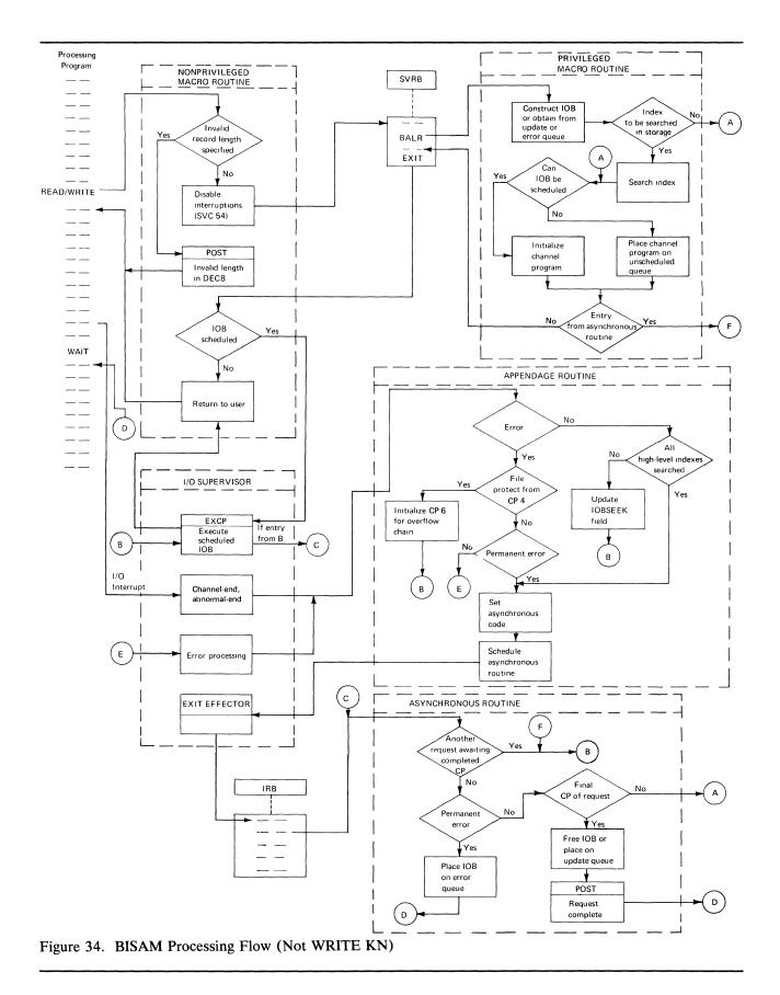
The check routine examines the DECB exception code (DECBEXCD) fields. If a permanent error has been posted, it searches the error queue for the corresponding IOB. The check routine then either gives control to the user's synchronous error (SYNAD) routine or, if the user has no SYNAD routine, issues SVC 55 (EOV) to request an ABEND with a code of 001.
