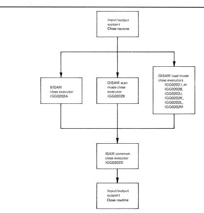
Figure 4. Flow of Control through the Close Executors
