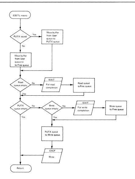
Figure 23. Scan Mode ESETL Routine
