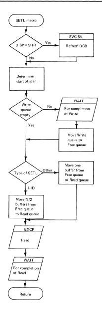
Figure 19. Scan Mode SETL Routine
