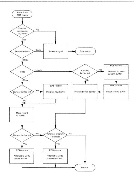
Figure 6. Load Mode Put Routine
