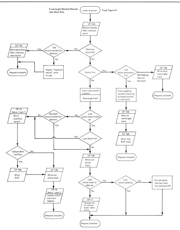
Figure 45. WRITE KN Channel Program Flow — Add to Prime (Fixed- Length Blocked Records, User Work Area)
