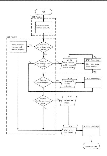
Figure 13. QISAM—Load Mode Channel Program Flow (Variable–Length Records)
