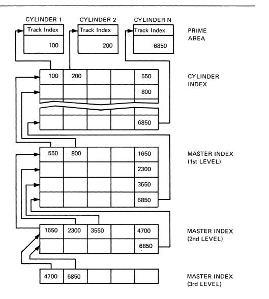
index. Each entry in the cylinder index identifies the key of the last record in the cylinder.
