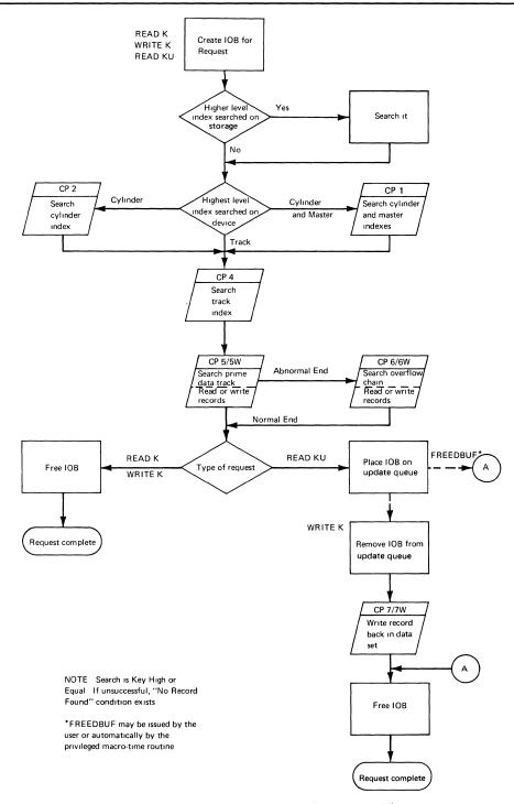
Figure 40. READ K, WRITE K, READ KU Channel Program Flow
