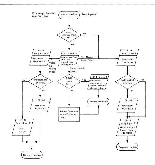
Figure 51. WRITE KN Channel Program Flow — Add to Overflow (Fixed-Length Records, User Work Area)
