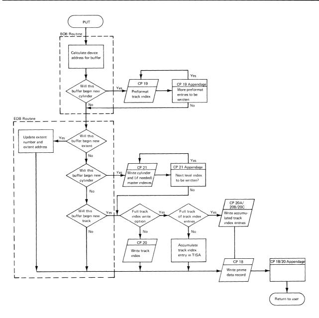
Figure 12. QISAM-Load Mode Channel Program Flow (Fixed-Length Records)
