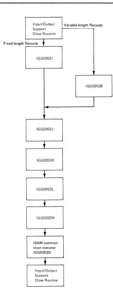
Figure 15. The Flow of Control through QISAM Load Mode Close Executors
