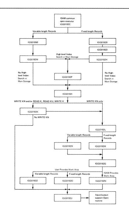
Figure 28. Flow of Control through BISAM Open Executors
