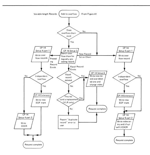
Figure 52. WRITE KN Channel Program Flow — Add to Overflow (Variable-Length Records)
