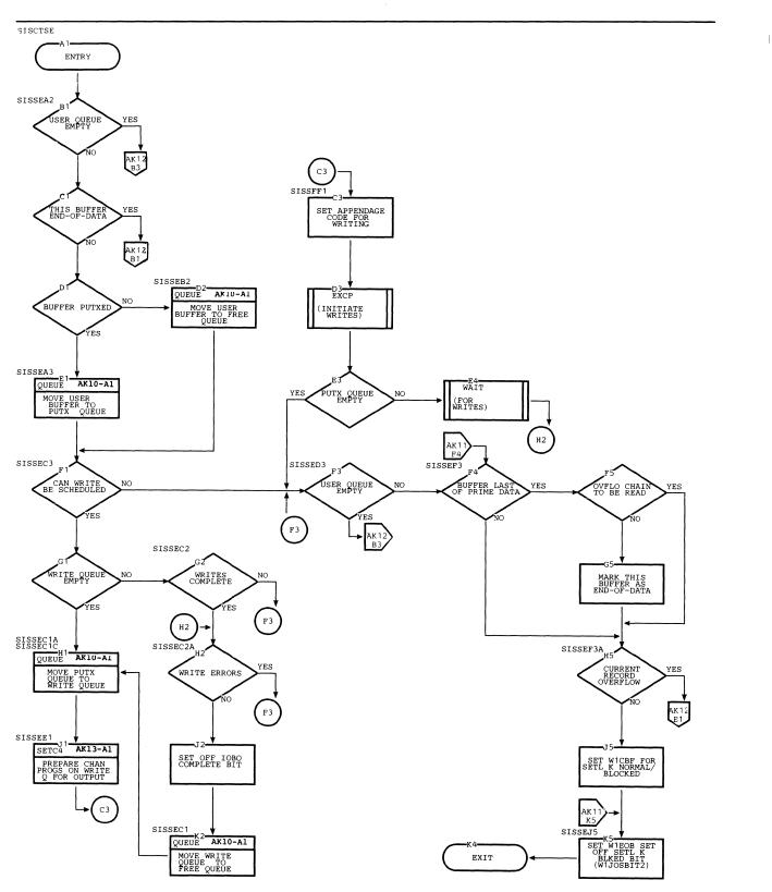
Chart AK11 QISAM Scan Processing Module (IGG019HB) End-of-Buffer Routine (Part 11 of 14)
