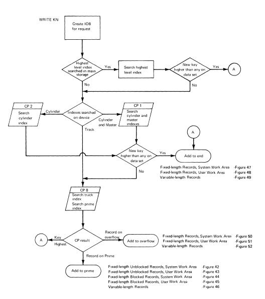
Figure 41. WRITE KN Channel Program Flow - Index Searching
