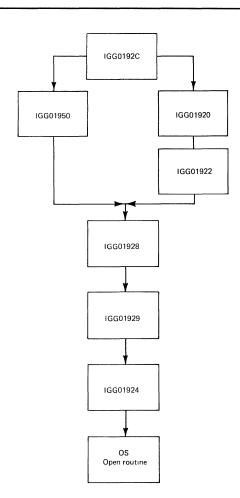
Figure 16. Flow of Control through Scan Mode Open Executors
