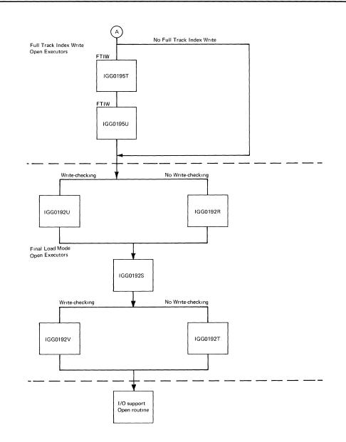
Figure 5 (Part 2 of 2). Flow of Control through Load Mode Open Executors
