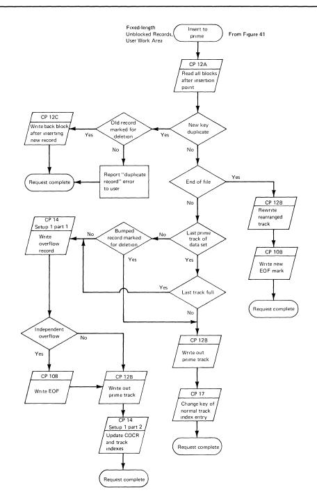
Figure 43. WRITE KN Channel Program Flow — Add to Prime (Fixed-Length Unblocked Records, User Work Area)
