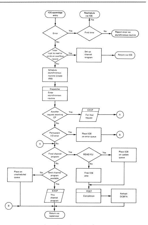
Figure 31. BISAM Appendage and Asynchronous Routines
