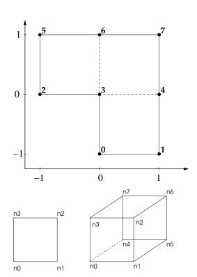
The file format is very simple: in the row, first the number of nodes in the coarse mesh is given, followed by the sum of mesh elements plus elements on the boundary. The last three values are always zero. This example has 8 nodes, 3 quads and 8 lines on the boundary.
