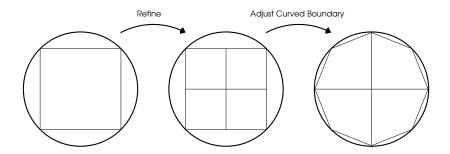
In Gascoigne boundary functions are described by the class BoundaryFunction<DIM> in File: GAS/src/Mesh/BoundaryFunction. The circle is given by:
