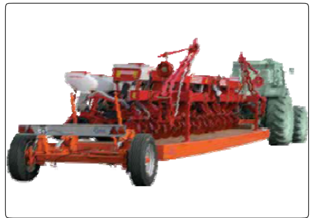
Road transport trailer with steering wheels
