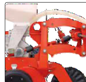
Planting unit drive with quick-release driveline-requires servicing less frequently
