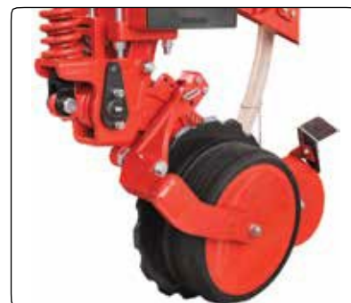
Planting unit with rubber depth gauge wheels
