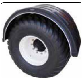
Low pressure wheels 700/50-22,5 (standard). Bumpers optional
