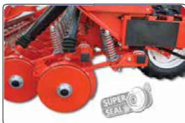
Double-disc coulters with compression spring
