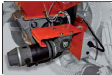
Electrical drive of doser GENIUS LITE
