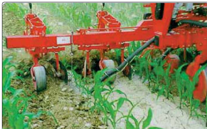
HEAVY DUTY CULTIVATOR UNIT - Frame with high ground clearance - Plate protection and excludible toothed side discs - Unit can be regulated with load spring (optional)
