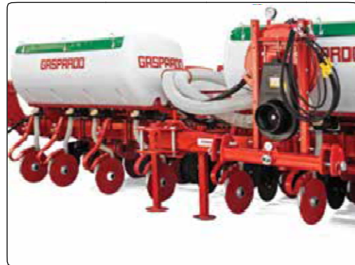
Folded drawbar for machine size reduction
