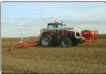
It seeds with no delays and waste. Pre-start and Pre-stop functions eliminate wastes due to delays of pneumatic systems during manoeuvring
