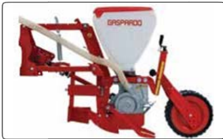
Seed boot coulters for thoroughly prepared soil.
