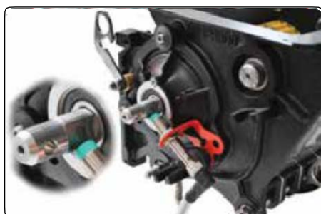
Dosing roller pin is inductive sensor ready (current standard)
