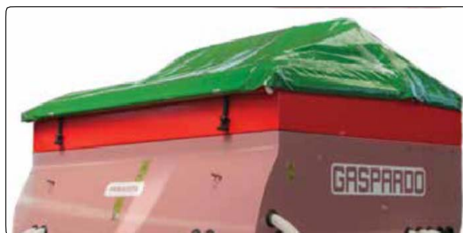
6 bu. hopper extension – optional, compliant with the 600 version only
