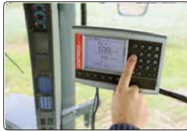
Easy dosing change from the tractor cab. The programmed dosage can be adjusted also while working through pre-set steps
