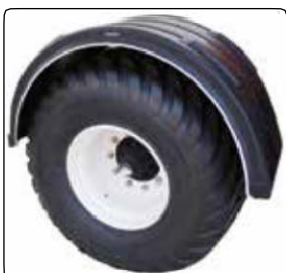
Low pressure wheels 700/50-22,5 (standard). Bumpers optional
