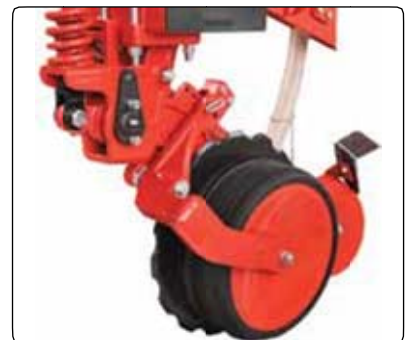
Planting unit with rubber depth gauge wheels
