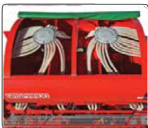
Hopper with four seed distributors
