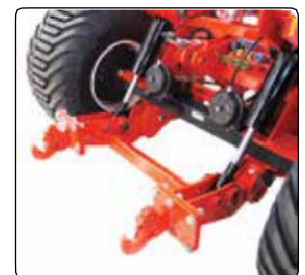
Hydraulic rear lifter with quick hitches, cat. 3 - 3N
