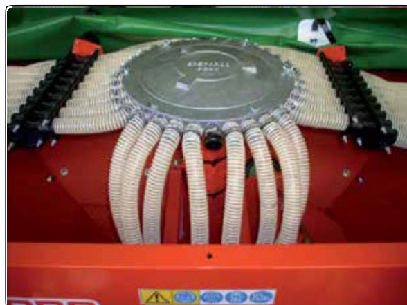
Electric seeding cut-off of lateral wings (optional)
