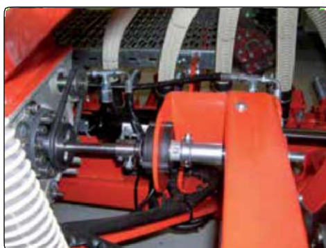
Electric seeding cut-off switch (optional)
