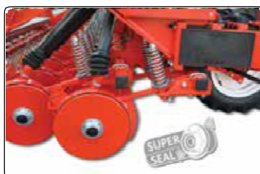
Double-disc coulter with compression spring
