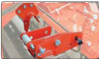
Hopper stands on the roller
