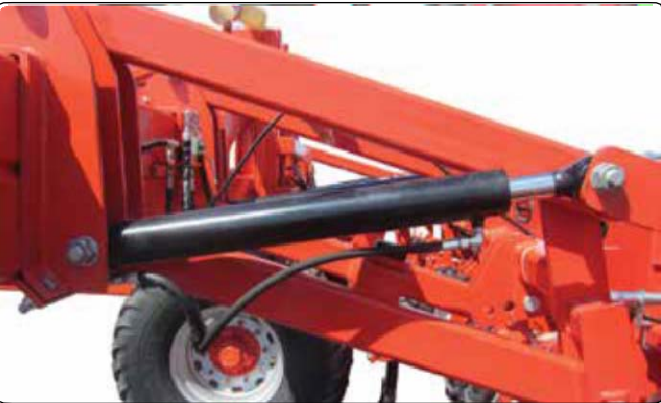
(METRO AIR) double effect cylinders on seeding hitches
