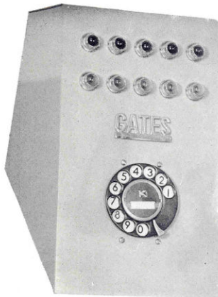
FIGURE A—Illustrates above the desk type dial circuit selector. This houses the dialing unit, circuit indicating lights and terminal connections which operate the stepping and control relays mounted on a separate rack panel. Its small size of 6 3/4 inches wide and 10 1/2 inches high makes it convenient for any type of desk mounting.
