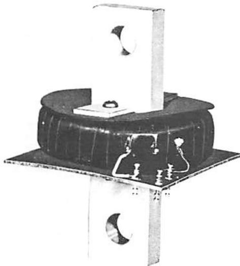
Fig. 21. Ground sensor coil with neutral mounting
