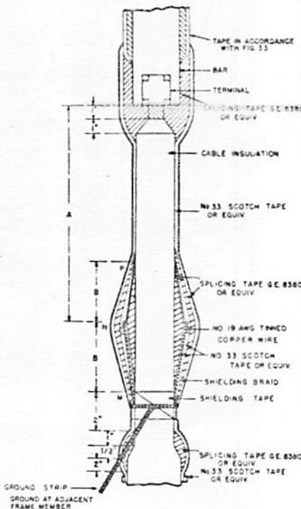
Fig. 37 Termination Non-Leaded Cable Single-Conductor
