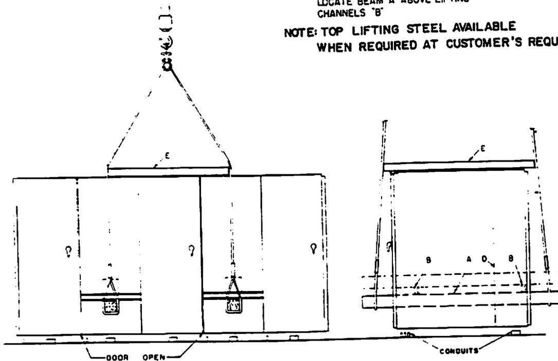
**ALTERNATE METHOD OF LIFTING**
