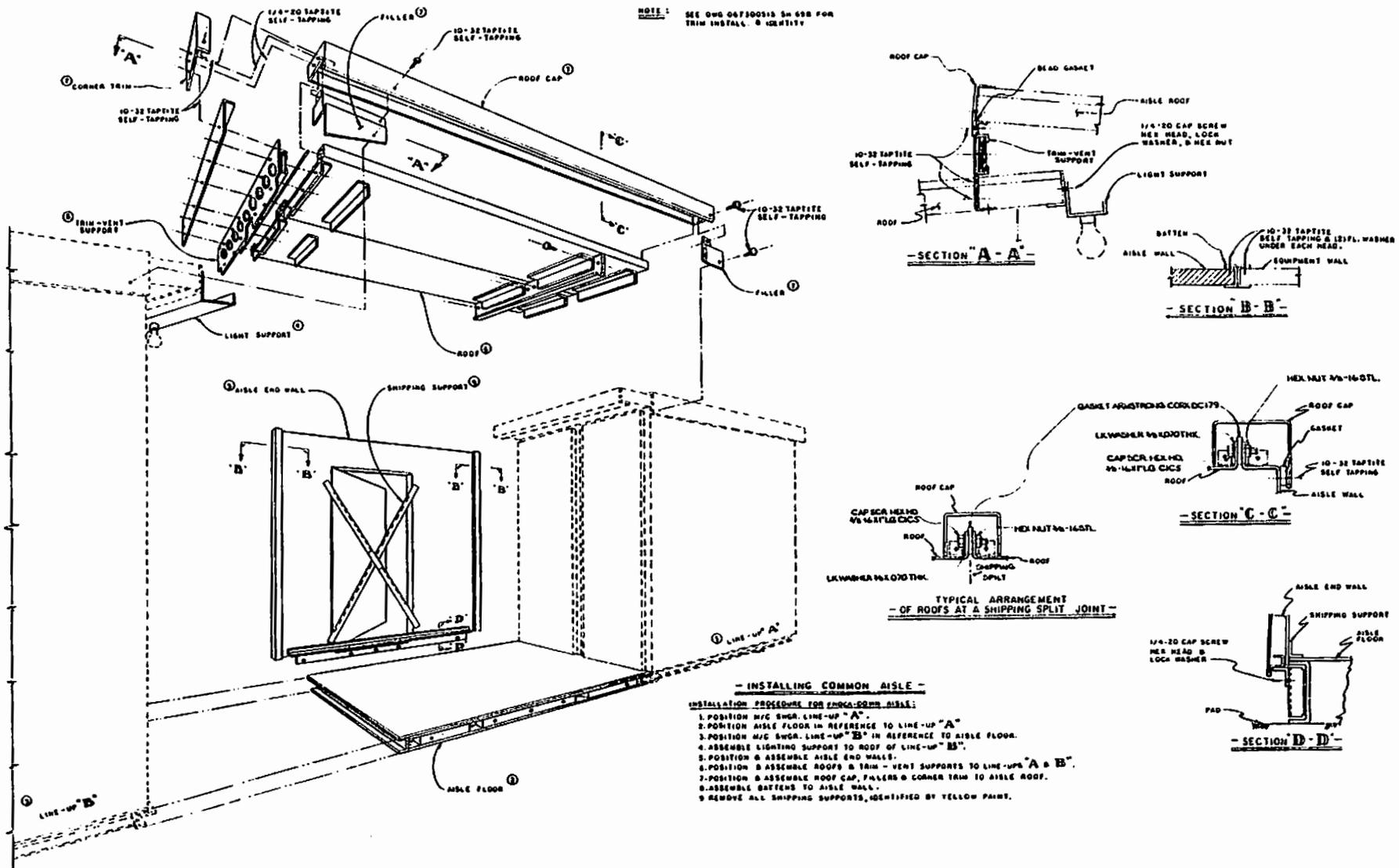
Figure 9. (0673D0515-019) Installation of Common Aisle
