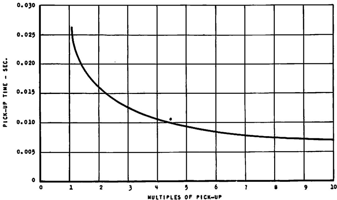
Fig. 7 Time-Current Characteristics of the Instantaneous Unit
