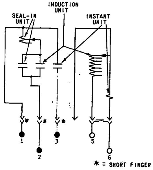
Fig. 13 Internal Connections For Type IAC53B Relay (Front View)
