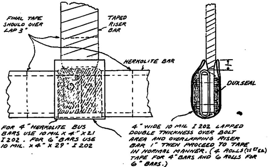
Fig. 26 13.8 KV Taped Joints
