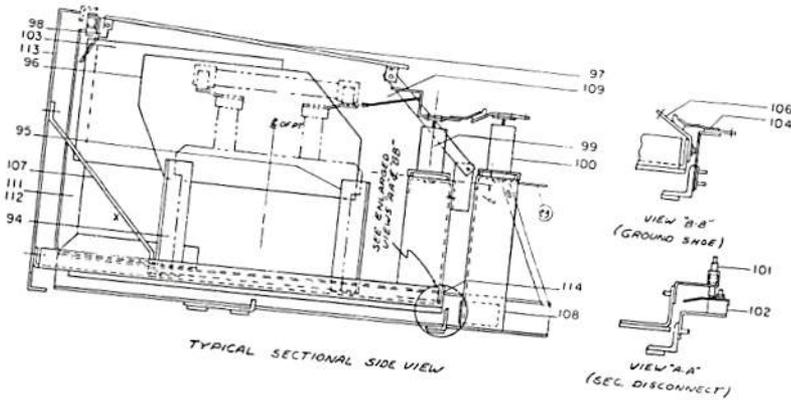
Fig. 56 Potential Transformer Rollout Unit
