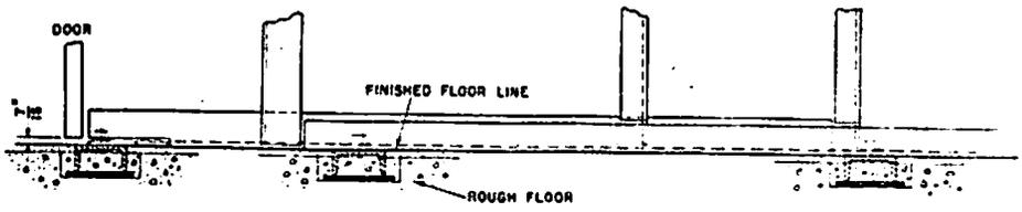
NOTE: IT IS IMPERATIVE THAT FLOOR STEEL BE EVEN WITH FINISHED FLOOR AND THAT BOTH BE LEVEL
