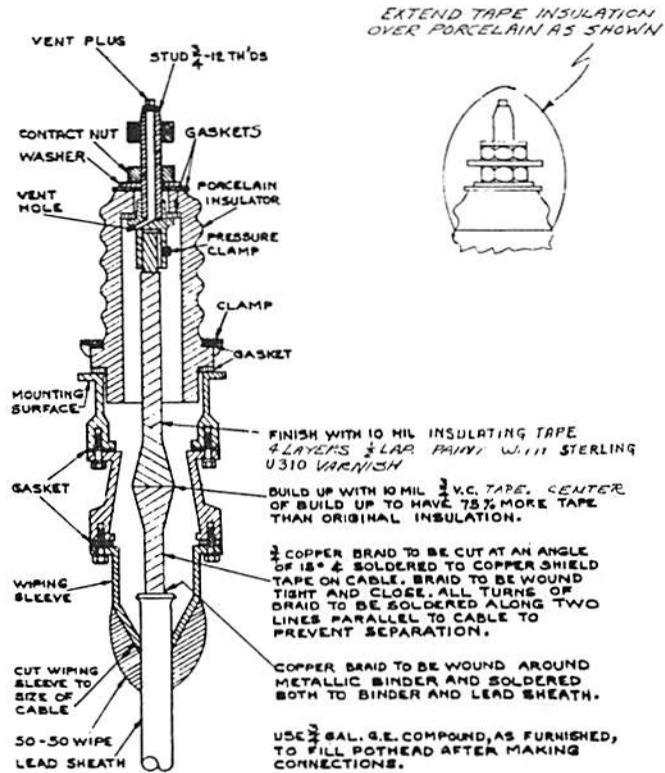
Fig. 40 Single-Conductor Pothead with Stress Cone
