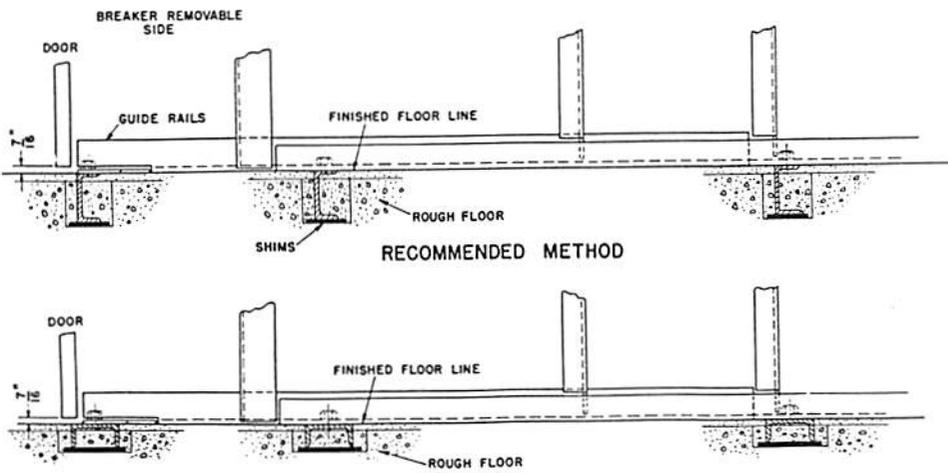
NOTE: IT IS IMPERATIVE THAT FLOOR STEEL BE EVEN WITH FINISHED FLOOR AND THAT BOTH BE LEVEL
