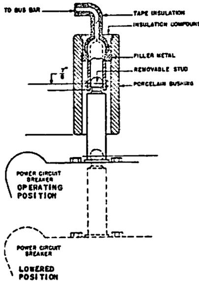
Fig. 9 Measurement of Adjustment of Primary Disconnecting Devices
