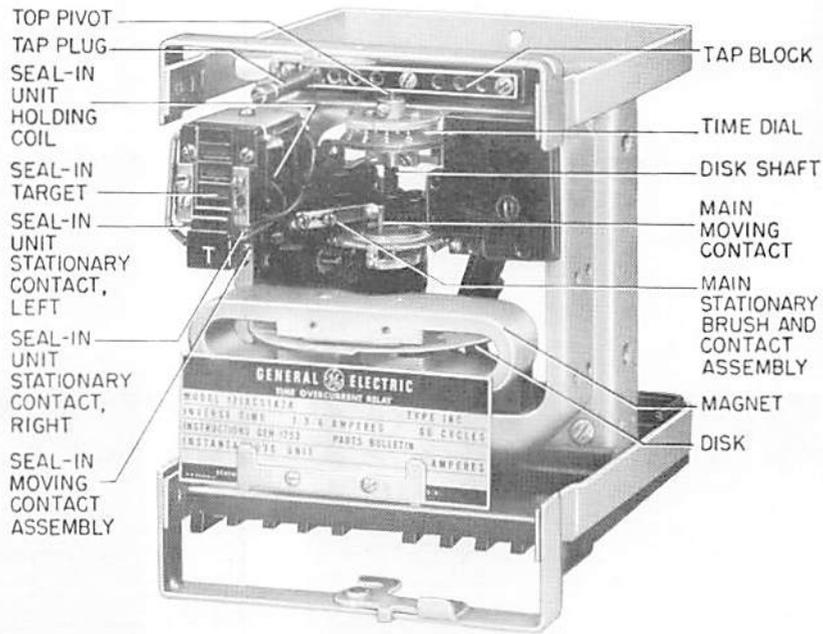
Fig. 1 The Induction Unit for Type IAC Relays (Front View)
