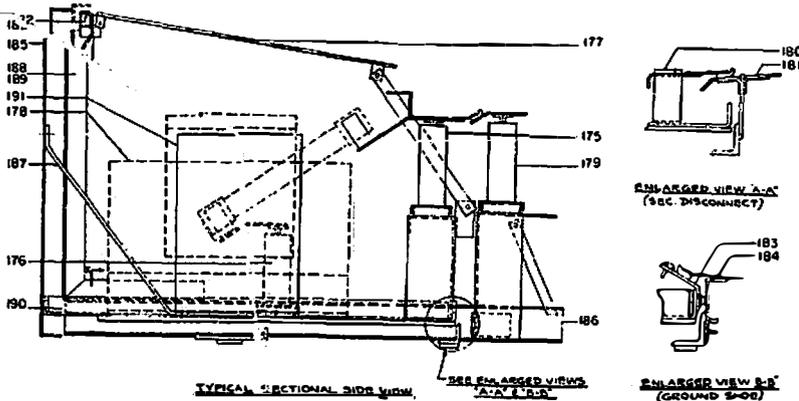
Fig. 57 Control Transformer Rollout Unit
