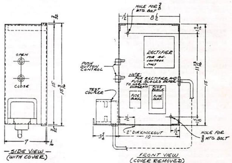
Fig. 22 Inspection Box for 13.8 KV Metal-Clad Switchgear
