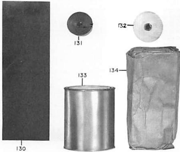
**Fig. 18 Taping material for bus connection joints**
