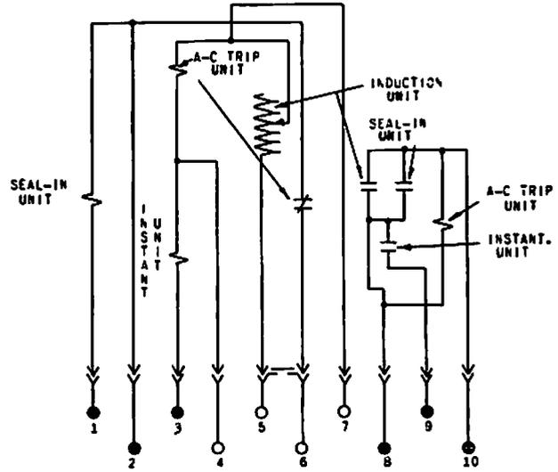
Fig. 15 Internal Connections For Type IAC53K Relay (Front View)
