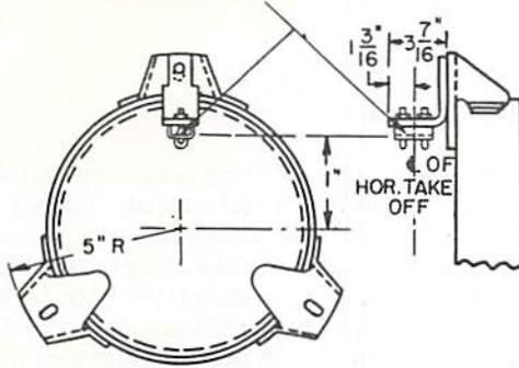
DETAIL OF LINE TERMINAL BRACKET FOR ARRESTERS 73 KV AND BELOW
