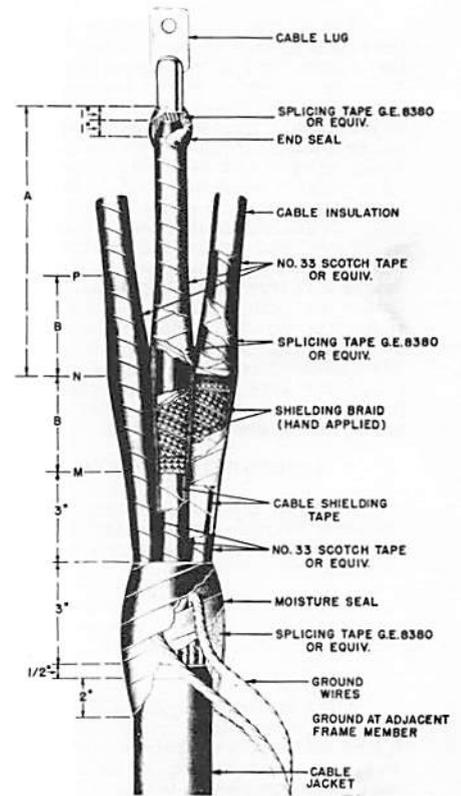
Fig. 44 Termination Without Pothead Multi-Conductor
