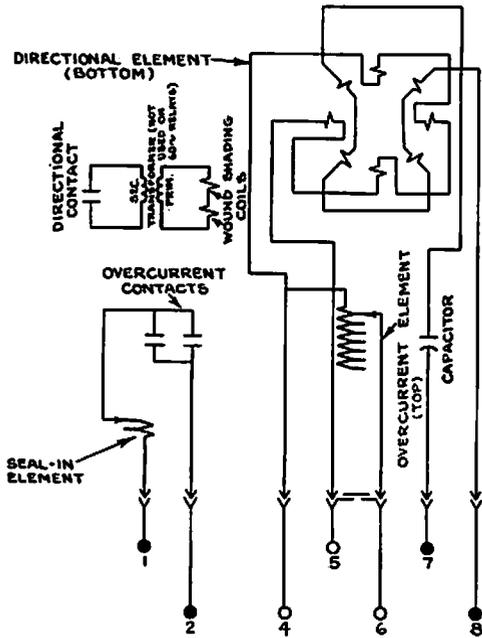
Fig. 14 Internal Connections For Type IAC53C Relay (Front View)
