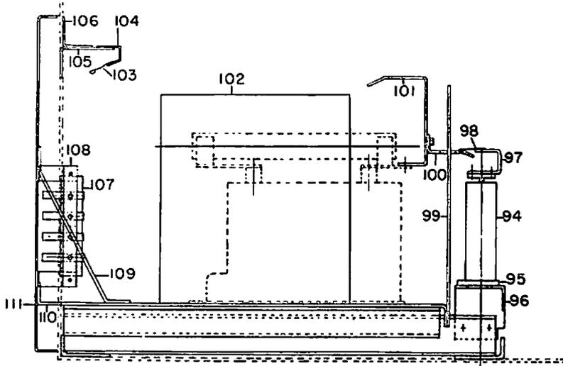
Fig. 41 Potential Transformer Rollout Unit
