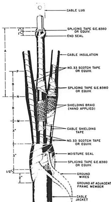
Fig. 44 Termination Without Pothead Multi-Conductor
