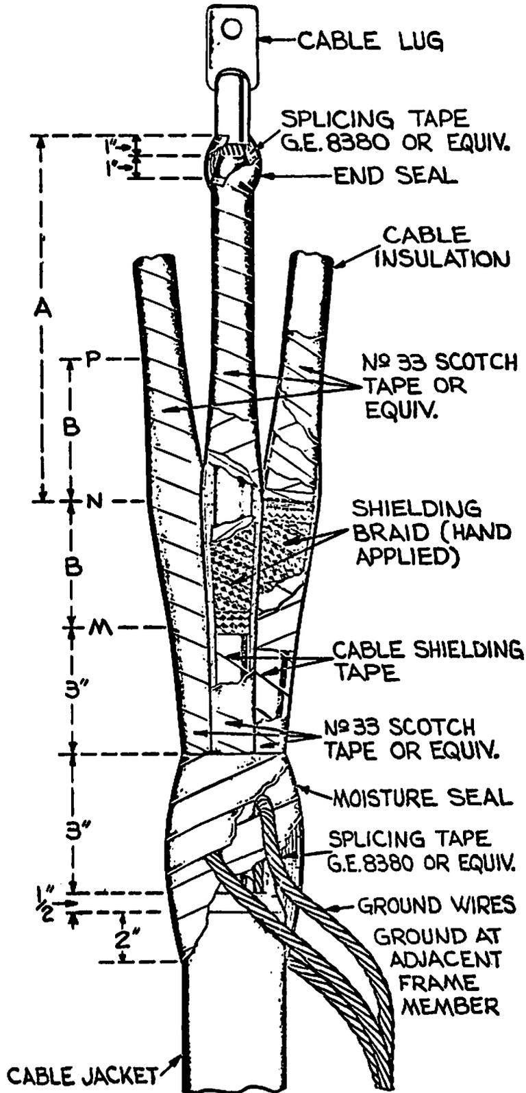
Fig. 29 (B232004C) Termination Without Pothead Multi-Conductor
