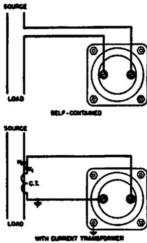
Fig. 5. External connections of a-c ammeter
