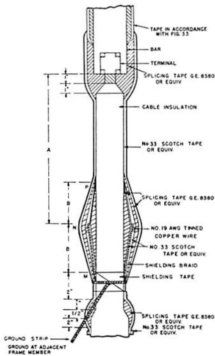
Fig. 43 Termination Without Pothead Single-Conductor
