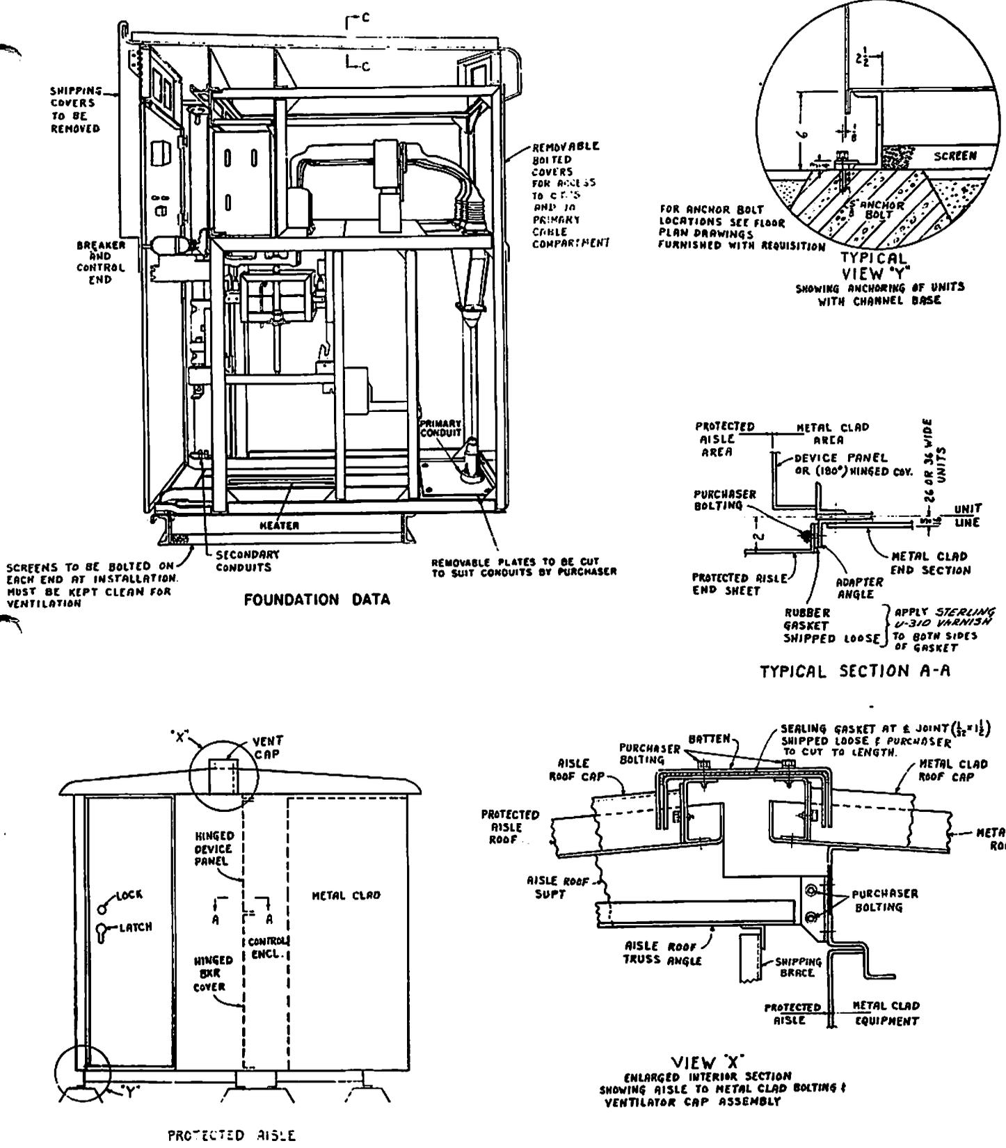
Fig. 9 Installation Details for Outdoor Metal-clad Switchgear with Protected Aisle
