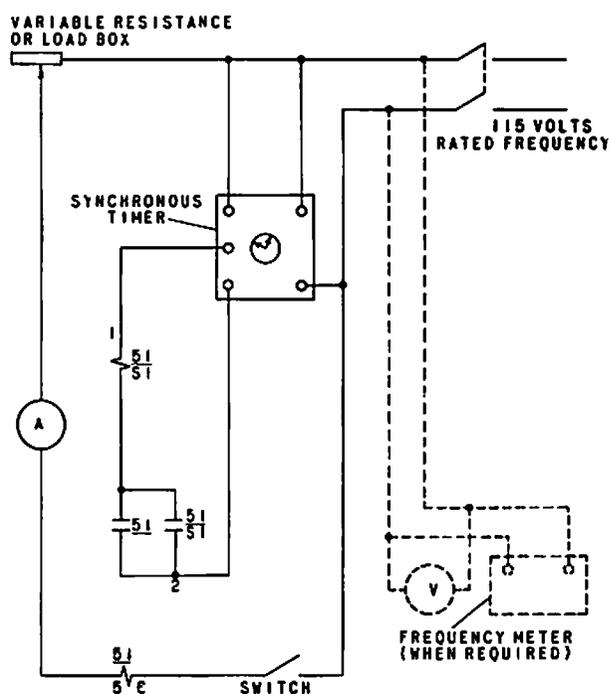
Fig. 19 Test Connections for Type IAC Relays such as Type IAC53A
