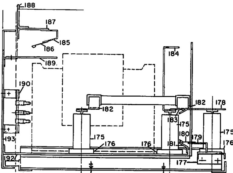
Fig. 42 Control Power Transformer Rollout Unit
