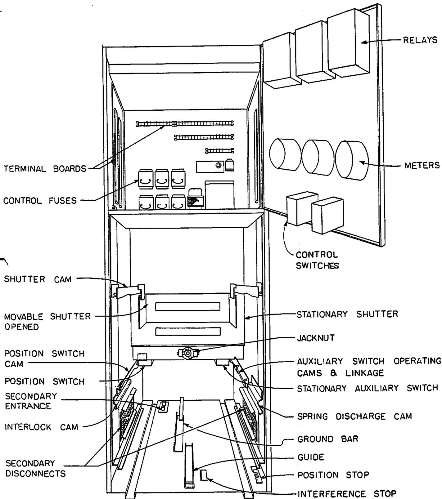
Figure 5. (0673D0515-183) Breaker Compartment 4.76 KV
