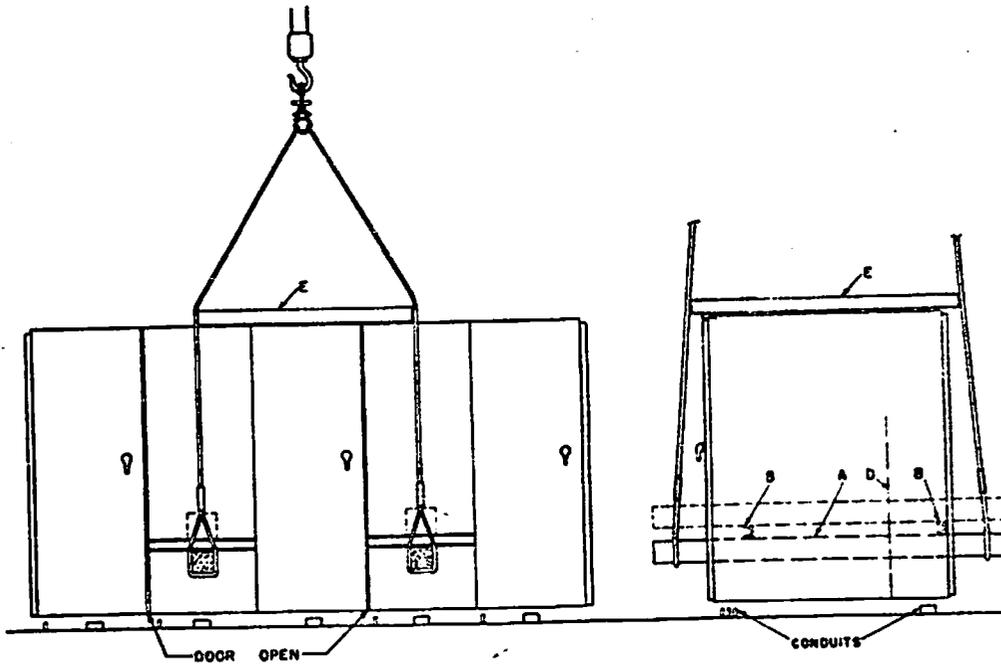
**ALTERNATE METHOD OF LIFTING**
