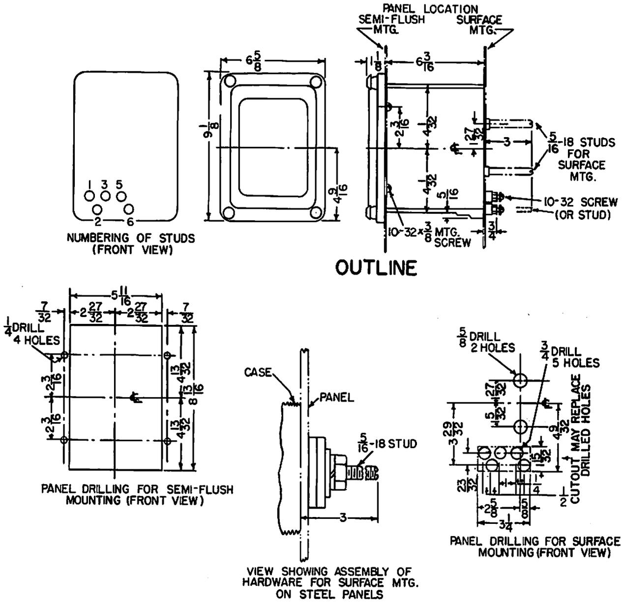
Fig. 20 Outline and Panel Drilling Dimensions for Relay Types IAC53A, IAC53B, IAC53C and IAC54A
