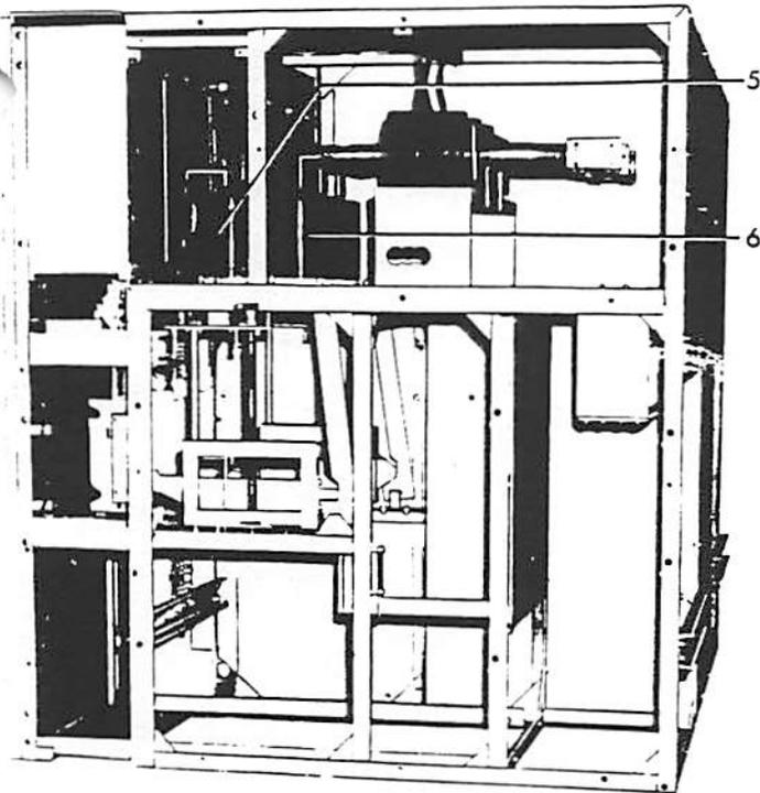
FIG. 10 (8039690) METAL-CLAD SWITCHGEAR
