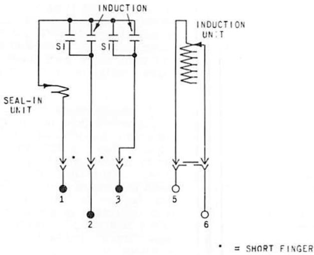
Fig. 16 Internal Connections for Type IAC54A
