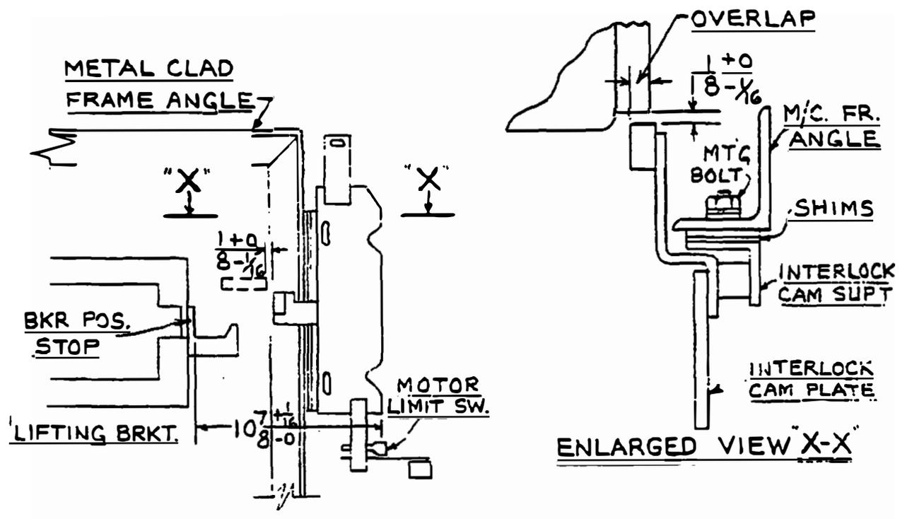
FIG. 29A (208A8952) POSITIVE INTERLOCK ADJUSTMENT
