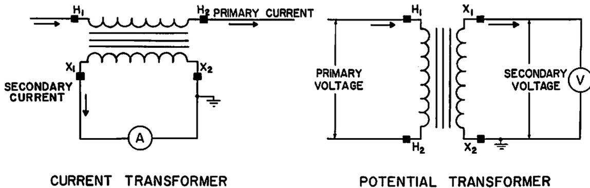
Fig. 1. Elementary Connections of Instrument Transformers
