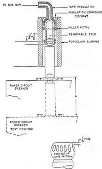
Fig. 11 Measurement of Adjustment for Primary Disconnecting Devices
