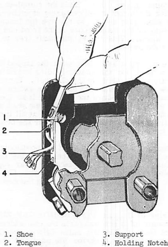
Fig. 8 Installing New Contact Finger
