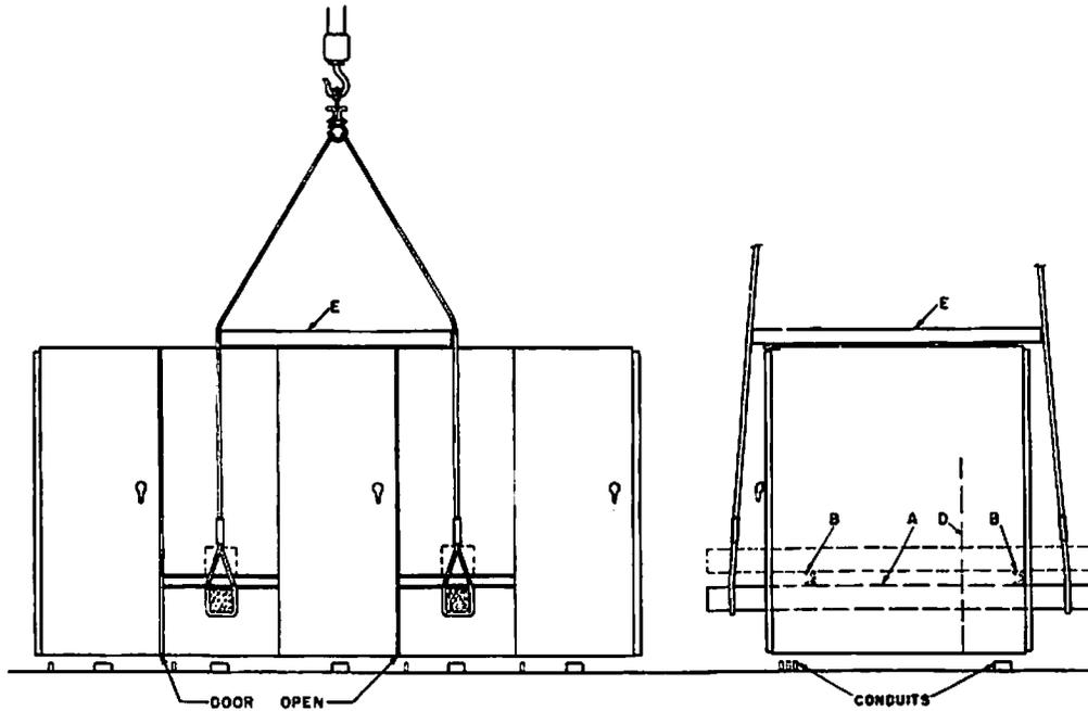
**ALTERNATE METHOD OF LIFTING**
