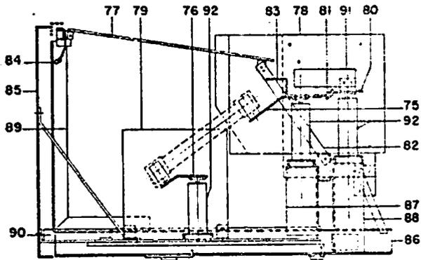
Fig. 49 Fuse Rollout Unit
