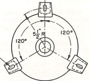
PLAN VIEW OF BOTTOM UNIT FITTING 121 KV ARRESTER
