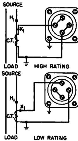
Fig. 6. External connections of double-rated a-c ammeter
