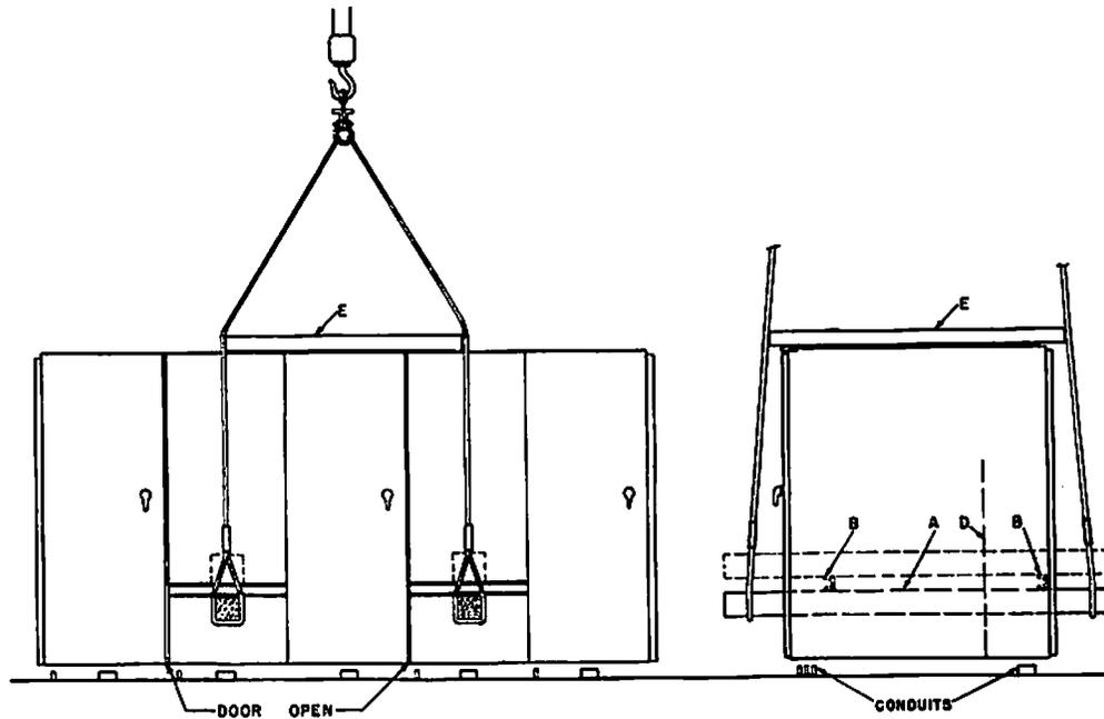
**ALTERNATE METHOD OF LIFTING**
