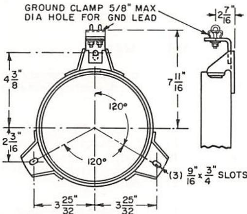
DETAIL OF ARRESTER BOTTOM FITTING AND GROUND TERMINAL FOR ARRESTERS 20-109 KV
