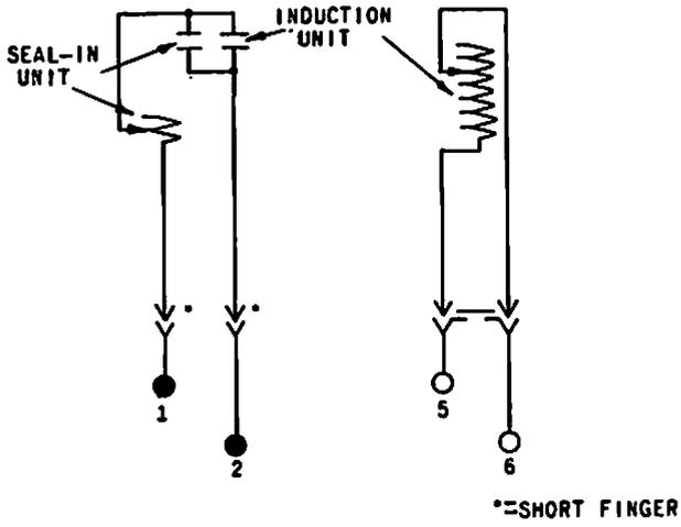
Fig. 12 Internal Connections For Type IAC53A Relay (Front View)
