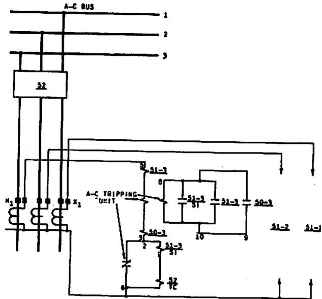
**Fig. 10 External Connections Of Three Type IAC53R Relays Used For 3-Phase Circuit Protection**
