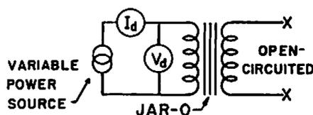
Fig. 2. Schematic diagram for demagnetizing JAR-O transformers
