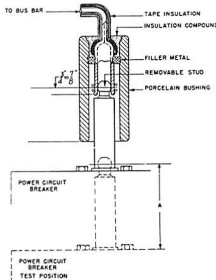
Fig. 11 Measurement of Adjustment of Primary Disconnecting Devices
