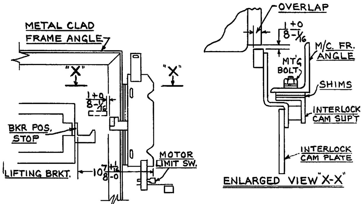
Fig. 29A (208A8952) Positive Interlock Adjustment
