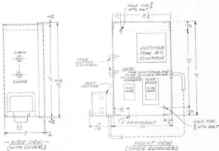
Fig. 23 Inspection Box for 13.8 KV Metal-clad Switchgear
