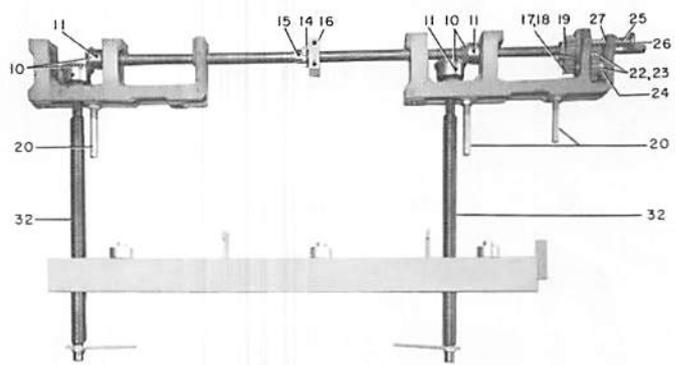
Fig. 5 Elevating mechanism for M-36HH equipments rated 1000 mva
