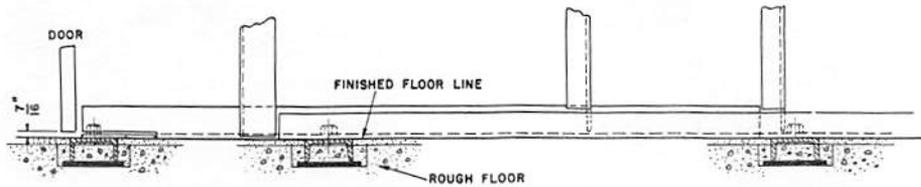
NOTE: IT IS IMPERATIVE THAT FLOOR STEEL BE EVEN WITH FINISHED FLOOR AND THAT BOTH BE LEVEL
