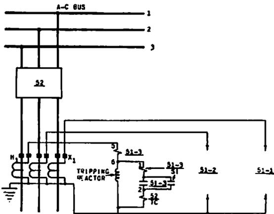
**Fig. 9 External Connections Of Three Type IAC53A Relays Used In Conjunction With Tripping Reactors For Protection Of A 3-Phase Circuit**
