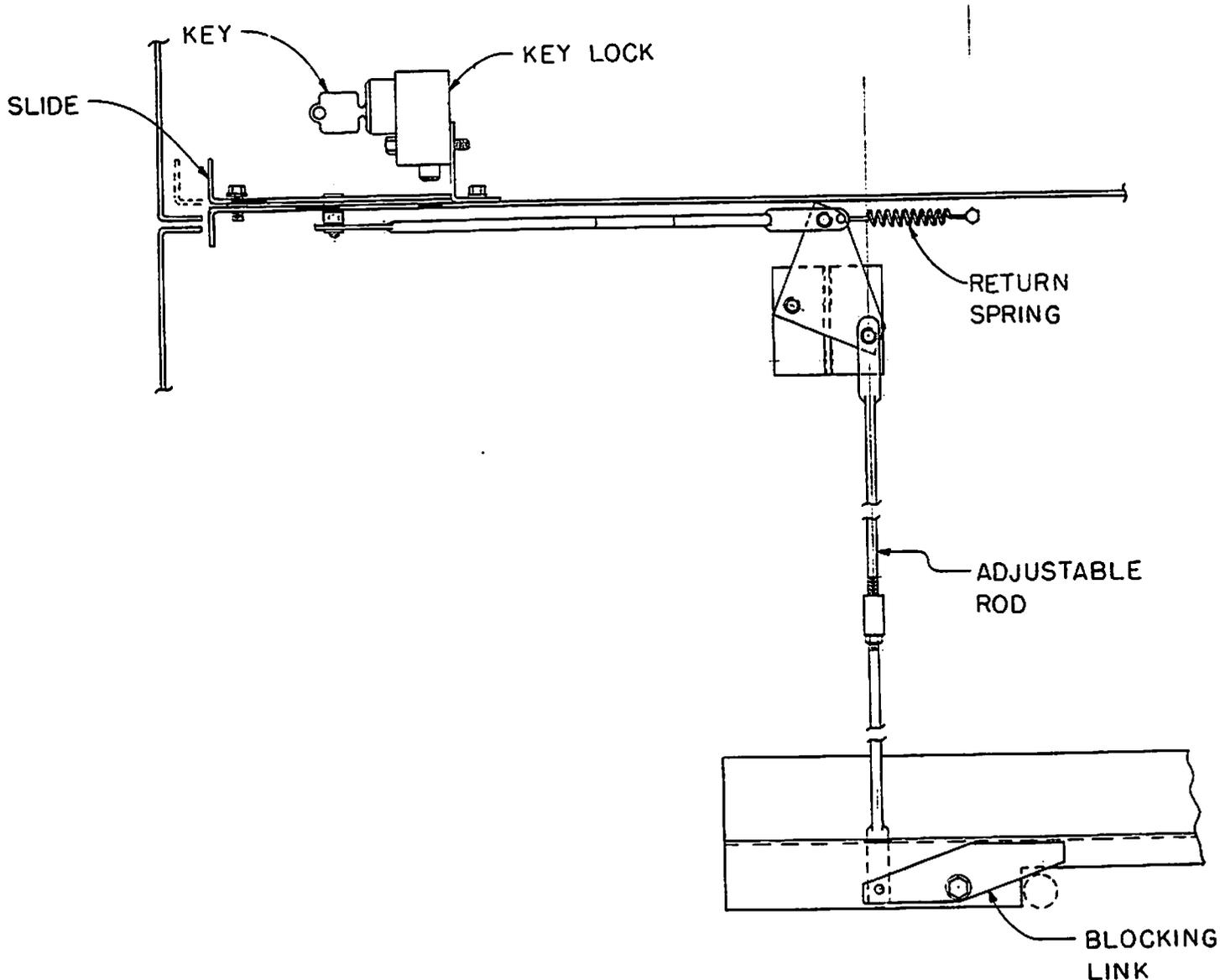
Figure 10 (0673D0515-182) Breaker Key Lock 4.76 KV
