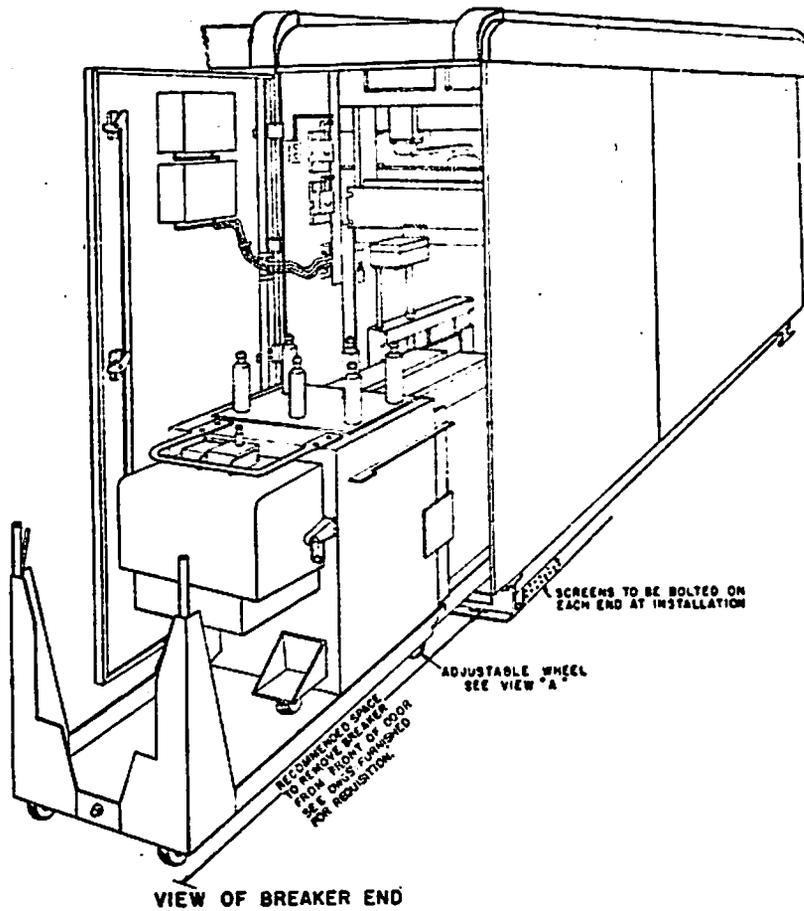
TO CHANGE HEIGHT OF TRUCK FLOOR, LOOSEN NUT "A" THRU OPENING IN TRUCK FLOOR, ADJUST SLOTTED SCREW "B" WITH SCREW DRIVER TO GIVE DESIRED HEIGHT, AND LOCK BY TIGHTENING NUT "A".
