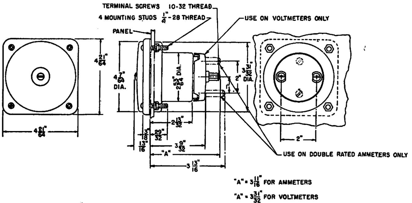
Fig. 4. Dimensions of Type AB-30 ammeters and voltmeters
