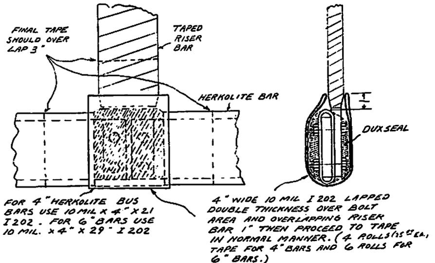
Fig. 26 13.8 KV Taped Joints
