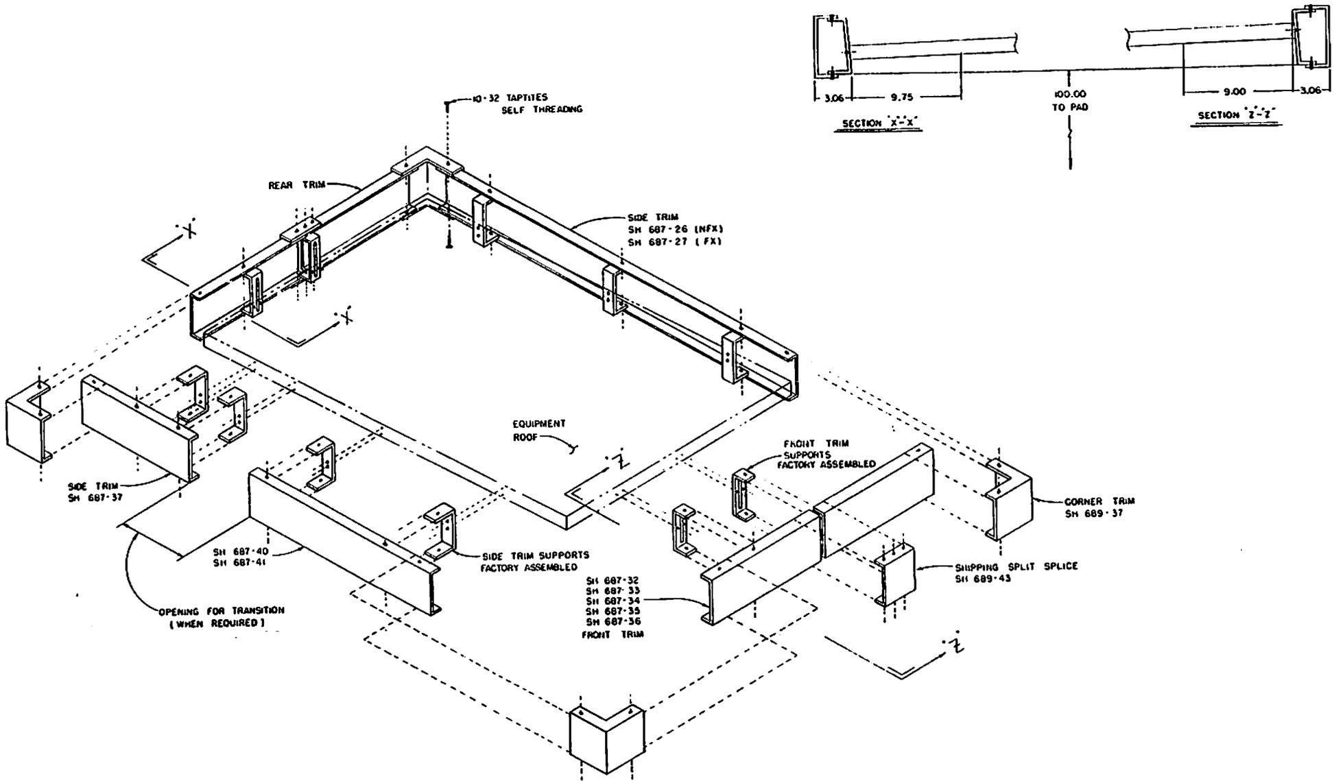
Figure 6. (0673D0515-696) Installation of Appearance Trim
