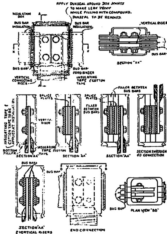
Fig. 25 Method of Making Bus Bar Connections
