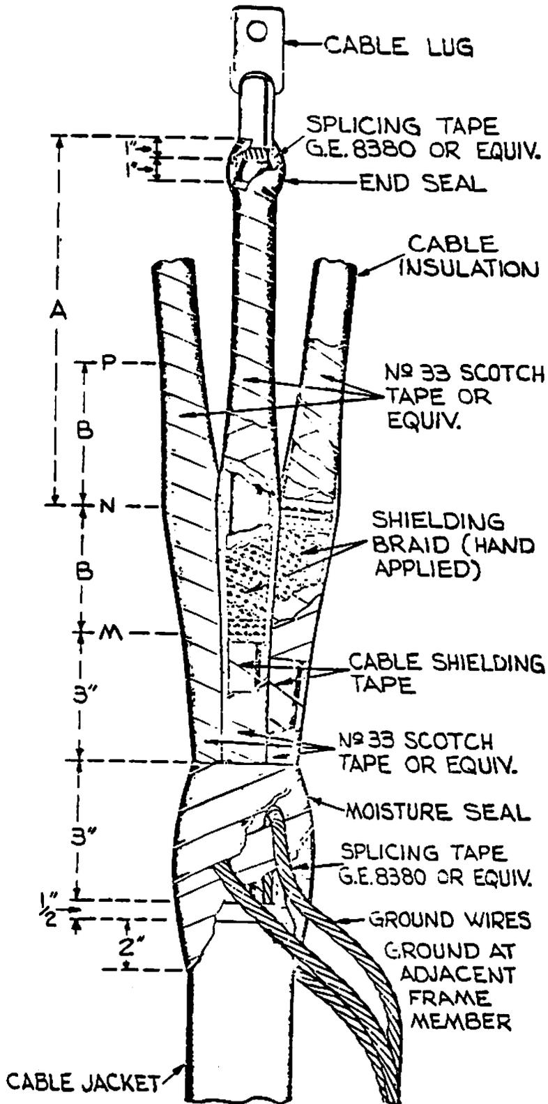
FIG. 29 (B232004C) TERMINATION WITHOUT POTHEAD MULTI-CONDUCTOR
