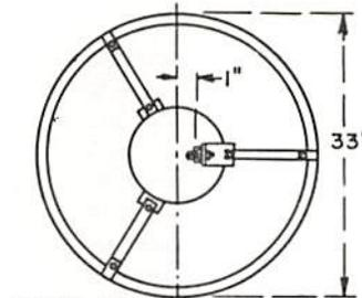
DETAIL OF LINE TERMINAL BRACKET AND GRADING RING FOR ARRESTERS RATED 97, 109 AND 121 KV
