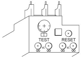
Figure 14. Over Current Relay
