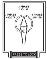
Figure 15. Voltage Selector Switch
