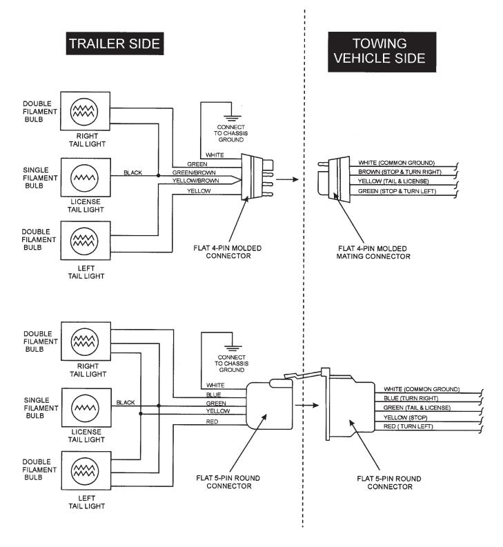
Figure 68. Trailer/Towing Vehicle Wiring Diagram
