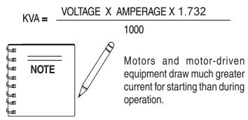
An inadequate size connecting cable which cannot carry the required load can cause a voltage drop which can burn out the appliance or tool and overheat the cable. See Table 5.
