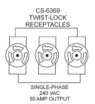
Figure 10. 240 VAC Twist-Lock Auxiliary Receptacles Each auxilliary receptacle is protected by a 50 amp circuit breaker. These breakers are located directly above the GFCI receptacles. Remember the load output (current) on all three receptacles is dependent on the load requirements of the UVWO terminals.
