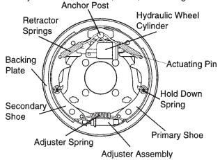
Figure 65. Hydraulic Brake Components
