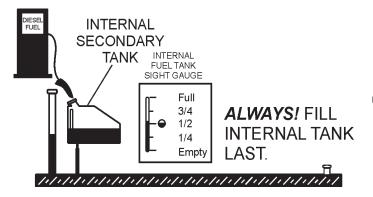
Figure 39. Filling Secondary Internal Fuel Tank
