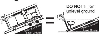
Figure 36. Only Fill on Level Ground
