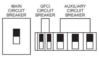
Figure 59. Main, AUX. and GFCI Circuit Breakers (ON)
