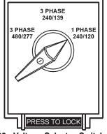
Figure 30. Voltage Selector Switch 240/120V Single-Phase Position
