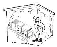
cause serious damage to the generator or engine and may cause injury to people. The generator engine gives off **DEADLY** carbon monoxide gas.
