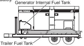
Figure 34. Double Fuel Tank System
