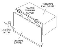
Figure 12. Plastic Face Plate (UVWO Terminals)
