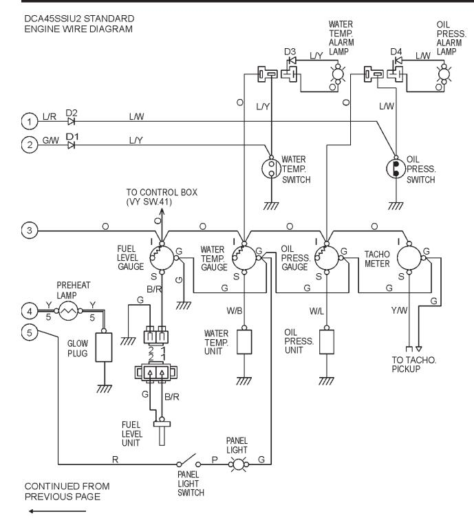
Figure 69. Engine Wiring Diagram(Continued)
