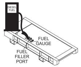
Figure 35. Skid Type Fuel Tank System
