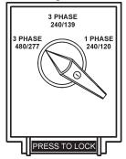
Figure 27. Voltage Selector Switch 480/277V Three-Phase Position
