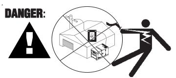
Backfeed to a utility system can cause *electrocution* and or property damage. DO NOT connect to any building's electrical system except through an approved device or after building main switch is opened. ALWAYS have a licensed electrician perform the installation
