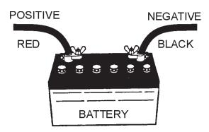
Figure 43. Battery Connections
