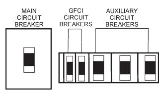
Figure 61. Main, AUX. and GFCI Circuit Breakers (OFF)
