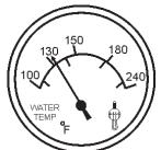
Figure 57. Coolant Temperature Gauge
