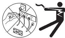
■ NEVER touch output terminals during operation. This is extremely dangerous. ALWAYS stop the machine and place the circuit breaker in the "OFF" position when contact with the output terminals is required. There exists the possibility of *electrocution, electrical shock or burn, which can cause severe bodily harm or even death*!
