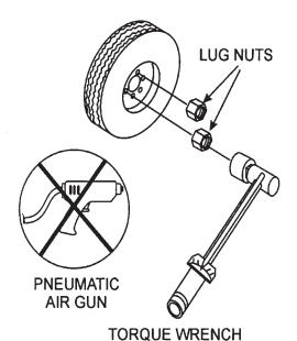
Figure 67. Wheel Lug Nuts Tightening Sequence
