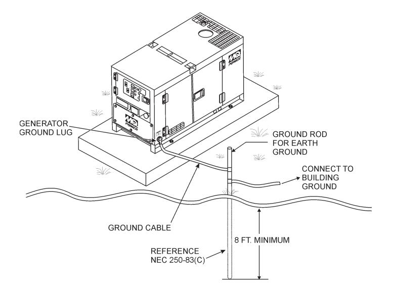
Figure 3. Typical Generator Grounding Application
