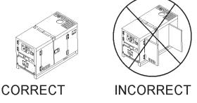
Figure 46. Engine Enclosure Doors
