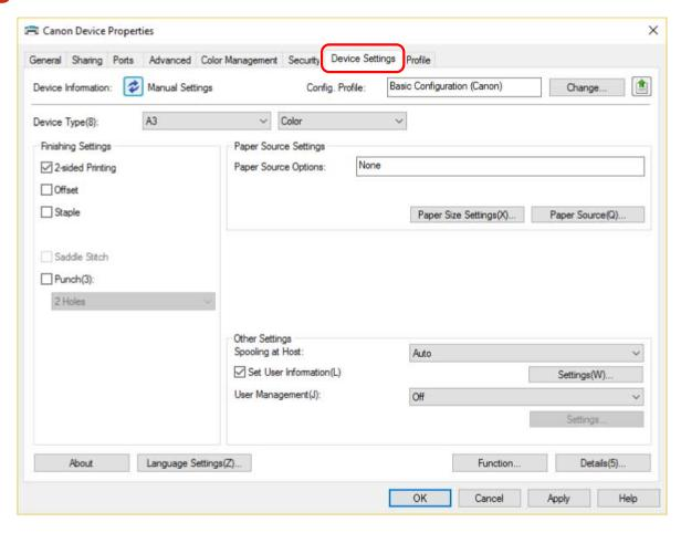
4 Check whether the configuration profile is suitable for the device you are using → if it does not match printer model, click [Change].
