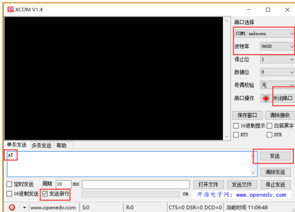
Figure 3: Send AT Command Diagram
