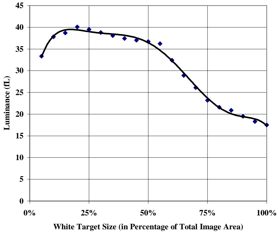
Figure II.2-1. The luminance of white varies inversely with the target size. The IEC luminance requirement is for full screen.
