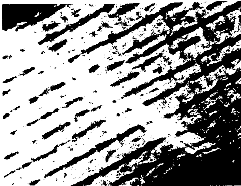
Figure 4: An intense or persistent slip band viewed metallographically and enhanced by polarized light (from Figure 3). Persistent slip bands evolve as initial precipitate shearing by dislocations compromises the order in the \gamma superlattice. This creates preferential avenues for further dislocation penetration through the weakened superlattice. 40X
