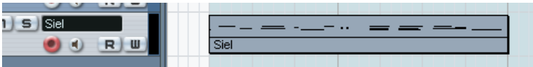
A MIDI part on a MIDI track. The black lines in the part indicate MIDI events.
