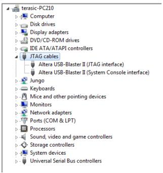
Figure 4-2 USB-Blaster II driver is installed correctly
