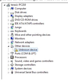
Figure 4-1 Unknown device on device manager
