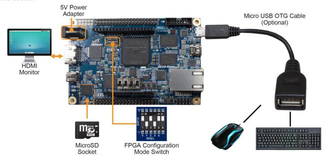
Figure 2-4 Setup for Xfce Desktop
