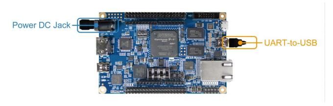
Figure 5-1 Hardware Setup for UART Terminal
