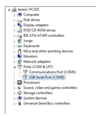
Figure 5-3 USB Serial Poet driver is installed correctly
