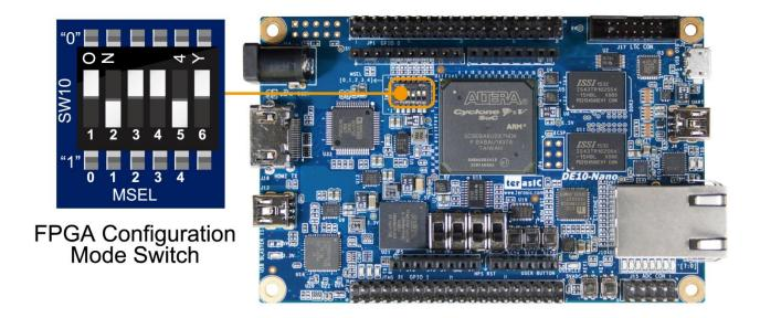
Figure 2-2 FPGA Configuration Mode Switch set in AS Mode
