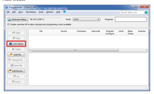
Figure 4-5 Auto detect FPGA device
