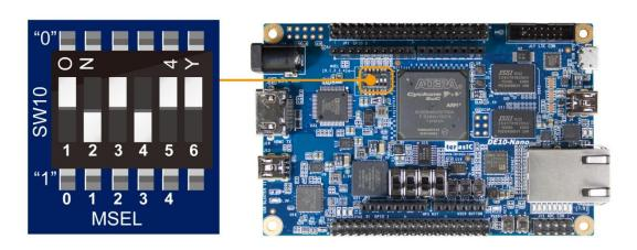
2. Use the Micro USB cable to connect the USB connector on the DE10-Nano board to a USB port on a computer. Once they are connected, plug in the 5-volt power adapter to power up the board.
