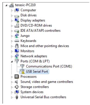
Figure 5-2 Unknown device on device manager
