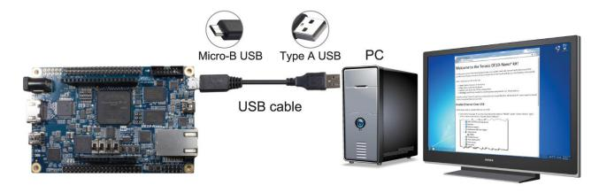
3. After they are connected, the DE10-Nano will display a USB Flash Drive feature in windows. The "**DE10-Nano**" will be shown in the Hard Disk Drives. The drivers and the web server related data will be used in the following steps.
