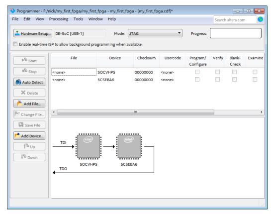
Figure 4-7 JTAG Chain on DE10-nano board
