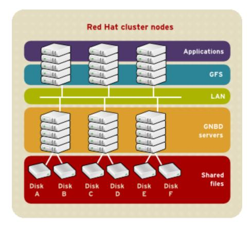
Figure 1.3. GFS and GNBD with Directly Connected Storage
