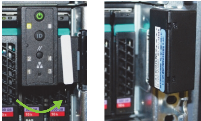
Figure 6 Service tag location on 24-drive Segment server
