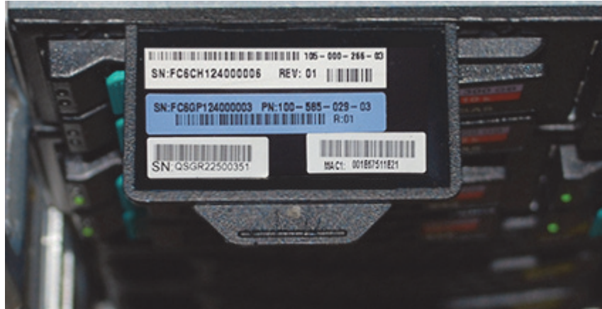
Figure 1 Service tag location on the Master server (Dragon24 shown)
