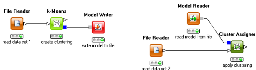
Fig. 7.29 Two KNIME workflows creating a clustering and writing the resulting model to a file ( left ) and reading data and model from file and applying the read clustering model ( right )
