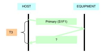
Function 0 is reserved for all Streams to indicated a failed transaction. This secondary reply is sent by the receiver, so the sender does not have to wait for a T3 timeout. In any case, it indicates a failed transaction just like a T3 timeout.
