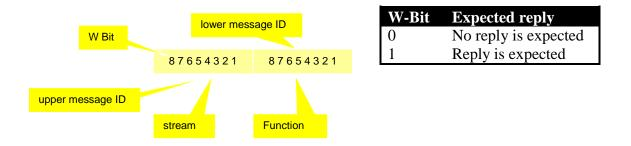
**Block Number** – Bytes 5 and 6 of the header is the block number. The left byte is the upper block number, and the right byte is the lower block number. The left most bit of the left byte is the end bit (E-bit). The E-bit indicates this is the last block of a message.
