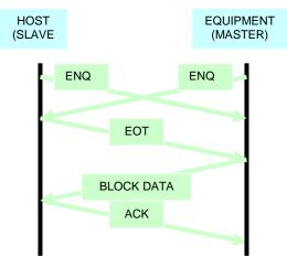
The Block Data is the data portion of either a single-block or multi-block message. It contains a Length Byte, N Data Bytes, and a two byte Checksum.
