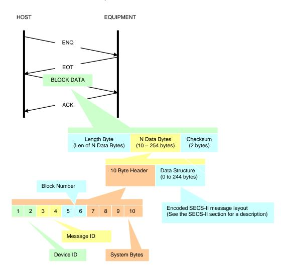
**Length Byte** – Is the first byte sent in the Block Data. It is the number of bytes in the N Date Bytes (10 Byte Header + Data Structure). The two byte Checksum is not included in this count The value ranges from 10 to 254 bytes.
