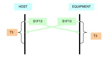
It may be best to allow the equipment to send the S1F13 first. Then the host can send a S1F13 after replying to the equipment's S1F13. Getting the equipment to send the S1F13 may take some experimenting with the equipment. Sometimes taking the equipment in and out of remote mode, or taking the equipment off-line then on-line, causes the equipment to send a S1F13.
