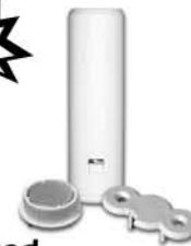
Wireless Recessed Door Contacts 56A00-1 This recessed supervised wireless transmitter is used for the protection of doors and windows in installations where the contact must be totally hidden. The transmitter is concealed within the door or window frame for virtual transparency. It is supplied with a replaceable lithium battery that lasts for 5 years under normal conditions.
