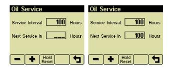
Button 1 decreases the service interval time while Button 2 increases the service interval time in 10 hour increments. Holding
