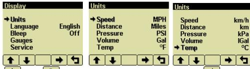
Use Buttons 1 and 2 to select the unit to change. Press Button 4 to change the selected value. Press Button 5 to return to Display menu.
