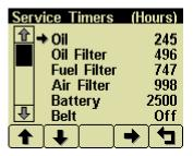
Pressing Button 4 allows adjusting the selected service timer.
