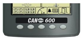
Five buttons access a context dependent **button bar** when any button from 1 to 4 is pressed. The graphical menu structure uses easily understood icons to indicate the button's current function. After 5 seconds of inactivity the button bar disappears.
