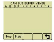
Button 1 Stop freezes the display while button 2 State shows CANbus data statistics screen.
