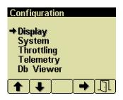
The top level configuration menu is displayed as shown. Buttons 1 and 2 allow you to choose from **Display**, **System**, **Throttling**, **Telemetry** or **Db Viewer**. Pressing button 4 selects the chosen menu item indicated in bold and the arrow. Each item is described in detail on the following pages. Settings are automatically stored when exiting the current menu even when power is removed.
