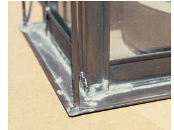
Other maker's seams after weathering
