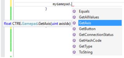
GetAxis() and GetButton() can be used to retrieve axis and button information. GetConnectionStatus() can be used to determine if a gamepad is present.
