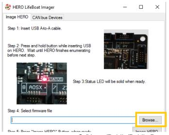
Next press the "**Browse**" button to navigate to the firmware file. Because the file path is blank, LifeBoat will start the dialog box inside the install location of LifeBoat, which is ideal since that is where the firmware files are located.
