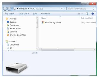
The first time you connect the USB-A-to-A cable, you will see a mass storage device for HERO Files. This is due to the ship-firmware in the HERO, and will function on any Window PC (even if HERO SDK is not installed).
