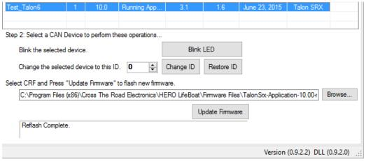
If power or communications is disrupted during the field-upgrade, LifeBoat will report the error and the CAN device will be left in bootloader mode (which is harmless). At which point you can simply try again after resolving the intermittent power/communication issue. In other words, the CAN devices are not susceptible to "bricking" due to incomplete flashes.
