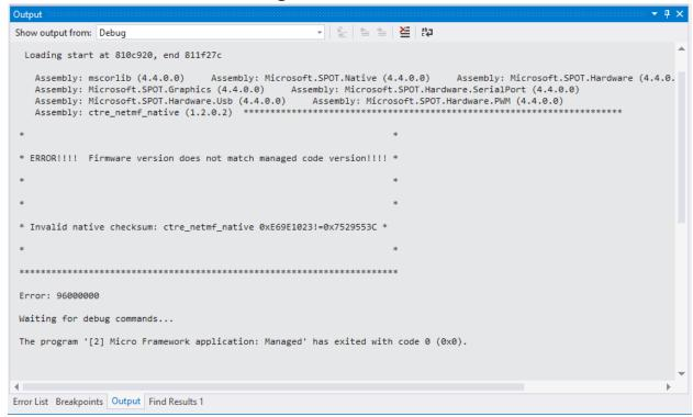
This can happen when there is a mismatch between the HERO's firmware and the HERO SDK installed on your PC. The simplest solution is to use HERO LifeBoat to re-image the HERO so that the firmware and SDK is synchronized again. See <u>Section 7.1</u> for instructions on reimaging the HERO.
