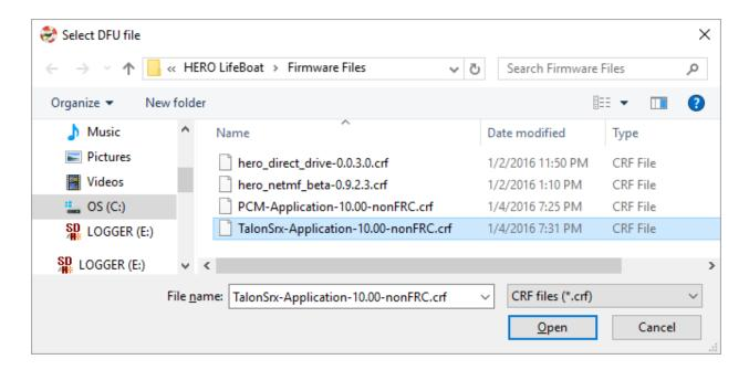
Next press "Update Firmware" to begin flashing the CAN device.
