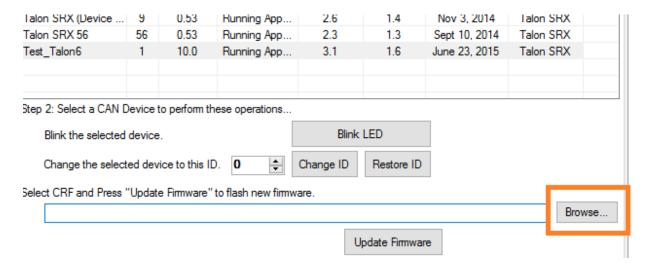
For example, if re-flashing a Talon SRX, choose the Talon SRX crf file. Then press "Open".
