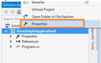
Select the **Micro Framework** Tab, select **USB as the Transport**, and (re)select the HERO as the device. It should appear as "**Cross Link HERO**.**NETMF\_Mini-USB**". **Always** click on the dropdown's down-arrow to repopulate the list of attached hardware, otherwise the selection may not take effect.
