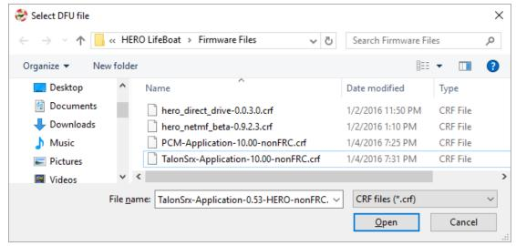
If the NETMF firmware is required (for developing robot applications in Visual Studio) select the latest "hero\_netmf\_XXXXXX.crf".
