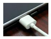
Plug the other end of the mini USB cable into PC Host port.
