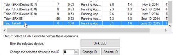
Then enter the new device ID into the number entry. If need be, the "Restore ID" button can be used to modify the number entry back to the device's current value. Beyond this, "Restore ID" has no effect on the actual CAN devices.
