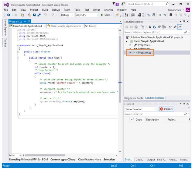
The next step is to debug/deploy this example to the HERO. To do these we will select the HERO as the target device (next section).
