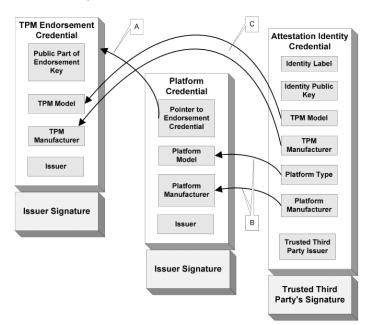
In this context the Endorsement Credential and the Attestation Credential have private keys within the TPM that can be used to validate their corresponding credentials. The Platform Credential links to the Endorsement key/Credential via a set of attributes within the credential. The Platform Credential cannot be considered valid unless the Endorsement Credential has been validated since it is linked to the Endorsement Credential and has no private key of its own.
