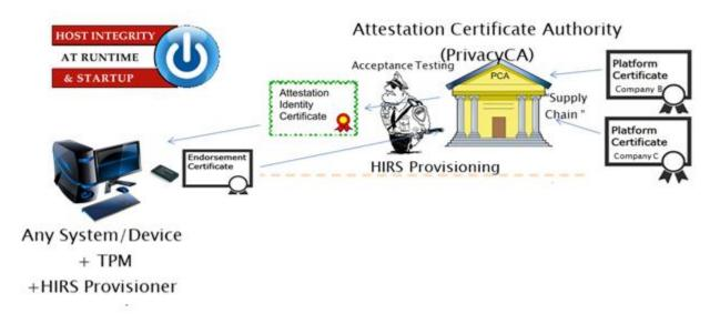
The Attestation CA is a core component of the TPM PKI architecture. Its role is certifying Attestation Identity Keys (AIK), used by TPMs to sign quotes. It issues an Attestation Identity Certificate (AIC) to the HIRS provisioner as part of the client provisioning process.
