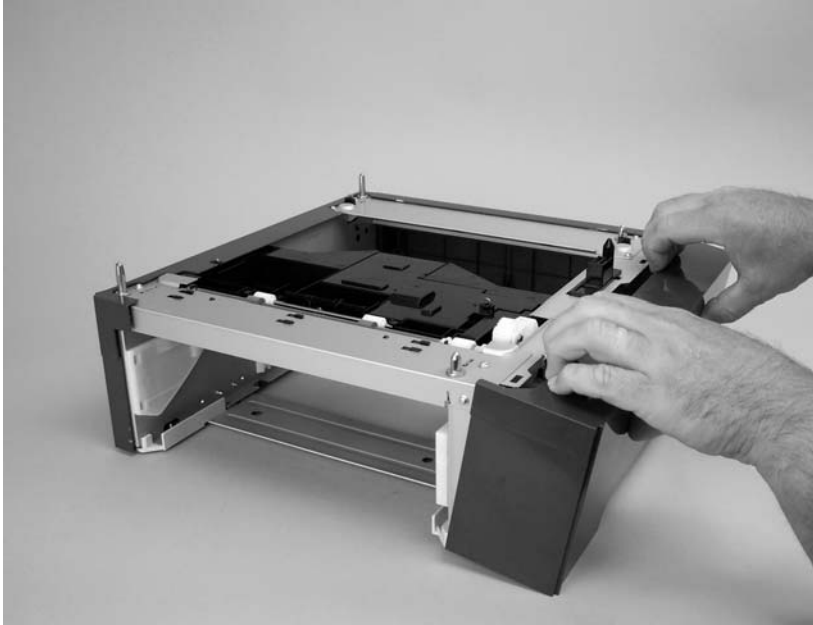
Figure 5-112 Remove the 500-sheet feeder right cover (2 of 3)
