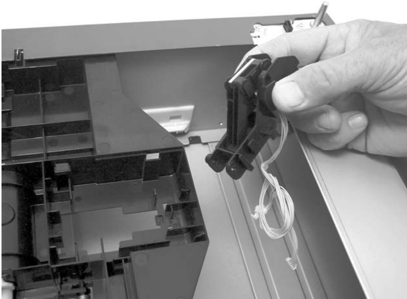
Figure 5-127 Remove the media sensor (500-sheet feeder) (4 of 4)
