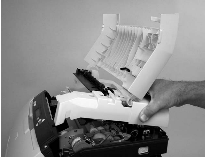
Figure 5-15 Remove the upper cover (5 of 5)
