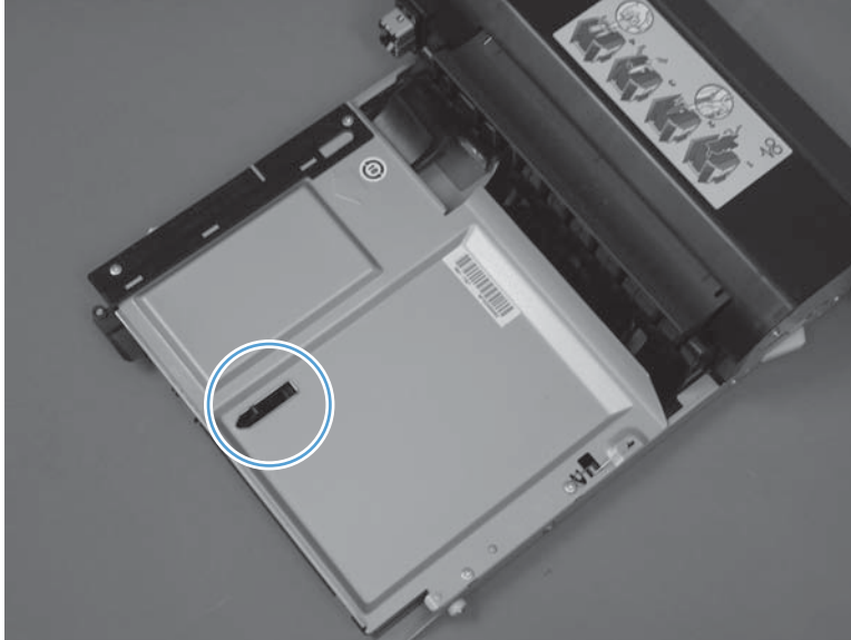
Figure 3-7 Test the fuser duplex sensor
