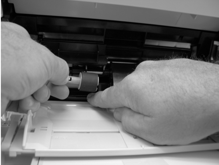
Figure 2-31 Remove the Tray 1 separation roller (3 of 3)
