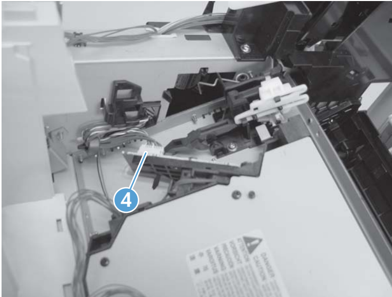
Figure 2-131 Remove the laser/scanner assembly (4 of 4)
