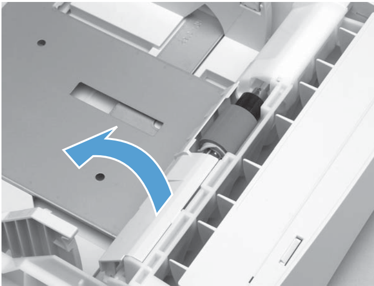
Figure 2-5 Remove the Tray 2 separation, pickup, and feed rollers (1 of 4)
