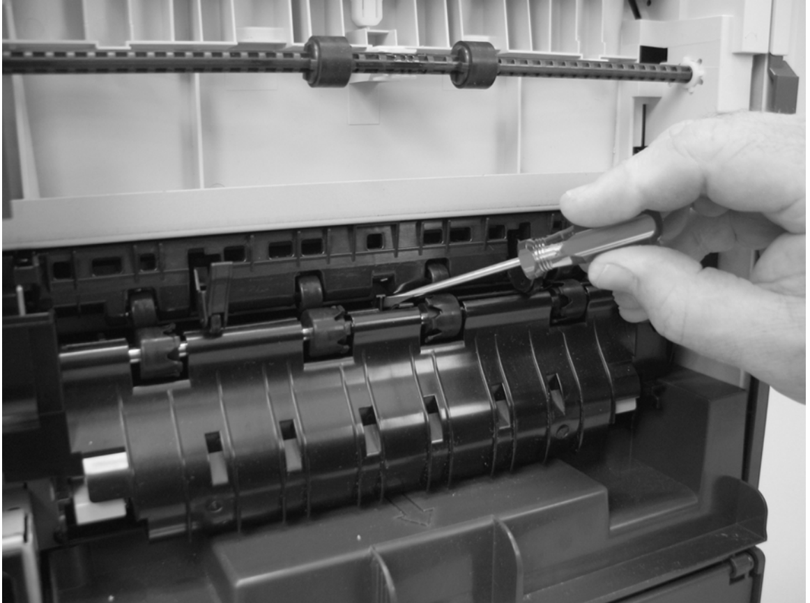
Figure 3-6 Test the fuser delivery sensor (PS700)
