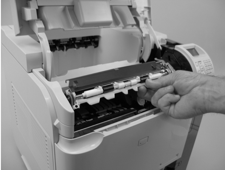
Figure 2-62 Remove the registration assembly (3 of 4)
