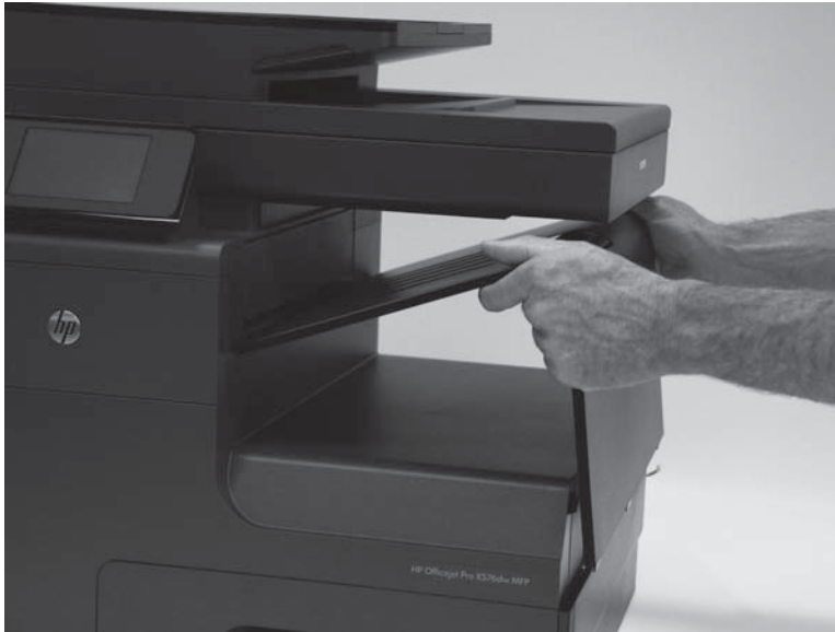
Figure 1-16 Remove the output bin
