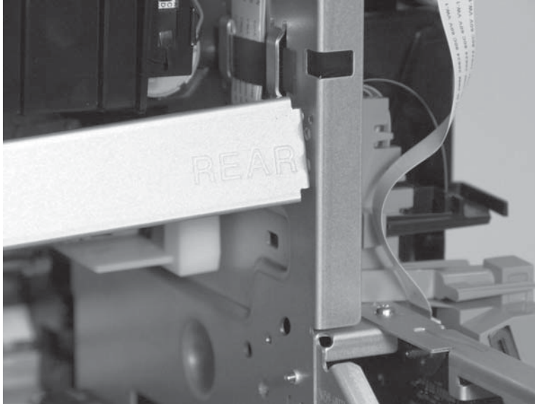
Figure 1-103 Remove the right cross brace (4 of 4)
