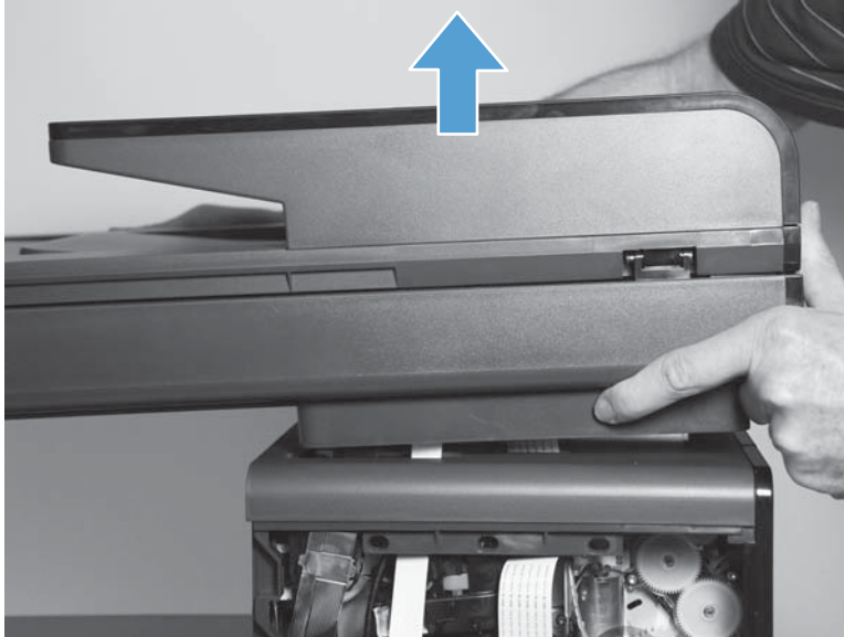
Figure 1-84 Remove the scanner and scanner support bracket (8 of 9)
