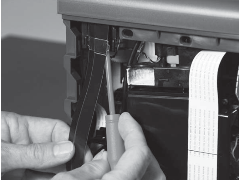
Figure 1-80 Remove the scanner and scanner support bracket (4 of 9)
