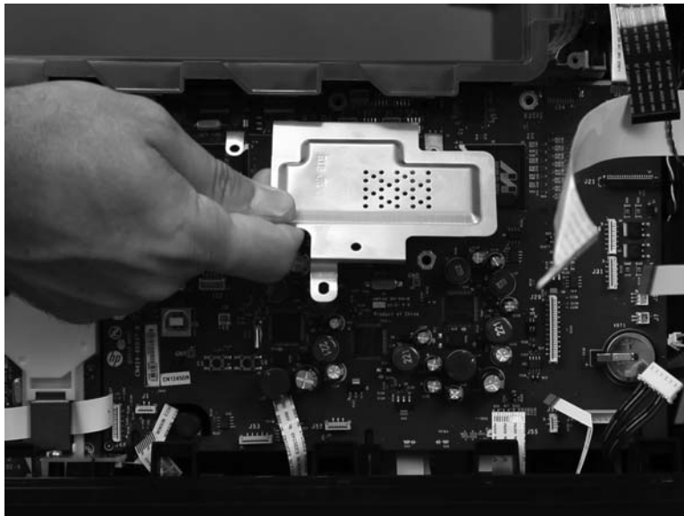
Figure 1-206 Remove the main PCA (6 of 8)
