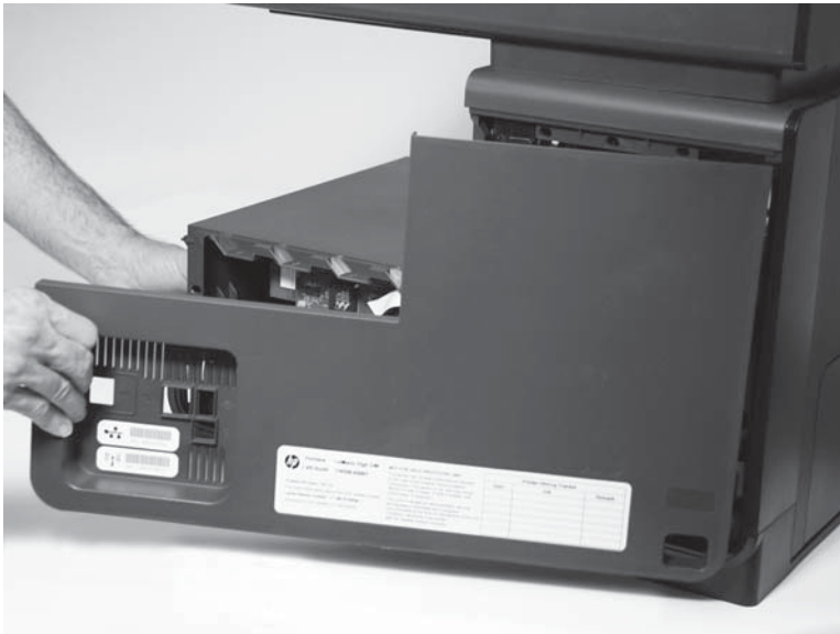
Figure 1-24 Remove the rear cover (2 of 2)
