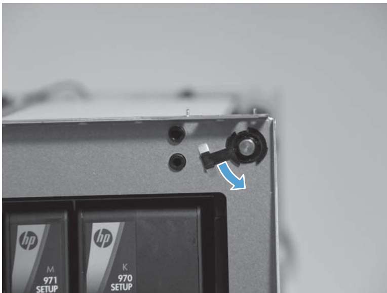
Figure 1-138 Remove the output drive shaft 6 (2 of 3)
