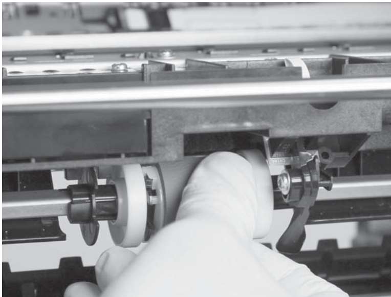
Figure 1-68 Reinstall the separator/pick assembly (4 of 5)
