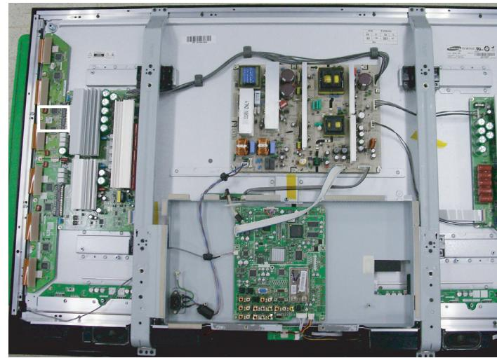
Set the main reset (rising : 60usec, falling : 80usec) by change the value of variable resistor.
