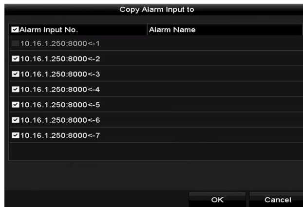
Figure 5-20 Copy Alarm Input
