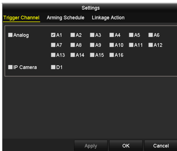
Figure 5-22 Set Trigger Camera of VCA Alarm
